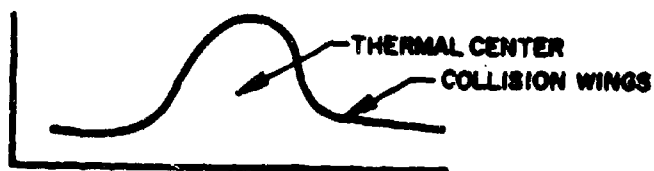
FIG. 3-4 REPRESENTATIVE LINE PROFILE SHOWING THERMAL CENTER AND COLLISION WINGS
