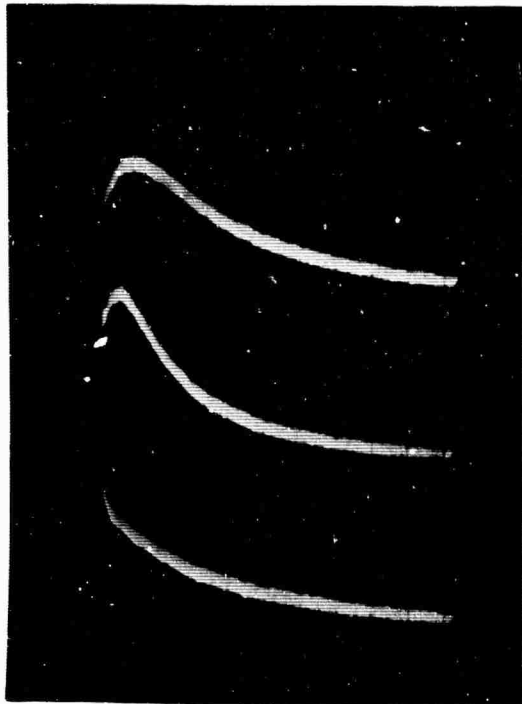
Fig. 18 Pulse Emission Profiles Generated when a C. W. Signal is Passed Through a Pulse Excited Amplifier. (Time scale: 1 division = 200 \mu\text{sec} )
