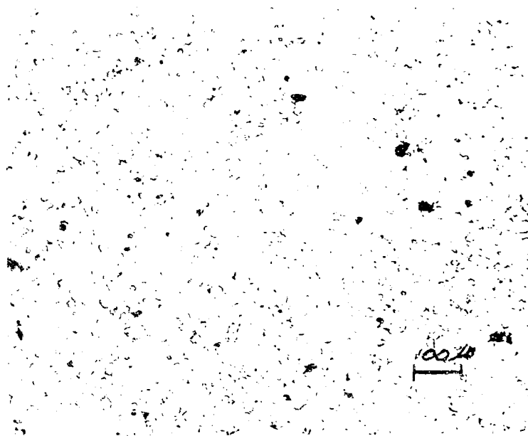
4144T-1 100 X Figure 3.28 Microstructure of Equiaxed Al 2 O 3 + 1/4% MgO after 80 Hour Anneal at 1800°C. Note the lack of appreciable grain growth during this annealing.
