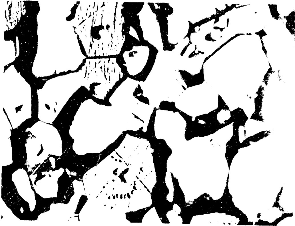
Figure 3.12 Polycrystalline matrix of billet FA-14 near strain-anneal single crystal after etching in K_2S_2O_7 at 700^\circ C for 30 seconds.
