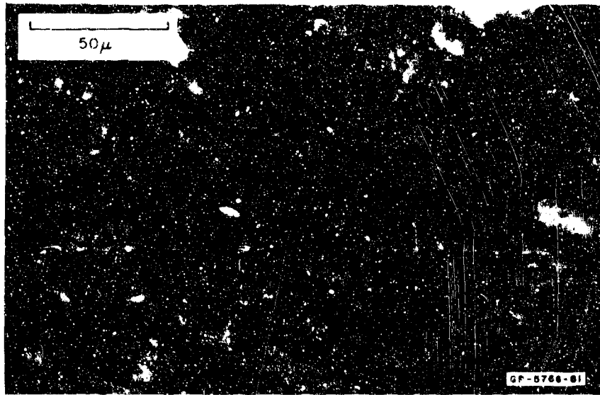
FIG. 56 PHOTOMICROGRAPH OF CERAMIC (AD94) SHOWING FRACTURE
