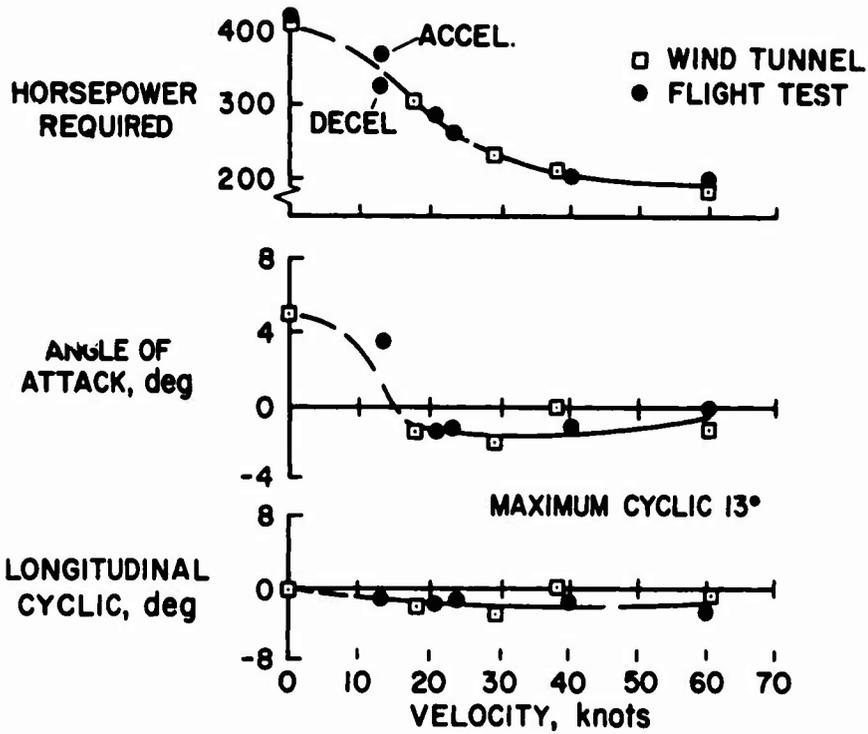
Fig. 6 Balanced, level flight characteristics of the XV-3 convertiplane
