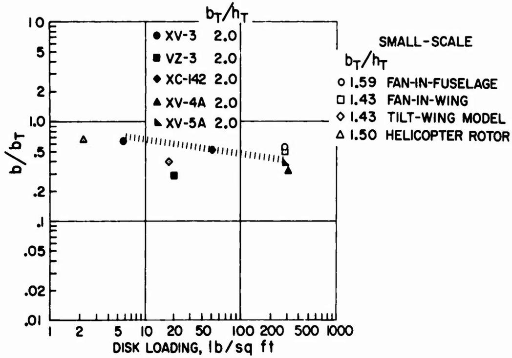
Fig. 18 Aircraft and model span (wind-tunnel width) ratios
