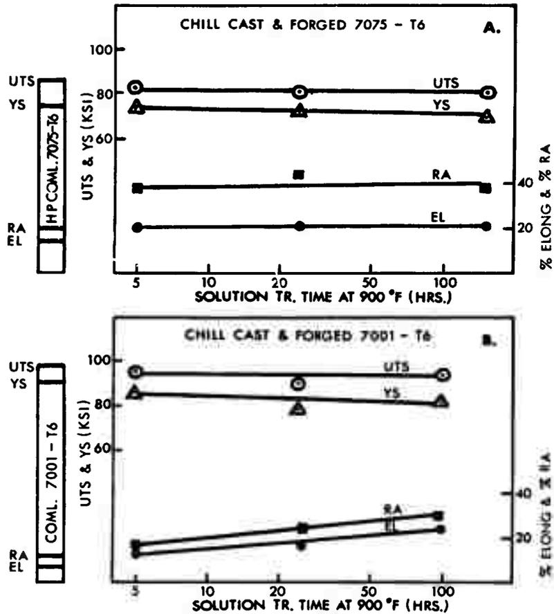
Bar-graphs at left: are tensile properties of commercial alloys, solution treated for 5 hours at 900 F and aged 24 hours at 250 F
