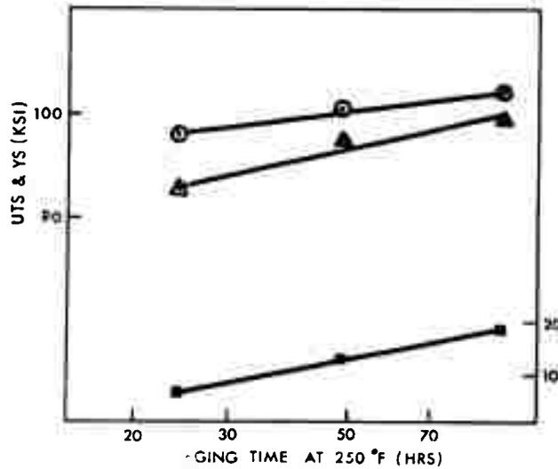
Figure 13. Effect of Aging at 250° F on Hardness and Tensile Properties of a Weld-cast and Hot rolled 7001 Alloy
