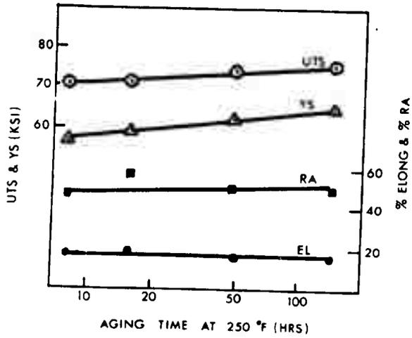
Figure 15. Effect of Aging at 250° F on Hardness and Tensile Properties of a "Leaner Solute" Alloy
