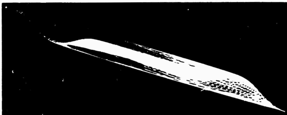
Fig. 10 - Photographic time exposure of boom tip motion after initial displacement in 90-deg direction
