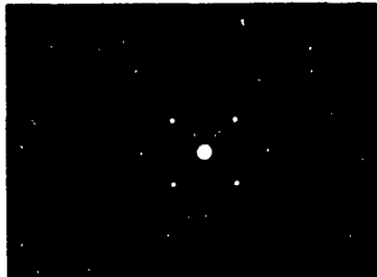
PLATE 9. Diffraction pattern of single crystal chromium film deposited on vacuum cleaved NaCl at 10^{-9} torr (100) orientation
