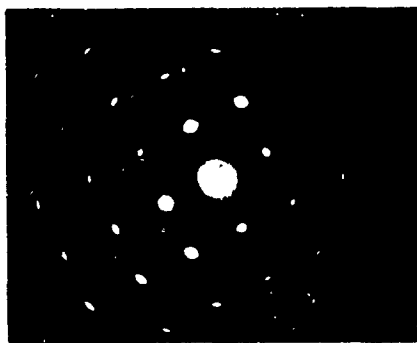
PLATE 8. Diffraction pattern of chromium deposited on air cleaved NaCl that had been heated to 480^{\circ}\text{C} and then cooled to deposition temperature at 10^{-6} torr.
