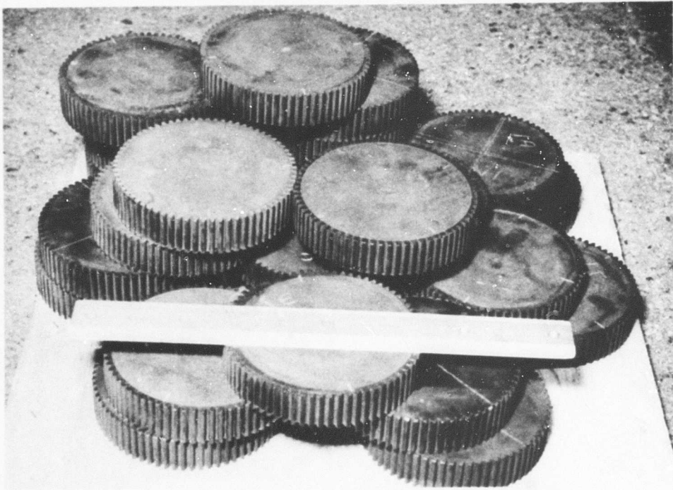
Figure 8. As-Forged 5-Inch Gears with Integral Teeth with Flash Removed.
