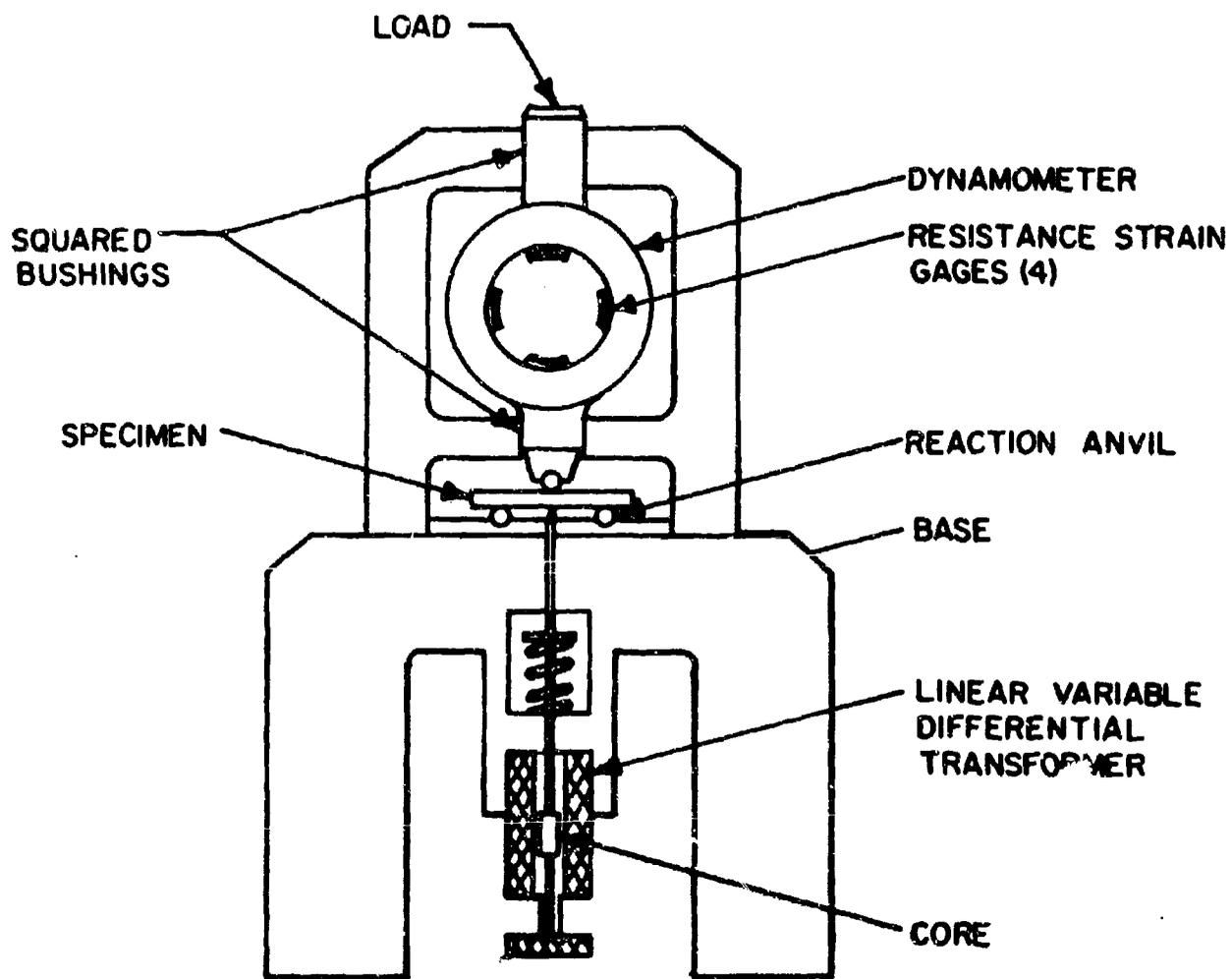
Figure 6. Schematic Diagram of Apparatus for Measuring Elastic Modulus.
