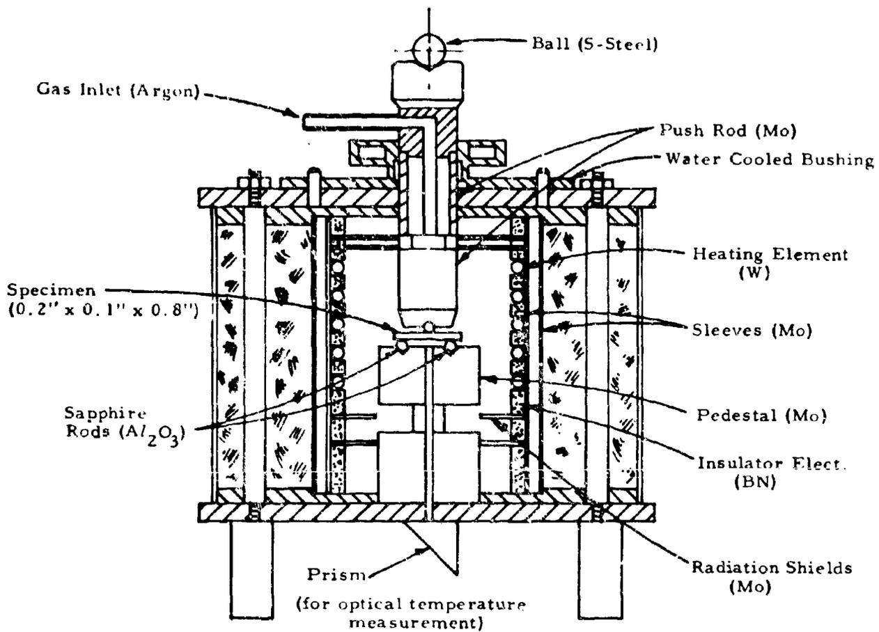
Figure 5. Schematic Diagram of Elevated Temperature Bend Test Apparatus.
