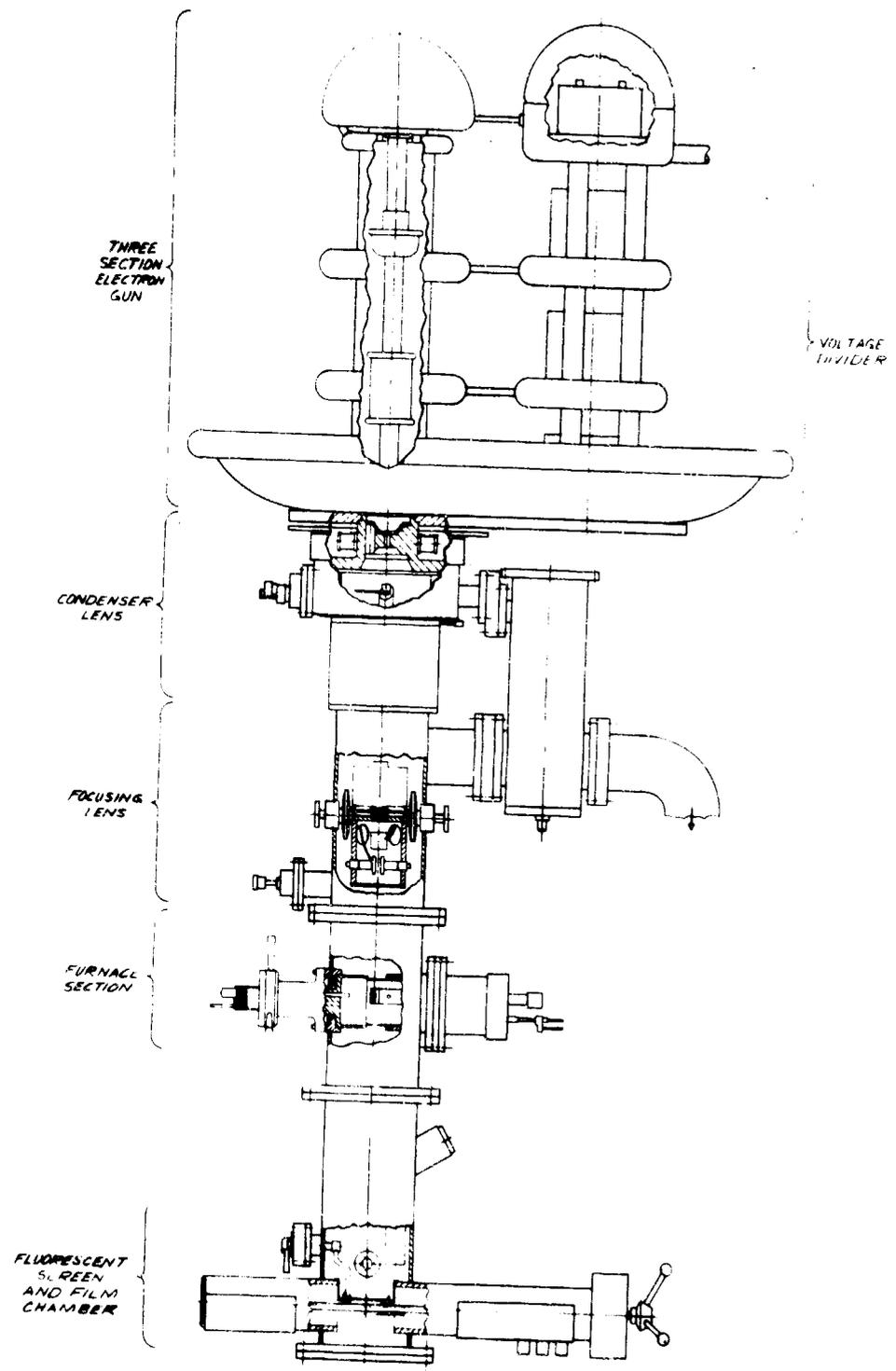
ELECTRON DIFFRACTION APPARATUS
