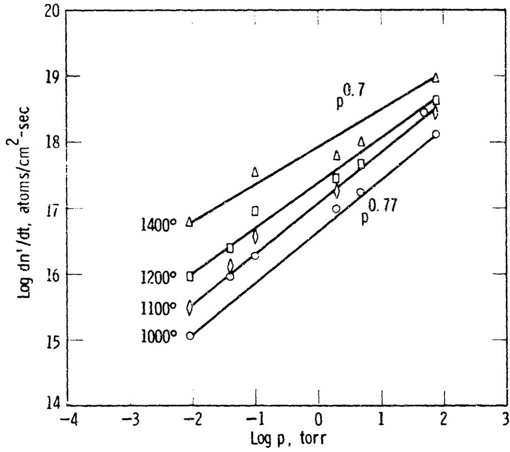
Fig. 10—Log rate vs log pressure, oxidation of molybdenum
