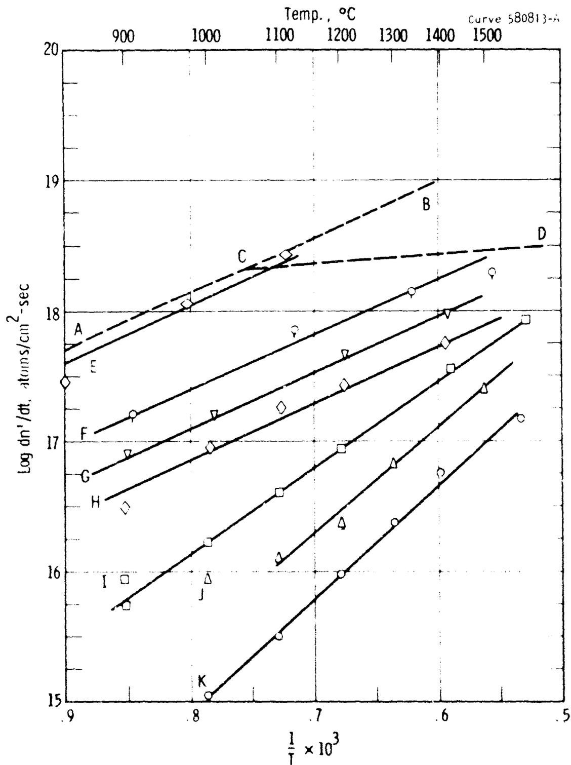
Fig. 9—Log  $dn'/dt$  vs  $1/T$ , oxidation of molybdenum AB chemical control
