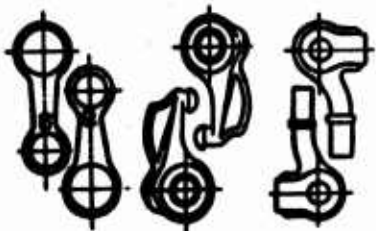
Fig. 33. Examples of doubled location of forgings for stamping.
