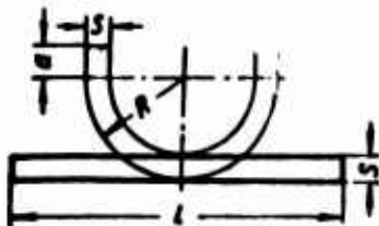
Fig. 75. Diagram of bending of the half-shell from thick-leaved steels.
