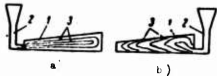
Fig. 16. Change of character of hardening of a casting depending on the place of feed of the metal; a) simultaneous hardening; b) sequential hardening; 1 - casting; 2 - flow gate; 3 - layers of consecutive hardening of the casting.
