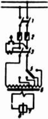
Fig. 38. Electrical diagram of machine for contact welding: 1 - knife switch; 2 - safety fuse; 3 - magnetic contactor; 4 - starting push button; 5 - sectional switch; 6 - welding transformer; 7 - electrodes; 8 - welded parts.
