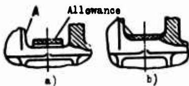
Fig. 55. Construction of poured cavities: a) untechnologic construction; b) technologic construction.
