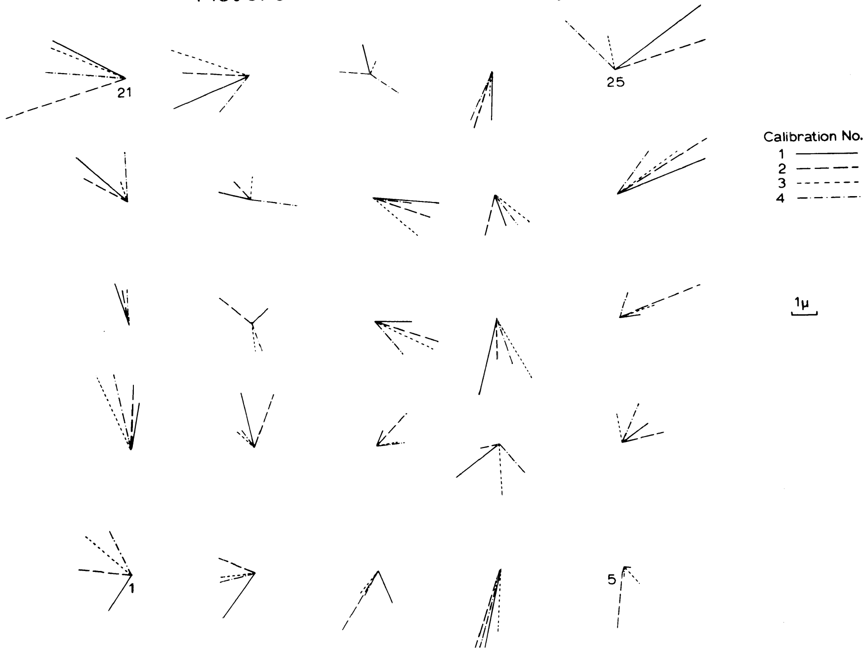
Fig. 7 Coordinate Differences Obtained from Four Grid Calibrations
