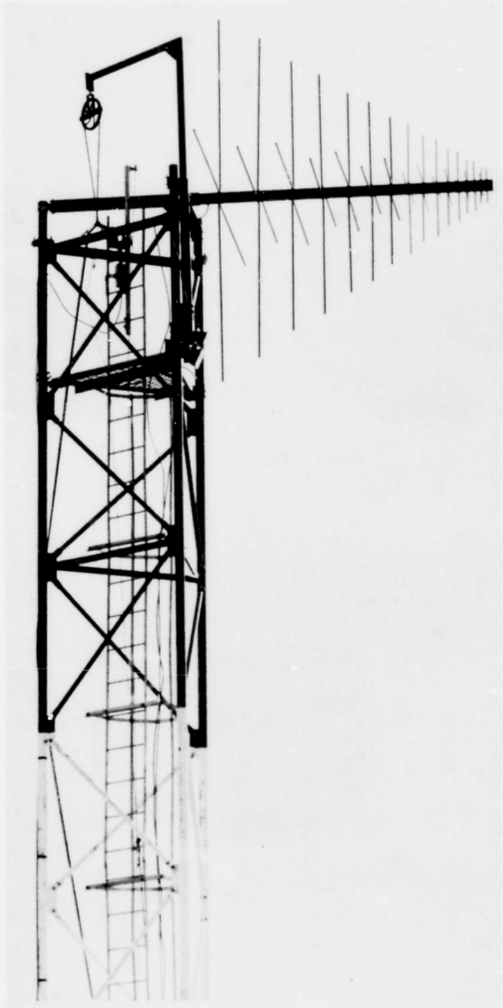
Figure 32. Circularly Polarized Log-Periodic Dipole Antenna Employing Square-Boom Construction
