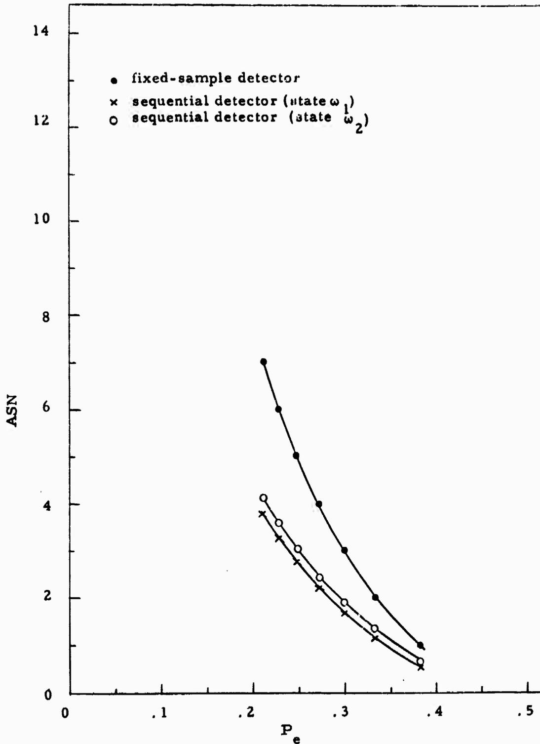
Figure 57. Calculated ASN for the two-known-signals case versus error probability for the fixed-sample detector ( $p(\omega_1) = p(\omega_2) = 1/2$ ) and the sequential detector for both states of nature  $\omega_1$  and  $\omega_2$  where  $\bar{y}_1 = 12$  and  $\bar{y}_2 = 10$ .
