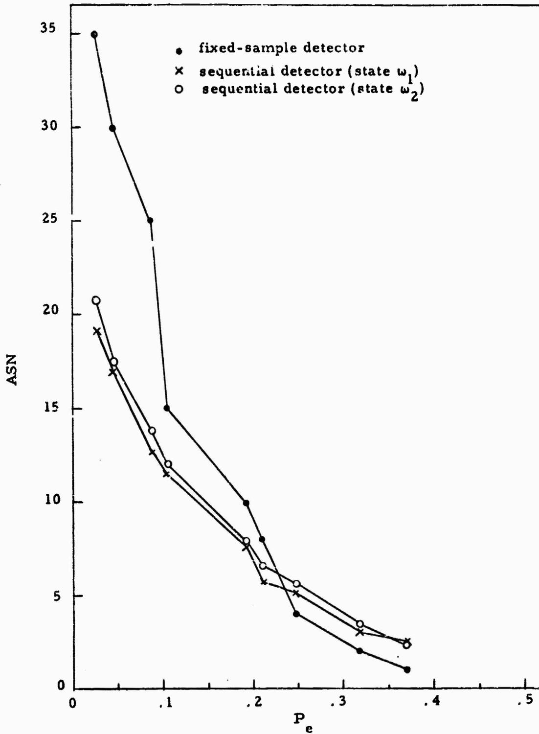
Figure 58. Computer-simulated ASN for the two-known-signals case versus error probability for the fixed-sample detector ( $p(\omega_1) = p(\omega_2) = 1/2$ ) and the sequential detector for both states of nature  $\omega_1$  and  $\omega_2$  where  $\bar{y}_1 = 12$  and  $\bar{y}_2 = 10$ .
