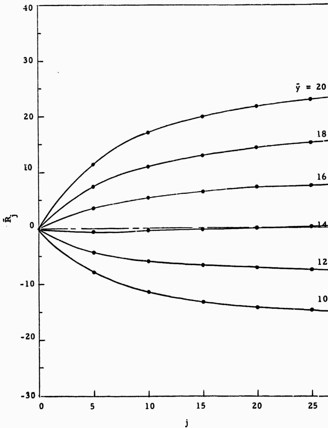
Figure 56. Computer-simulated mean cumulative information versus sample number for a sequential detector designed for two unknown signals and for various values  $\bar{y}$  of actual signal present where  $\bar{y}_1 = 20$ ,  $\bar{y}_2 = 10$ , and  $u = 100$ .
