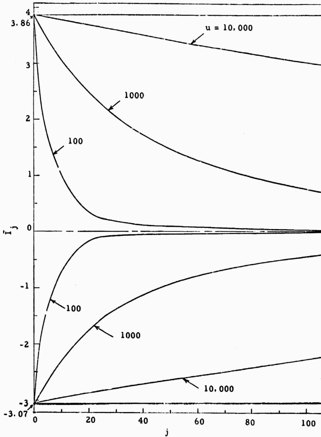
Figure 50. Calculated mean information per sample versus sample number for a sequential detector designed for the two-known-signals case and the two-unknown-signals case where  $\bar{y}_1 = 20$ , and  $\bar{y}_2 = 10$ .
