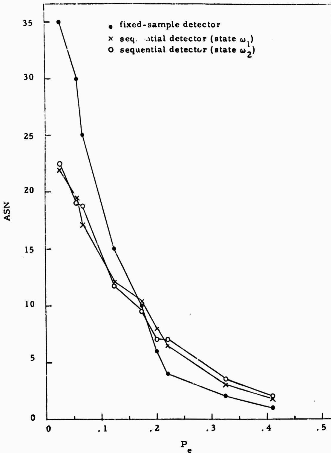
Figure 59. Computer-simulated ASN for the two-unknown-signals case versus error probability for the fixed-sample detector ( $p(\omega_1) = p(\omega_2) = 1/2$ ) and the sequential detector for both states of nature  $\omega_1$  and  $\omega_2$  where  $\bar{y}_1 = 12$ ,  $\bar{y}_2 = 10$ , and  $u = 1000$ .
