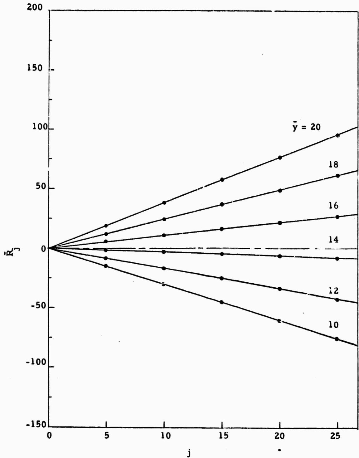
Figure 55. Computer-simulated mean cumulative information versus sample number for a sequential detector designed for two known signals,  $\bar{y}_1 = 20$  and  $\bar{y}_2 = 10$ , and for various values  $\bar{y}$  of actual signal present.
