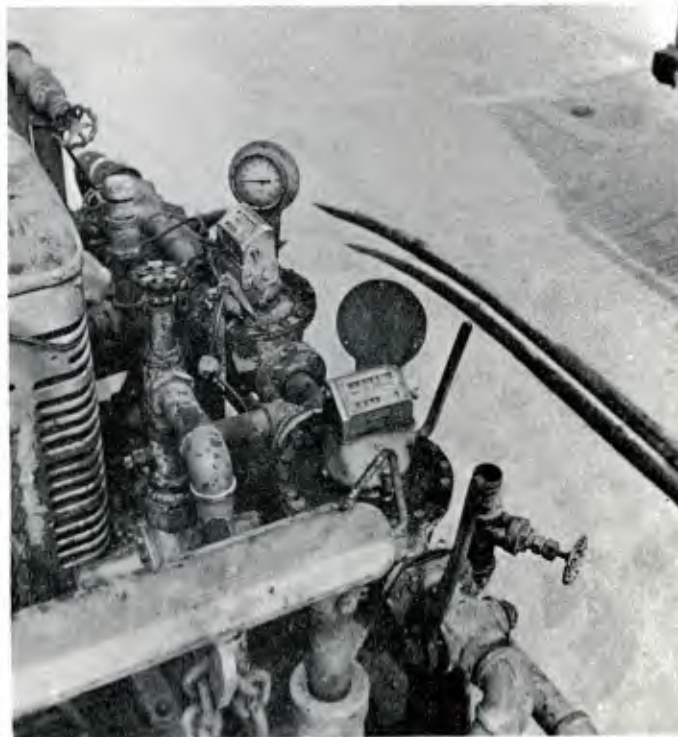
Figure 13. Close-up of chemical pumps, meters, and control valves.
