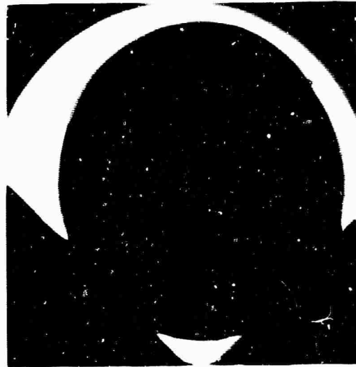
Figure 10. No. 2500-10-5 - Schlieren photograph showing the effect of horizontal and vertical movement of the boule on core shape and size.
