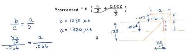
For the 10 inch beam of 0.128 inch thickness and a deflection of 1 inch the corrected strain was:
