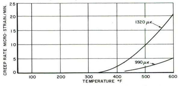
The characteristic drift at temperature was a notable part of creep data at temperatures over 500°F. The drift function added to or subtracted from the creep data depending upon whether the test beam was loaded in compression or tension.
