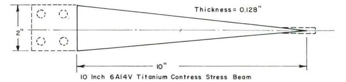
A stepping block with deflection steps of .250" was used to deflect the beam. The top step caused a total beam deflection of one inch.
