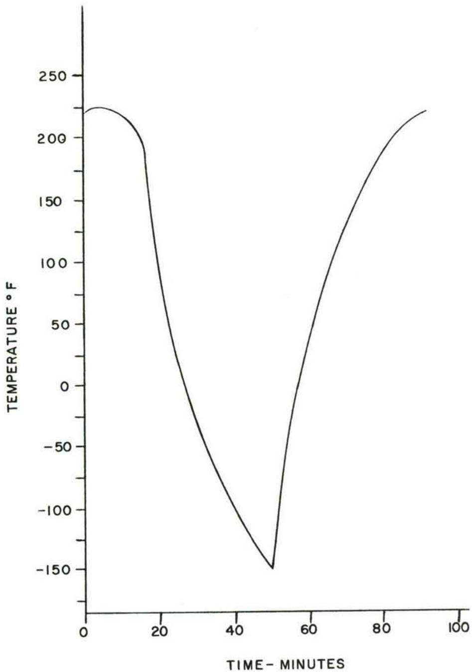
Figure 7. Time-Temperature Profile Adapted to Solar Collector Tests
