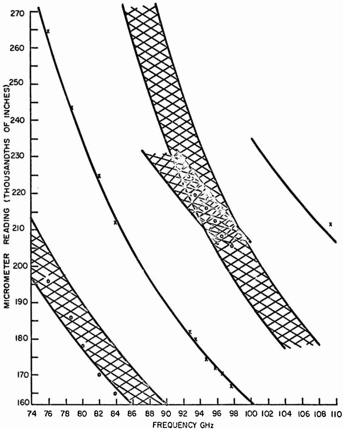
FIG.17-CALIBRATION CURVE FOR TUNABLE FILTER (X,O MEASURED POINTS)
