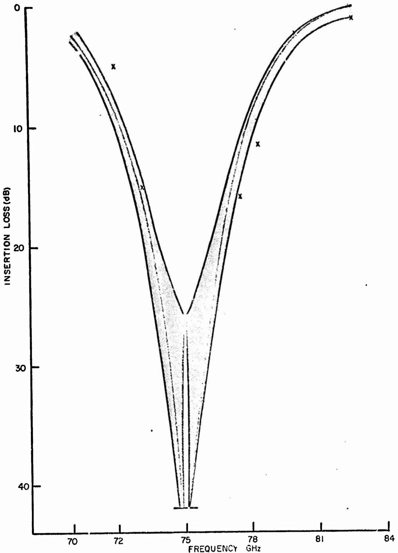
FIG.14-CALCULATED INSERTION LOSS OF A HYBRID JUNCTION FILTER.
