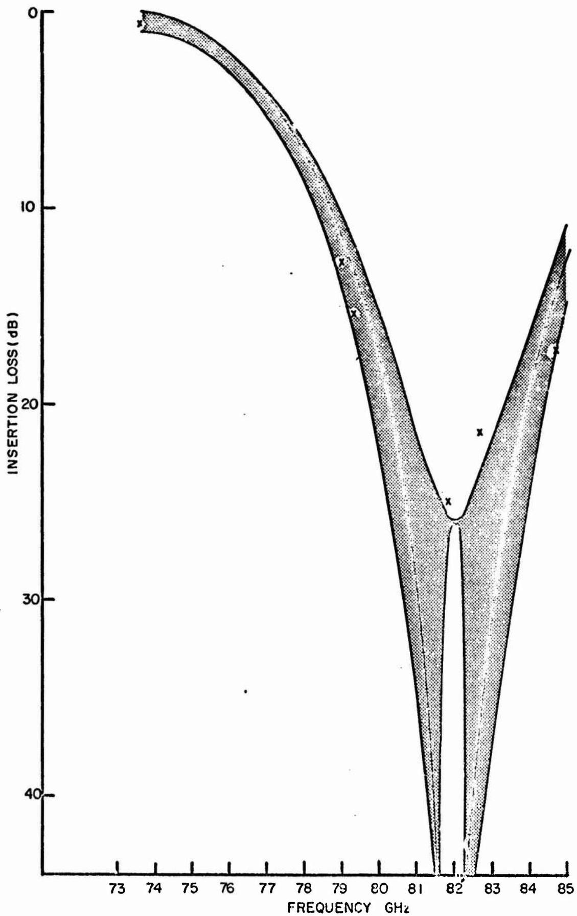
FIG.13-CALCULATED INSERTION LOSS OF A HYBRID JUNCTION FILTER
