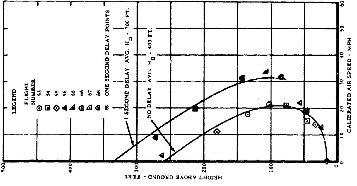
FIG. 5 HEIGHT VELOCITY DIAGRAMS - BASIC DATA. HELICOPTER GROSS WEIGHT, 10,100 POUNDS. THREE DENSITY ALTITUDES SHOWN.
