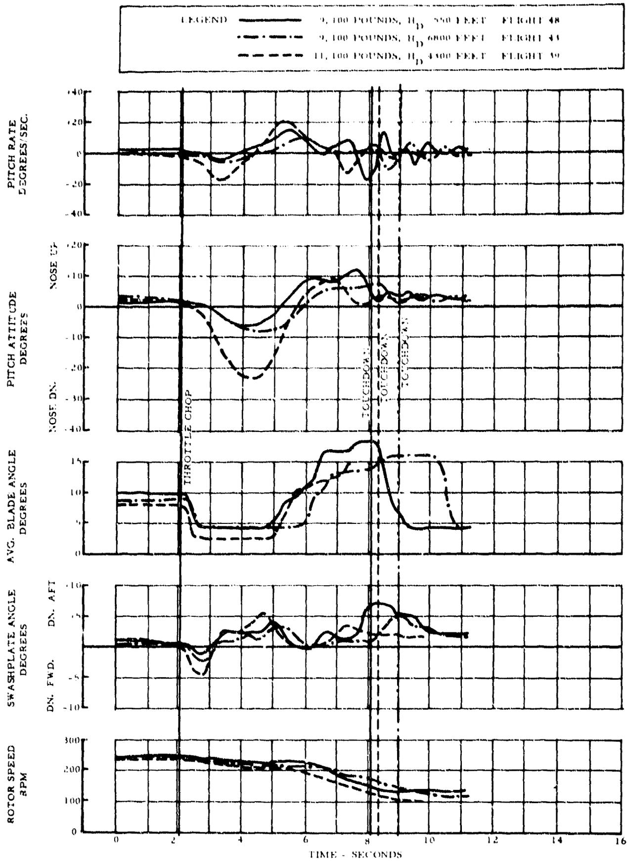
FIG. 11 COMPARISON OF TIME HISTORY DATA FOR CRITICAL SPEED AREA ( $V_{cr}$ ,  $h_{cr}$ )
