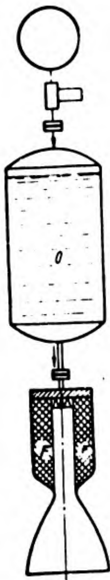
Fig.28 - Schematic Diagram of Bipropellant Rocket Engine with Solid Fuel Housed in Chamber
