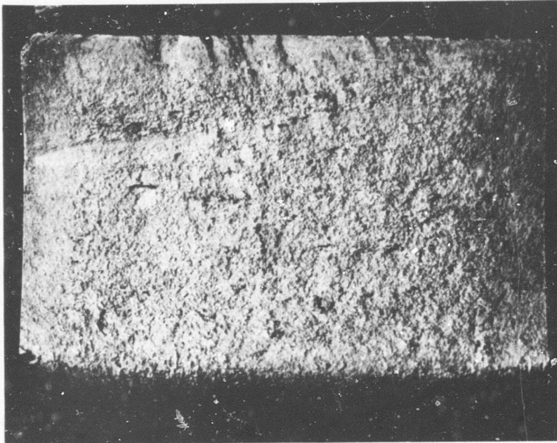
Magnification: 9X EX-78782, Serial Number CX 9113 Figure 69. Photomicrograph of Surface of Failure of Tooth 1 of Test Gear Showing Multiple Origins of Failure in Root of Loaded Involute – No Typical Arrest Lines of Fatigue Progression.
