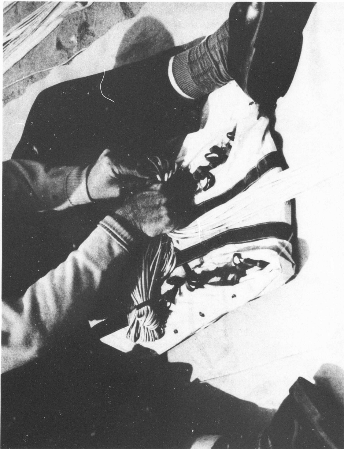
Figure 10. Line Bundle Stowage on Deployment Sleeve.
