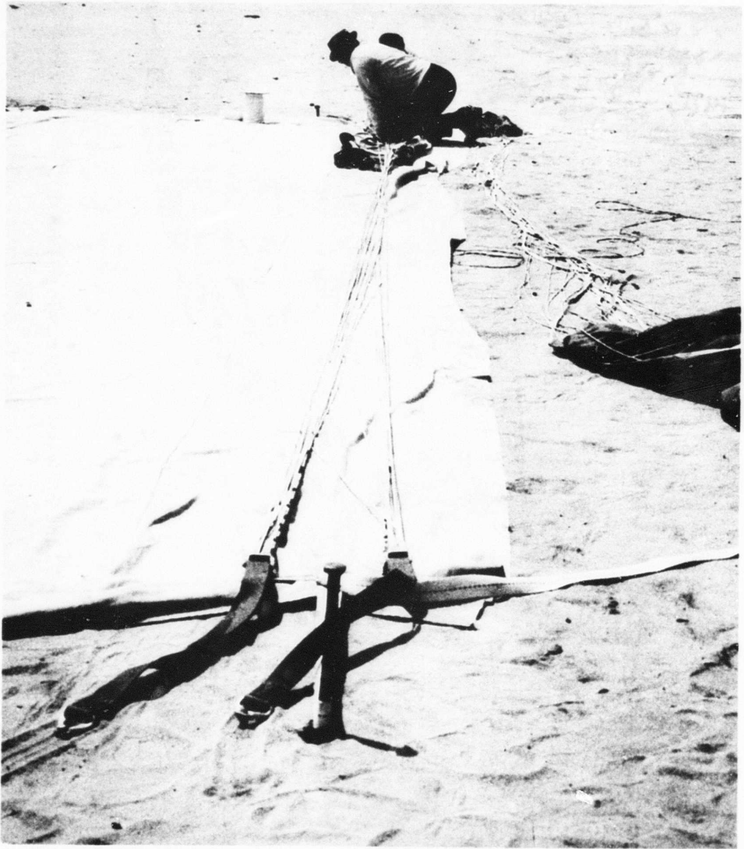
Figure 6. Line Position of Parawing With Pleating Complete.
