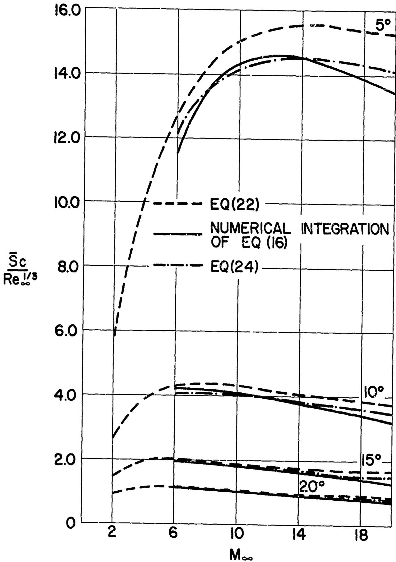
FIG. 9 SWALLOWING DISTANCE PARAMETER  $\bar{S}_c / R_{e_\infty}^{1/3}$  AS A FUNCTION OF FREESTREAM MACH NUMBER, ( $\bar{S}_c / R_{e_\infty}^{1/3}$  vs.  $M_\infty$ )
