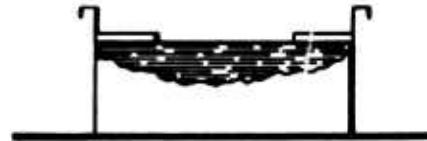
FLOATING ROOF TANK Roof deck moves with liquid level
