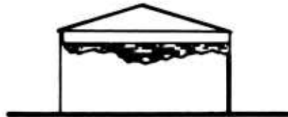
ORDINARY CONE ROOF TANK
