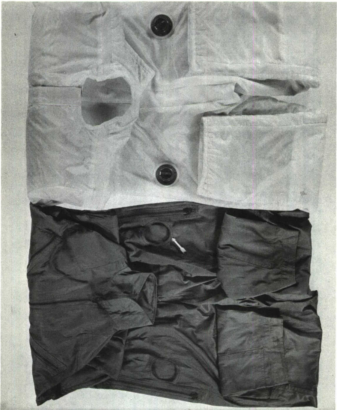
Figure 1. Adapted flight suit and ventilating liner (white) illustrating ram air inlet and adaptation of standard flight suit.
