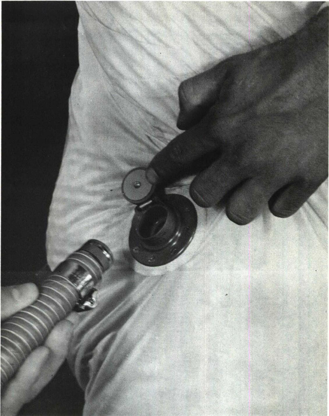
Figure 4. Quick disconnect for ram air hose.
