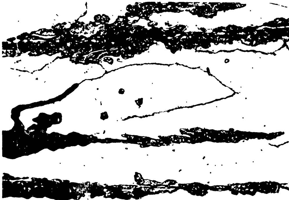
Figure 29. A portion of the area in Figure 28 showing that corrosion was along the grain boundaries and in the stringers of austenite decomposition product. Electrolytic oxalic acid etch; X500.
