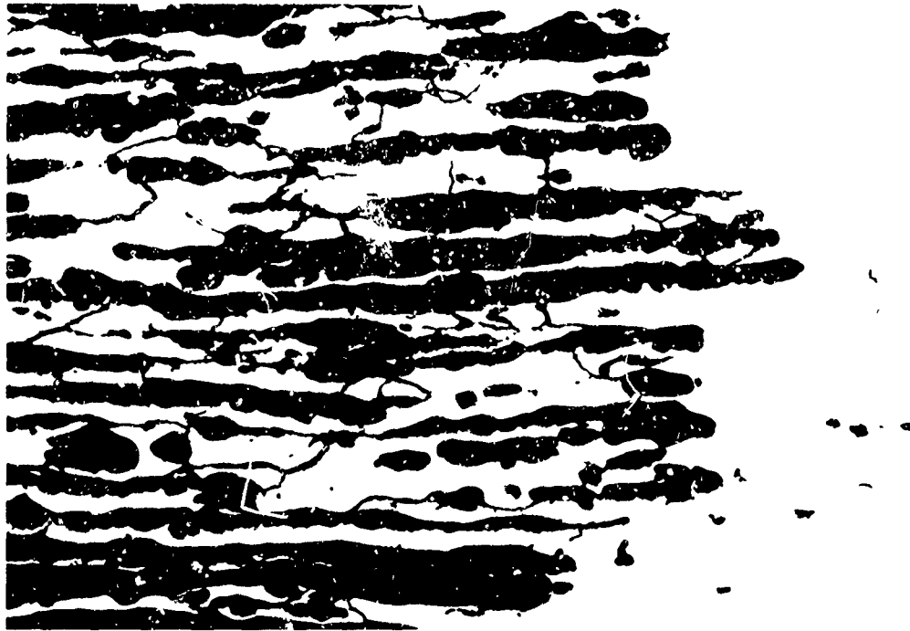
Figure 28. Edge corrosion in type 405 stainless steel showing corrosion at grain boundaries. Unetched; X100.
