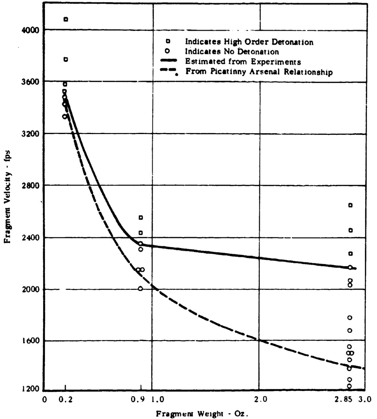
FIGURE 12 - BOUNDARY VELOCITY CURVE OF CYCLOTOL. SHOWING FRAGMENT IMPACT VELOCITY VERSUS FRAGMENT WEIGHT
