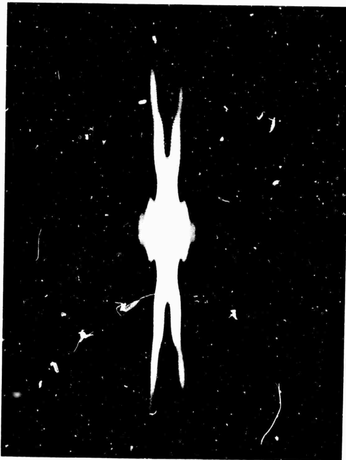
Figure 38. Enlarged Micrograph of Transform of Pie-Shaped Source
