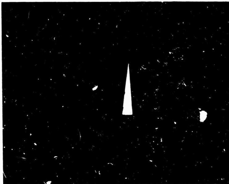
Figure 36. Micrograph of Pie-Shaped Source (100X)
