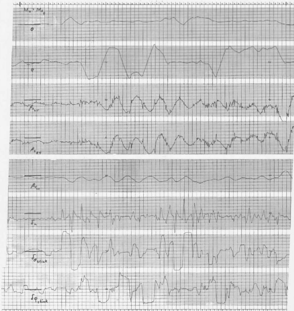
Fig. 3 Typical Time Histories of Simulated Flights Showing Variation of M_u
