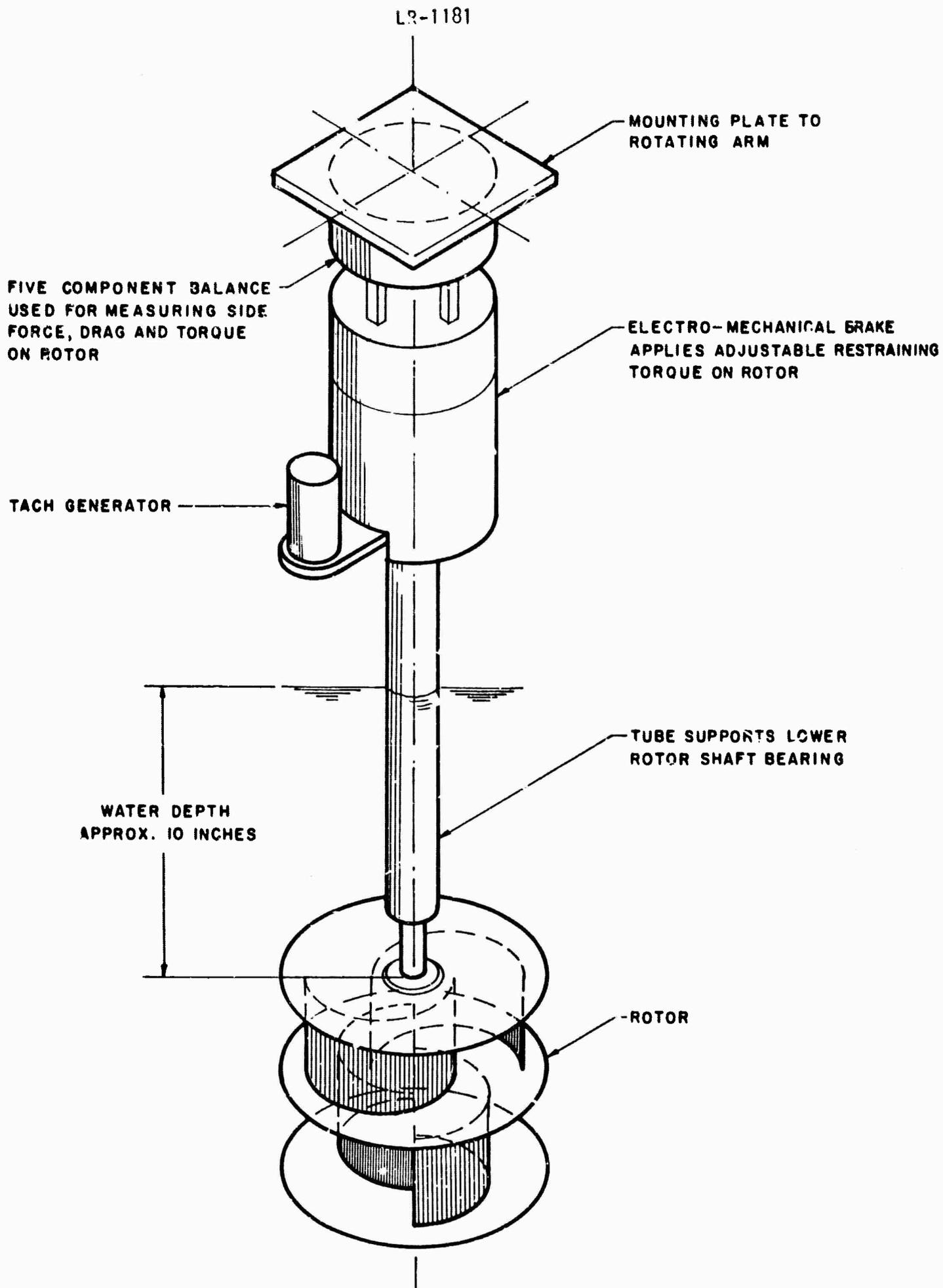
FIGURE 3. APPARATUS FOR TESTS OF SAVONIUS ROTOR MODELS
