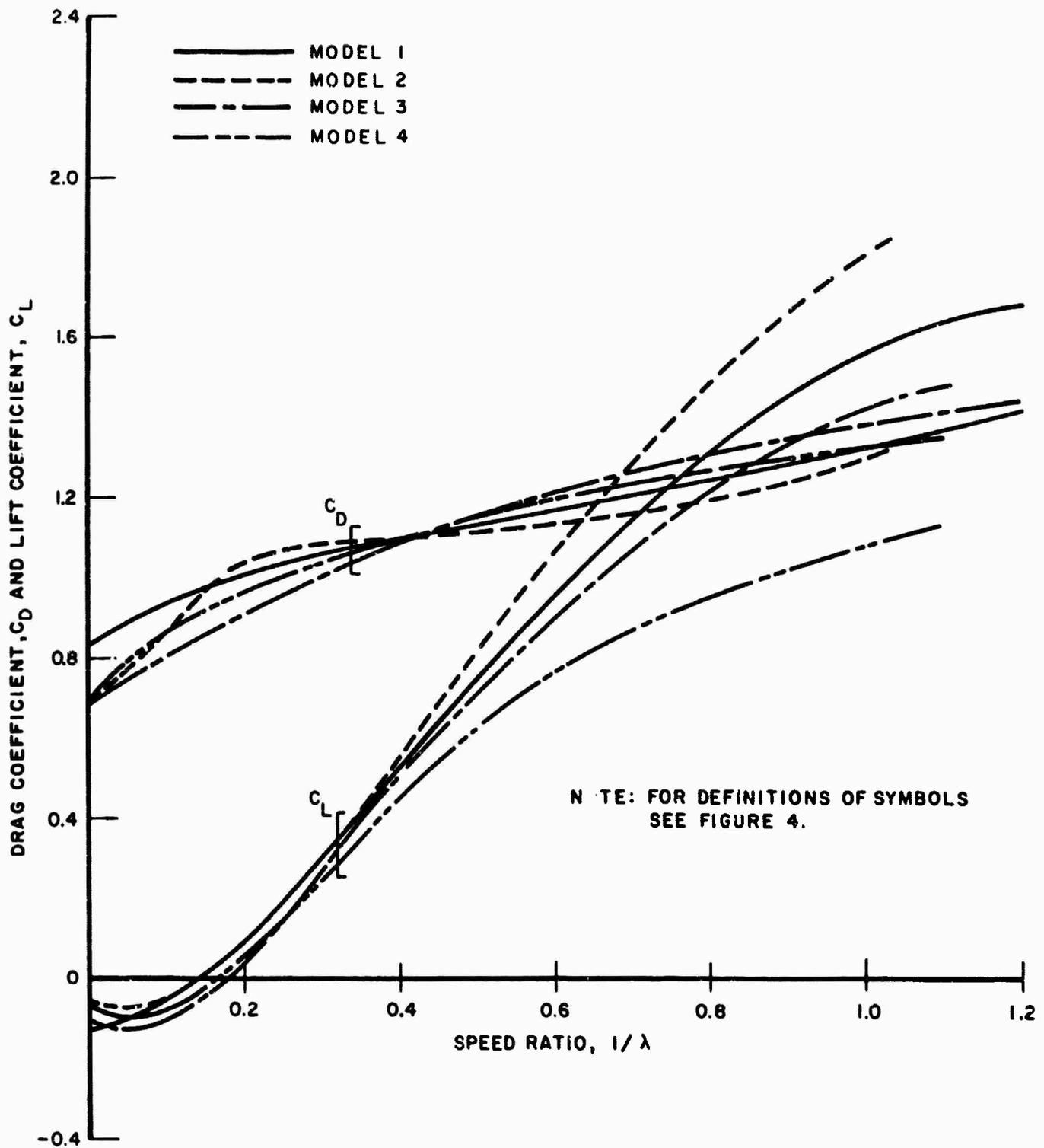
FIGURE 8. EFFECT OF ROTOR VANE TIP WIDTH ON DRAG AND SIDE FORCE FOR SAVONIUS ROTORS
