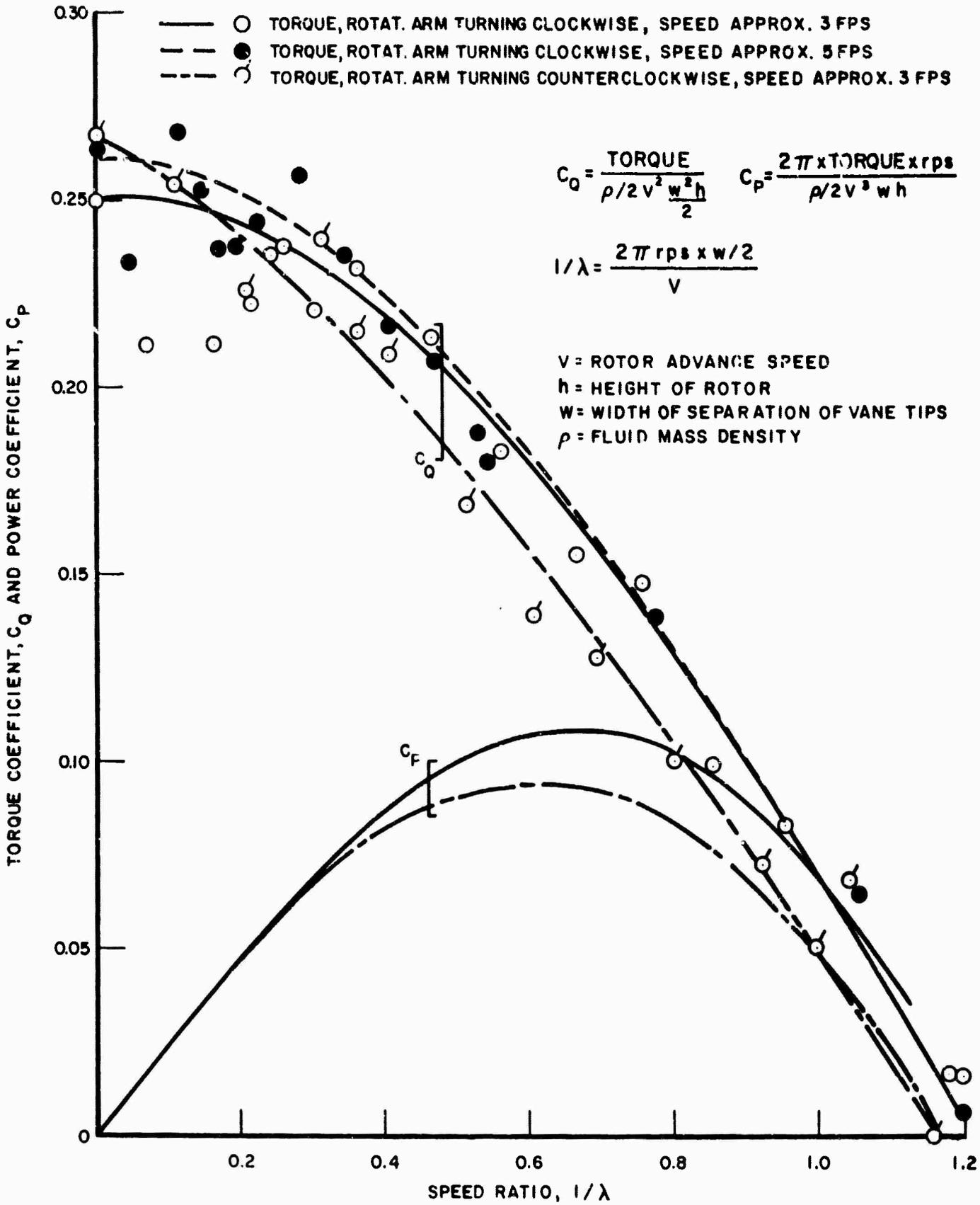
FIGURE 5. SAVONIUS ROTOR MODEL NO. I TEST RESULTS FOR TORQUE AND POWER
