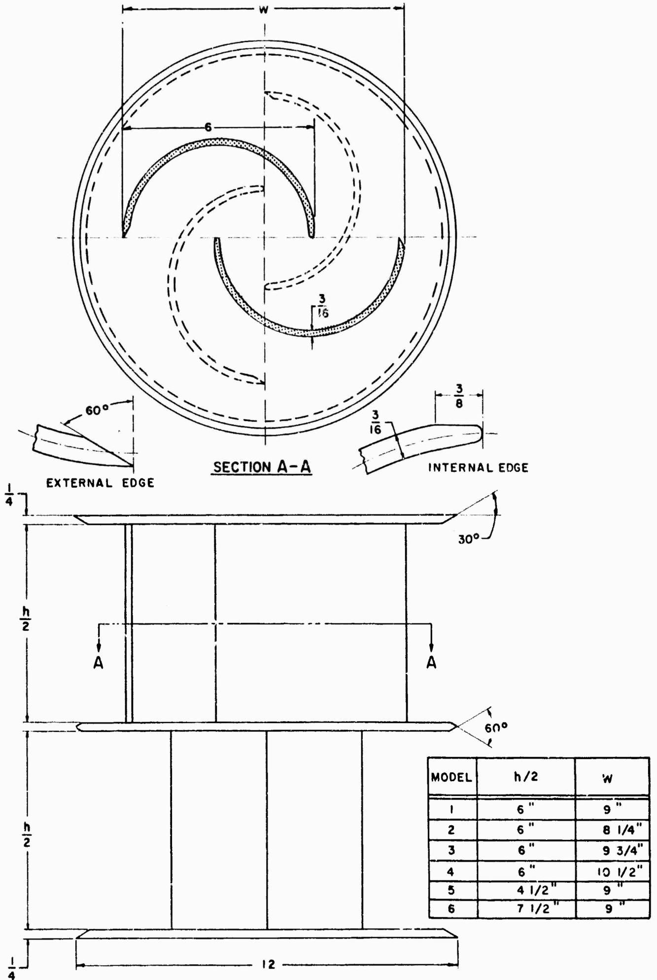
FIGURE 2. DETAILS OF SAVONIUS ROTOR MODEL GEOMETRIES
