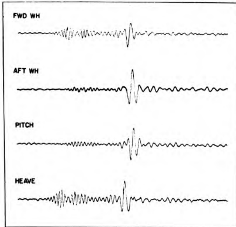
Fig. 26 - Record of transient test conducted with Model 4889 at zero speed in head waves
