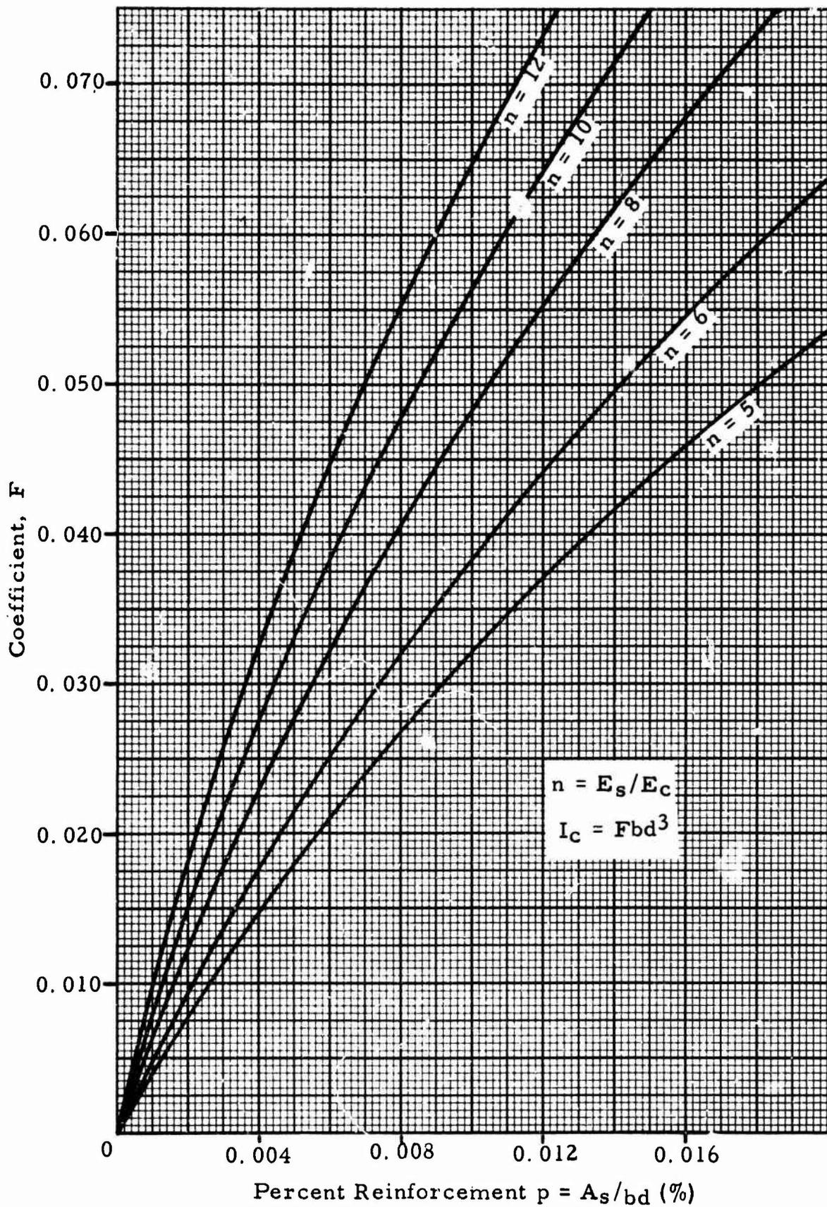
FIGURE B-15 COEFFICIENTS FOR MOMENT OF INERTIA
