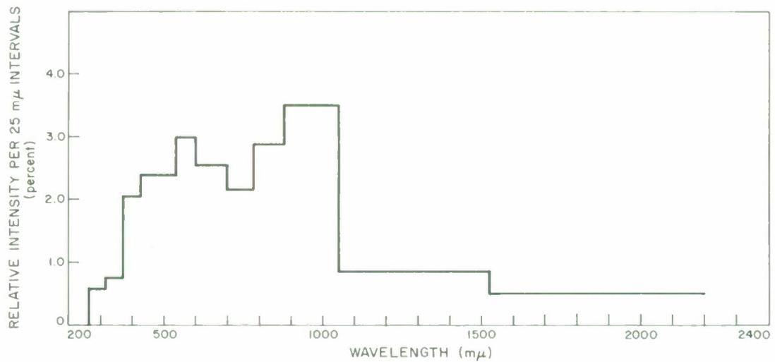
11. Xenon Arc Spectrum at 15 Kw.
