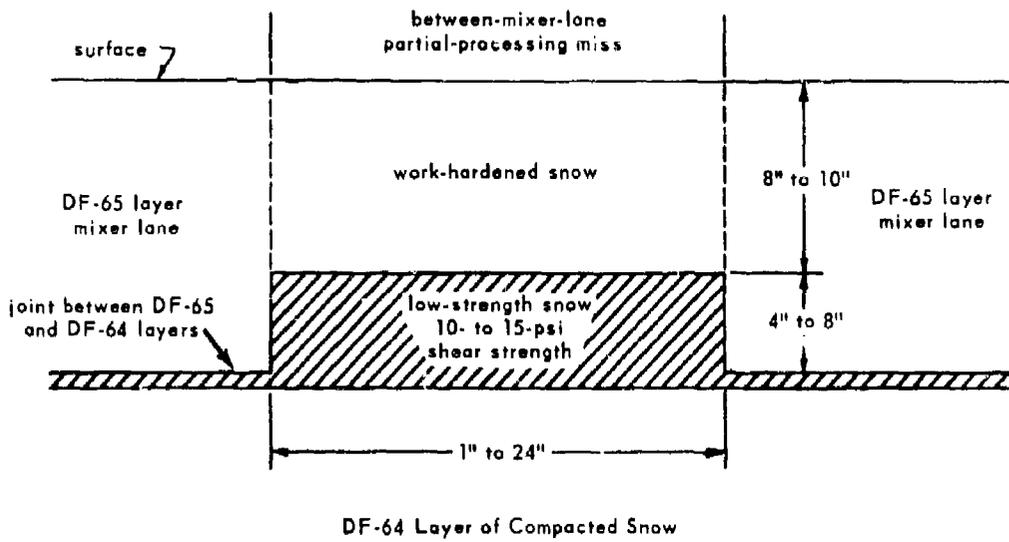
Figure 20. Cross section of a between-mixer-lane partial-processing miss in the DF-65 layer of compacted snow in 11 January 1965 test.
