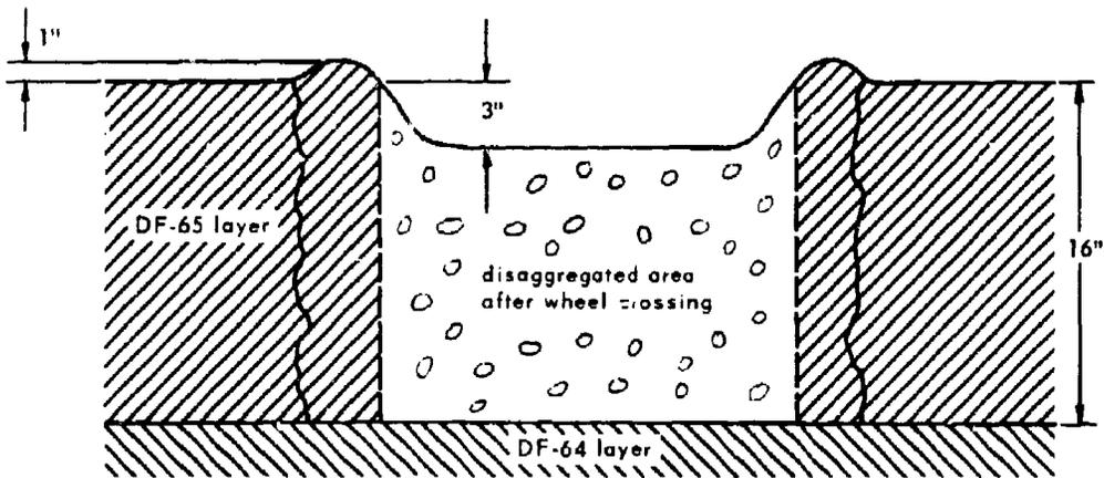
Section B-B. Wheel track in between-mixer-lane partial-processing miss
