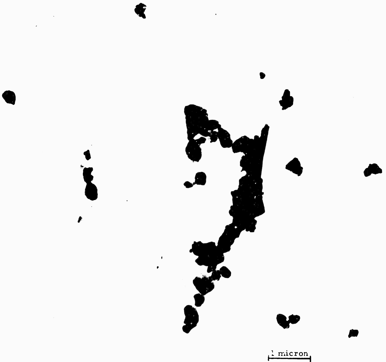
Fig. 9 Electron micrograph of an epoxy resin comminuted 72 hours at room temperature in the cryogenic ball mill (magnification is 15000X). The presence of small particles (0.2 microns) is shown. Similarly, the loose agglomeration of the small particles can be seen in this micrograph.
