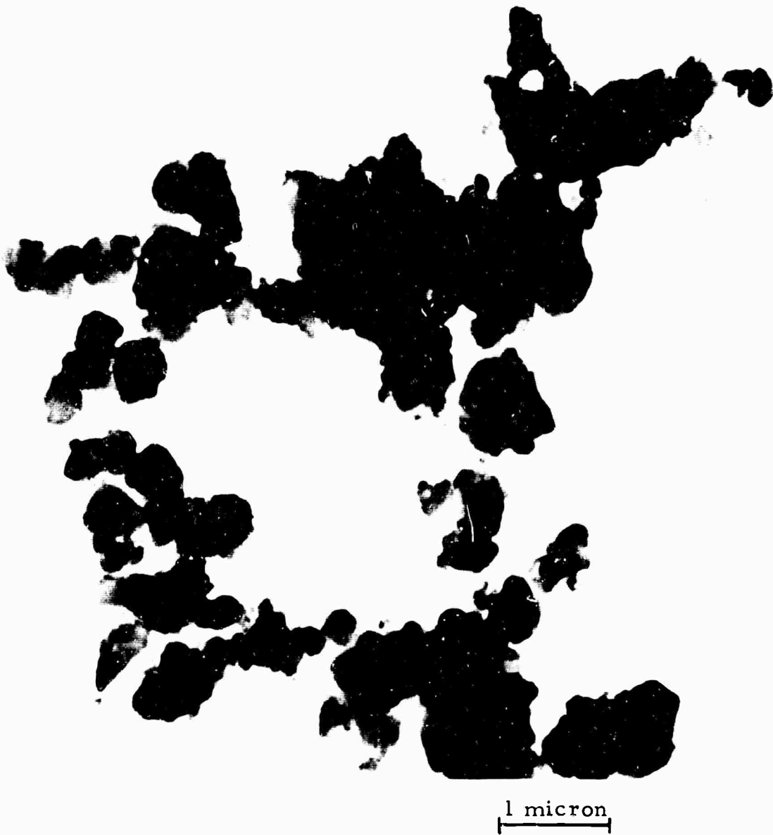
Fig. 10 Electron micrograph of an epoxy resin comminuted 72 hours at room temperature in the cryogenic ball mill (magnification is 15000X). The presence of small particles (0.2 microns) is shown. Similarly, the loose agglomeration of the small particles can be seen in this micrograph.
