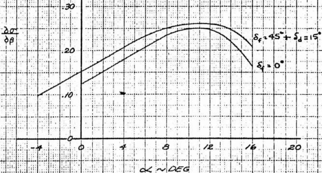
Figure 3.27 Rate of Change of Vertical Tail Sidewash Angle with Sideslip Angle,  $\frac{\partial \sigma}{\partial \beta}$ , vs Angle of Attack.
