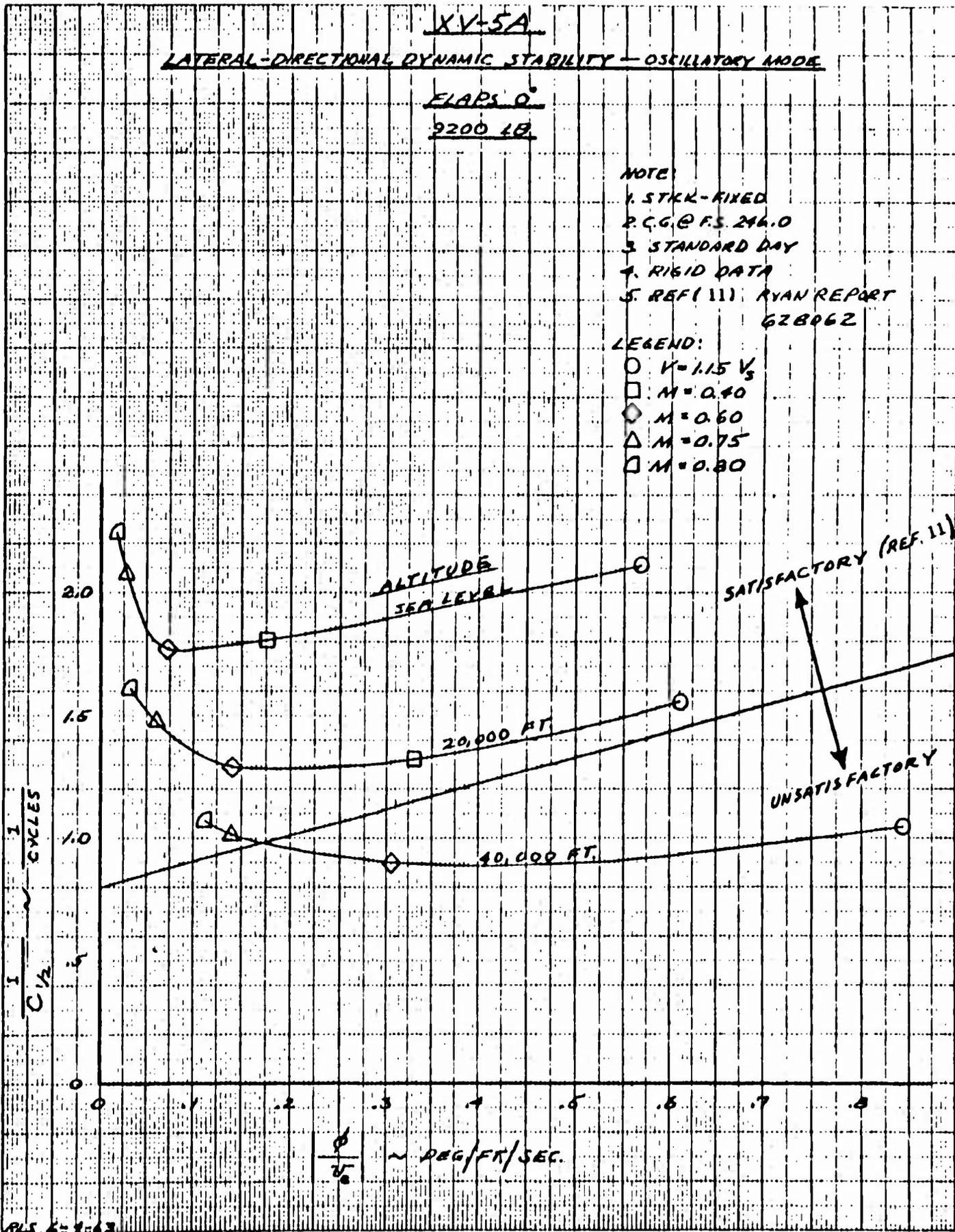
Figure 3.37 Lateral-Directional Dynamic Stability - Oscillatory Mode.  $\delta_f = 0^\circ$ .
