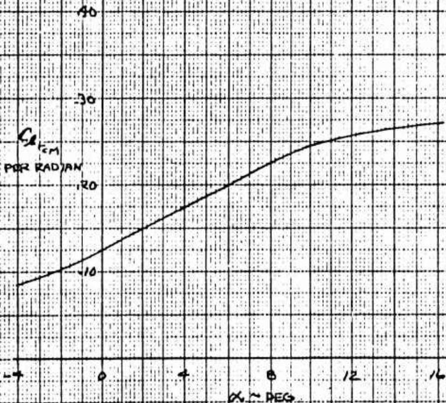
Figure 3.17 Rate of Change of Rolling Moment Coefficient with Yawing Velocity,  $C_{l_{r_{CM}}}$ , vs Angle of Attack.
