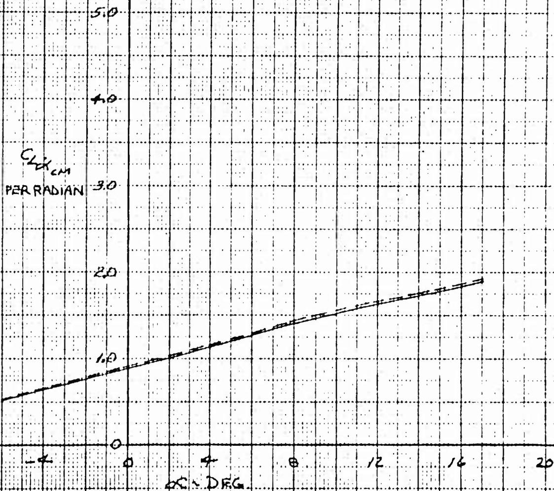
Figure 3.1 Rate of Change of Lift Coefficient with Rate of Change of Angle of Attack,  $C_{L\dot{\alpha}_{CM}}$ , vs Angle of Attack.
