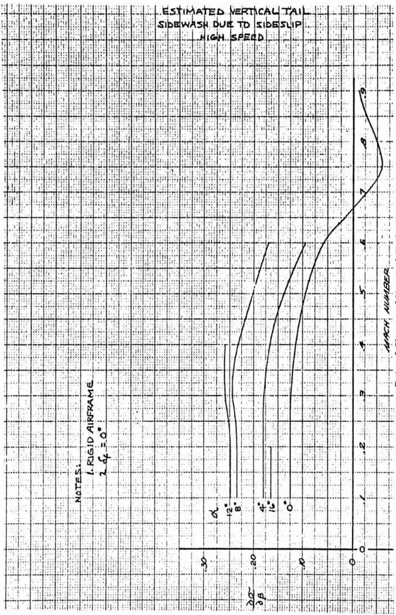
Figure 3.28 Rate of Change of Vertical Tail Sidewash Angle with Sideslip Angle,  $\frac{\partial \sigma}{\partial \beta}$ , vs Mach No.
