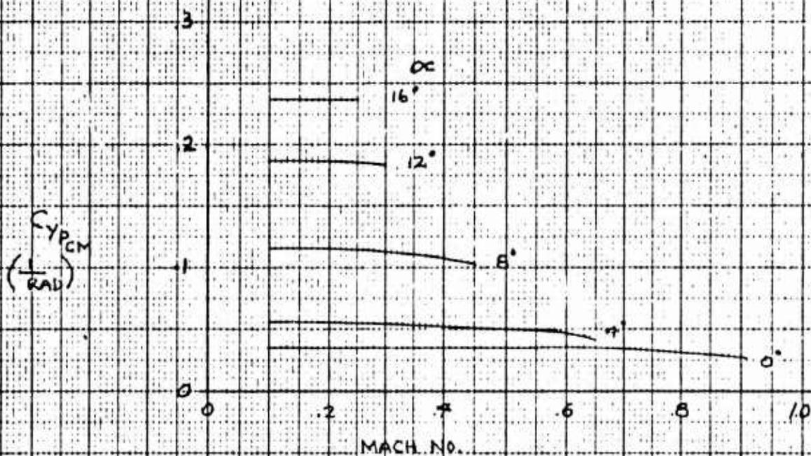
Figure 3.20 Rate of Change of Sideforce Coefficient with Rolling Velocity,  $C_{y_{PCM}}$ , vs Mach No.
