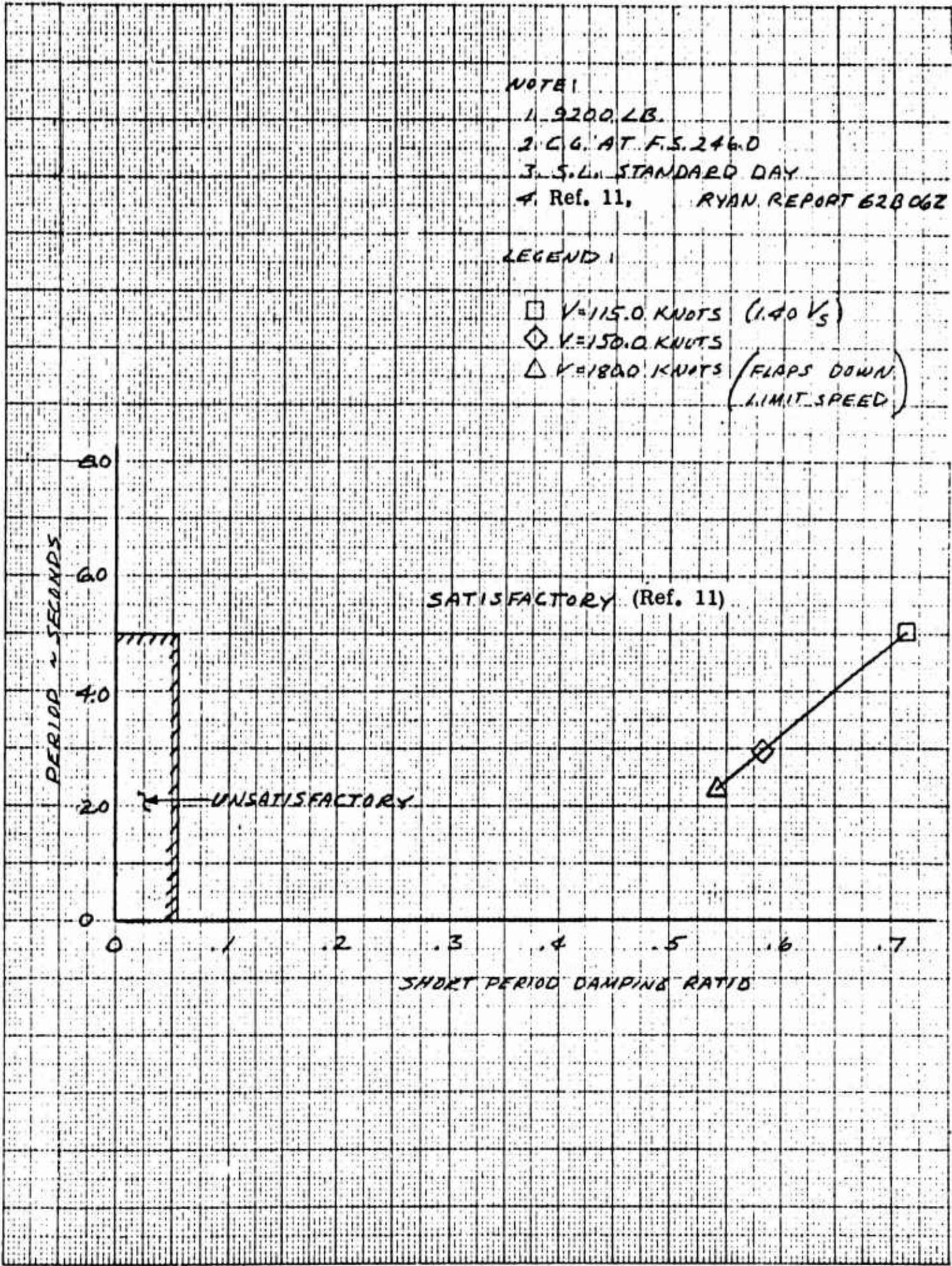
Figure 3.29 Longitudinal Dynamic Stability - Short Period
