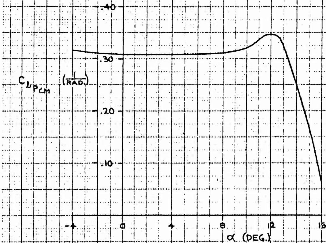
Figure 3.23 Rate of Change of Rolling Moment Coefficient with Rolling Velocity,  $C_{lP_{CM}}$ , vs Angle of Attack.
