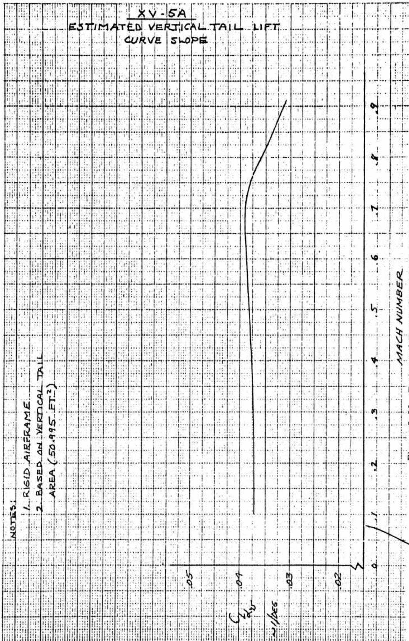
Figure 3.26 Estimated Vertical Tail Lift Curve Slope,  $CL_{\alpha}$ , vs Mach No.
