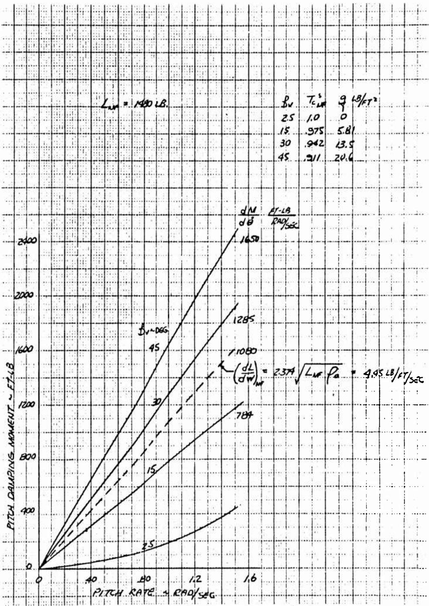
Figure 4.4 Estimated Pitch Damping Contribution of Nose Fan.
