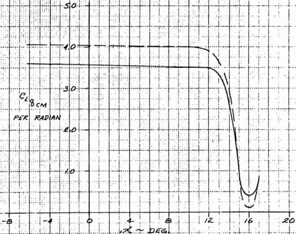
Figure 3.5 Rate of Change of Lift Coefficient with Pitching Velocity,  $C_{LqCM}$ , vs Angle of Attack.
