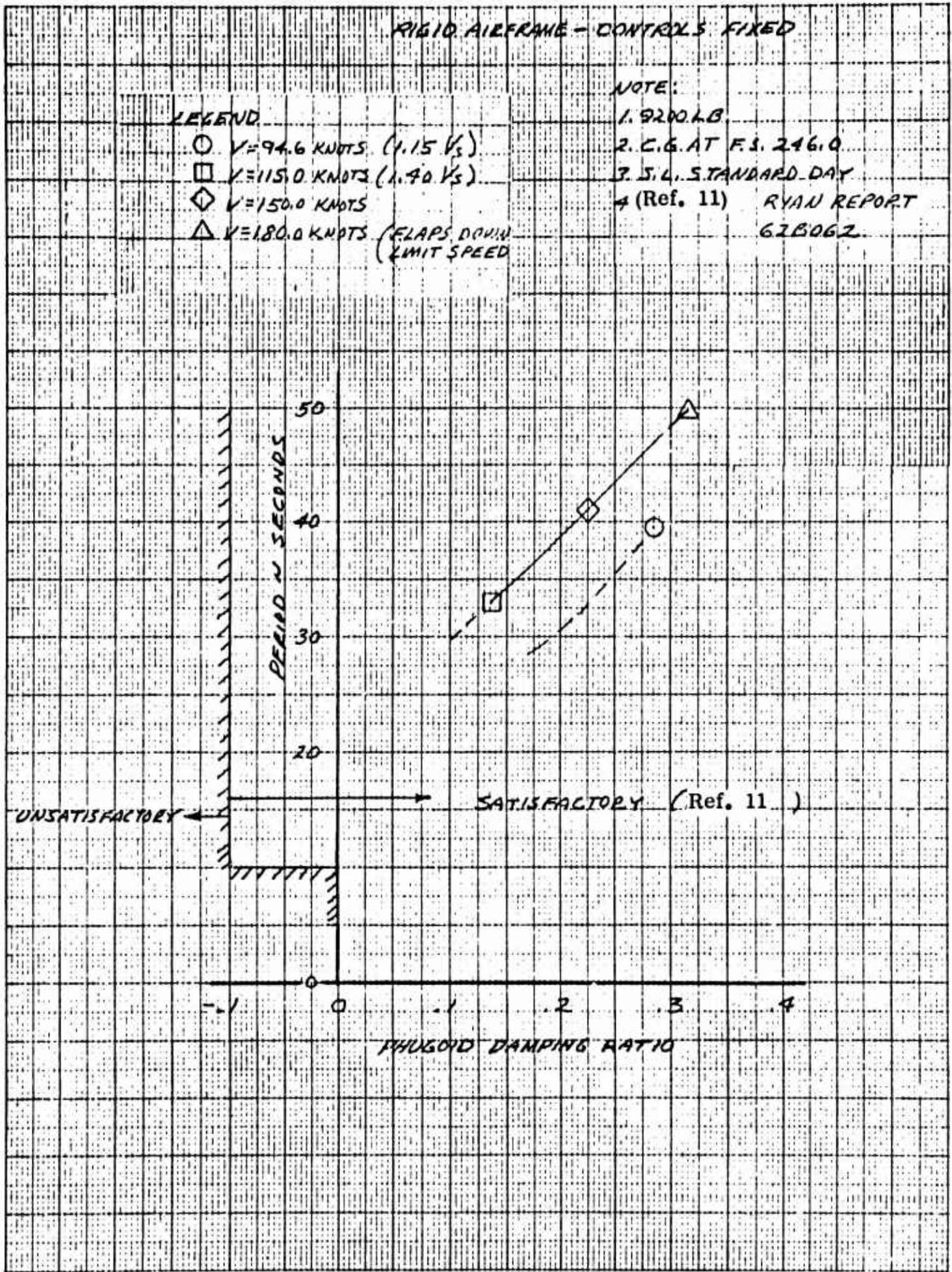
Figure 3.30 Longitudinal Dynamic Stability - Phugoid Mode.
