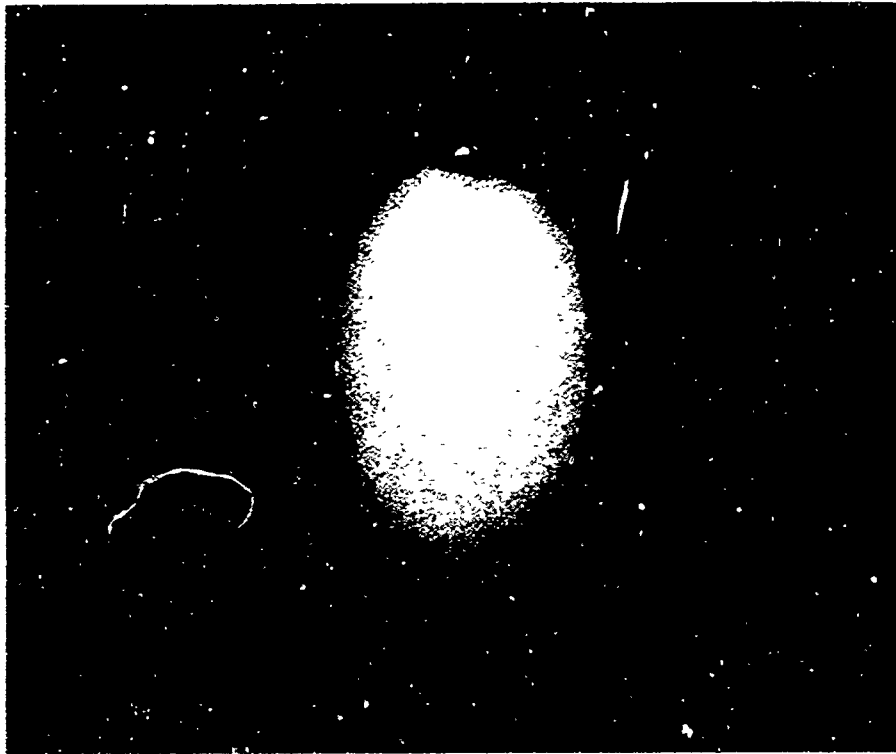
Fig. 2. Detonation products of 30-g charge photographed at 3.0 \times 10^{-6} sec.
