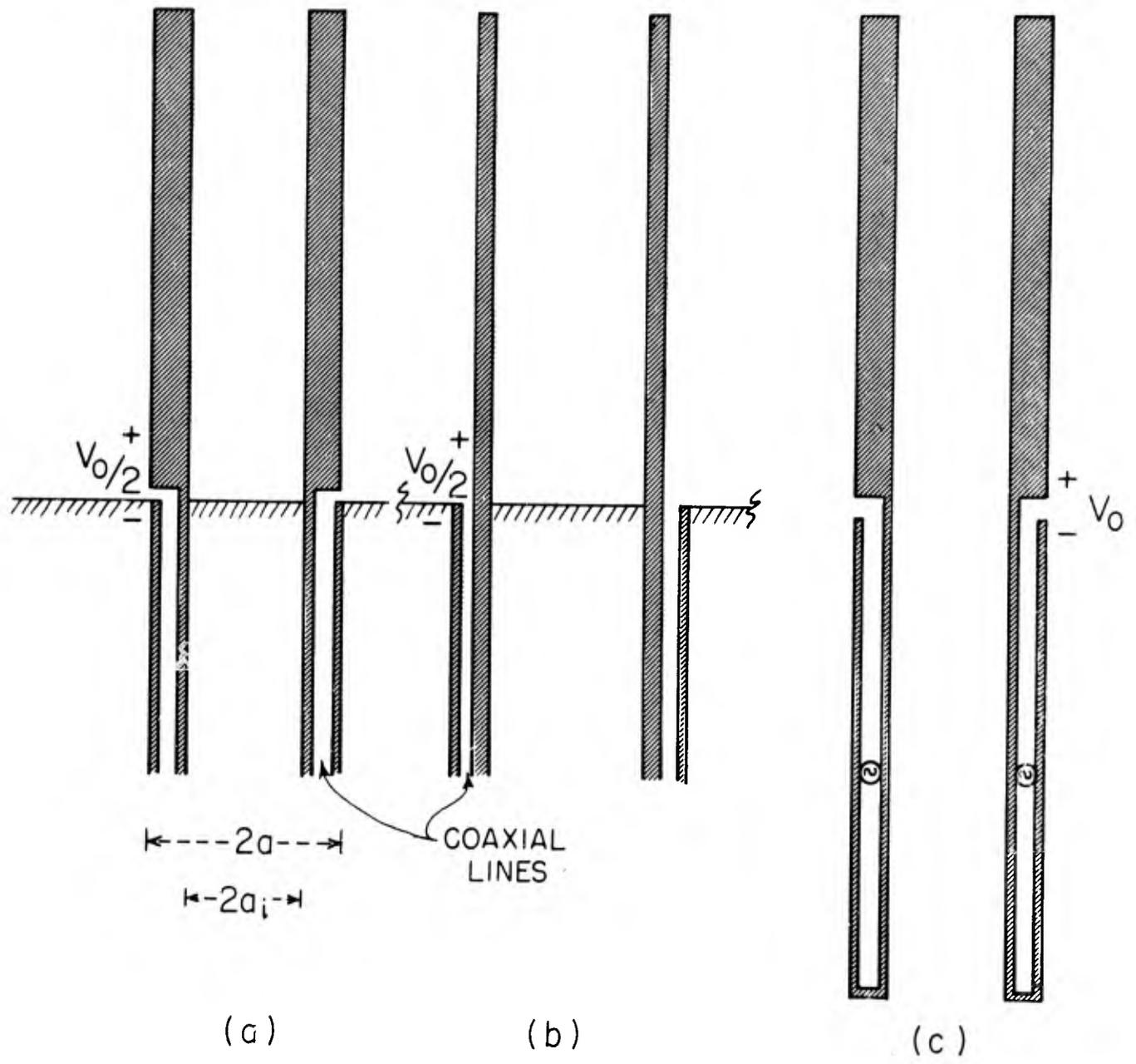
FIG. 2 ELECTRICALLY THICK ANTENNAS DRIVEN BY COAXIAL LINES
