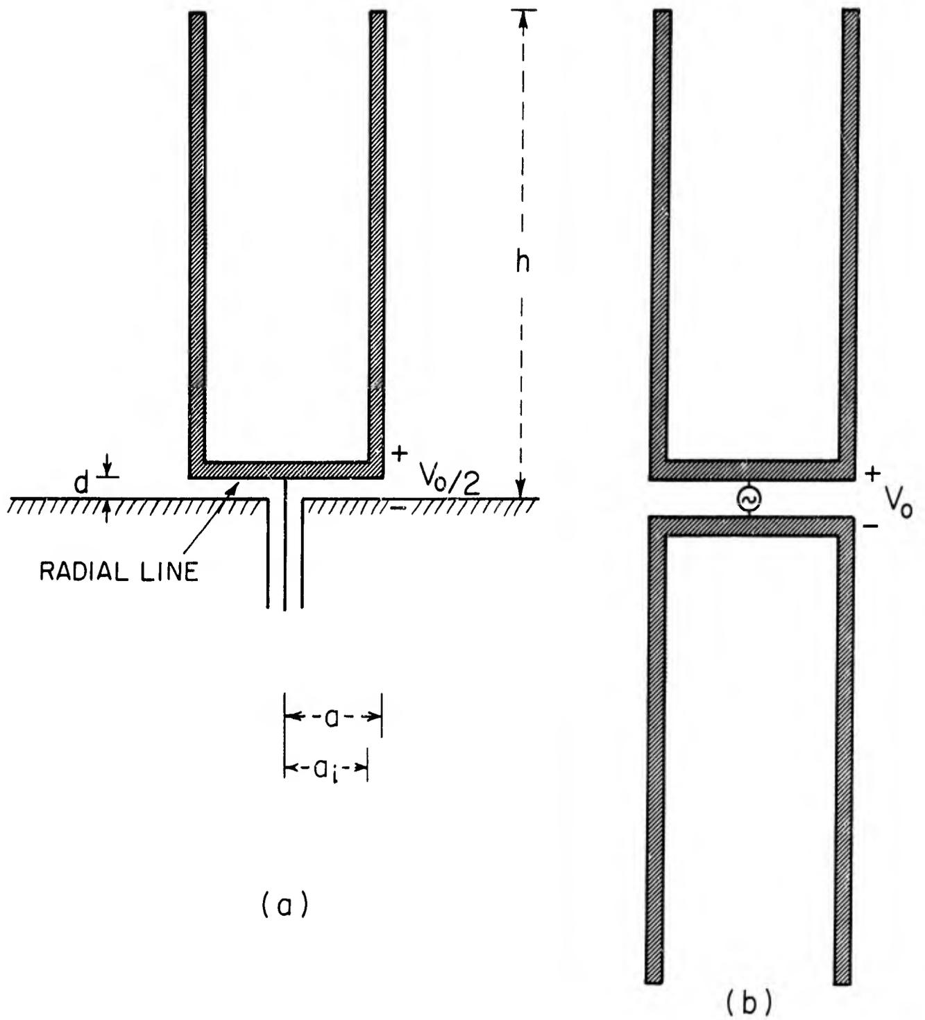
FIG. 1 ELECTRICALLY THICK ANTENNAS DRIVEN BY RADIAL TRANSMISSION LINES.
