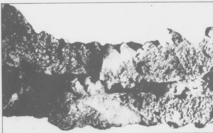
Fig. 6. Small internal fatigue fracture in weld metal. Note also the slag inclusions, poor penetration of weld metal, and rough weld beads. x 3.
