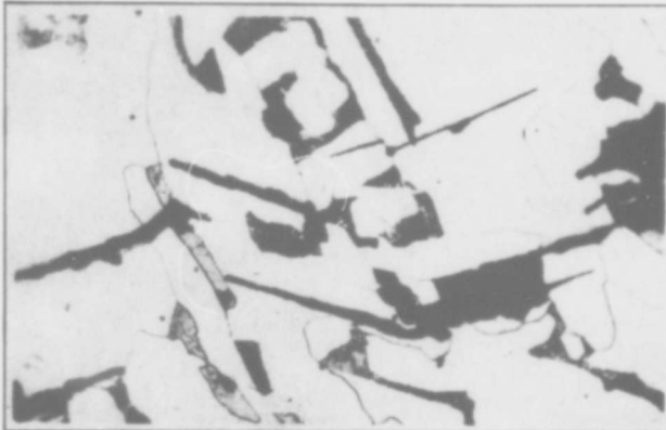
Fig. 21. Directional cracks adjacent to main fracture. x 500
