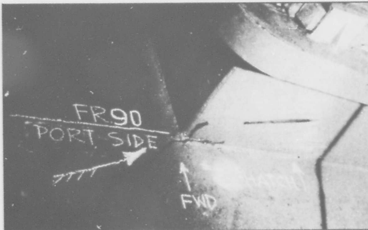
Fig. 5. Fracture originating at hatch corner of cargo vessel. (U. S. Coast Guard Photograph).
