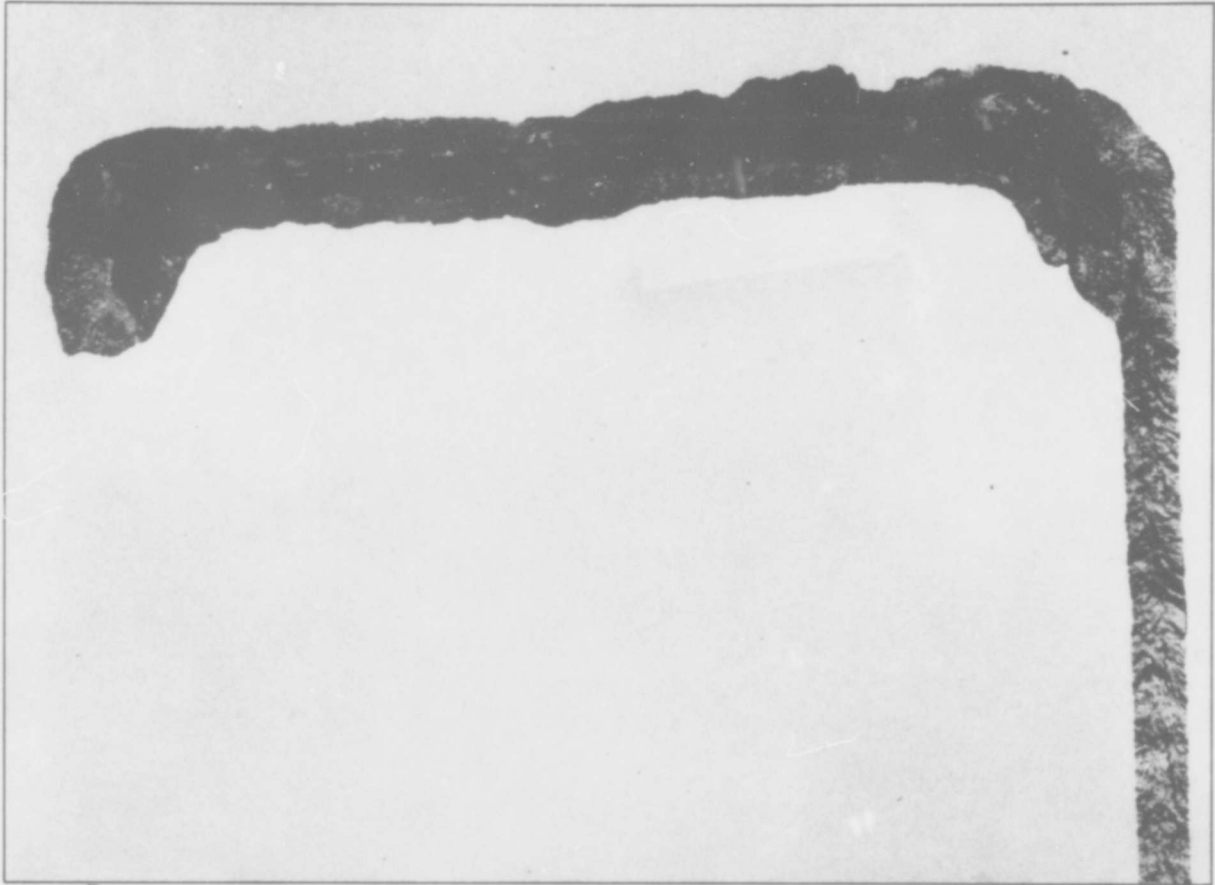
Fig. 9. Saddle weld in bulwark cap rail. Note the herringbone markings in bulwark plate (right) pointing to source of fracture in defective weld of cap rail (top). x 1.
