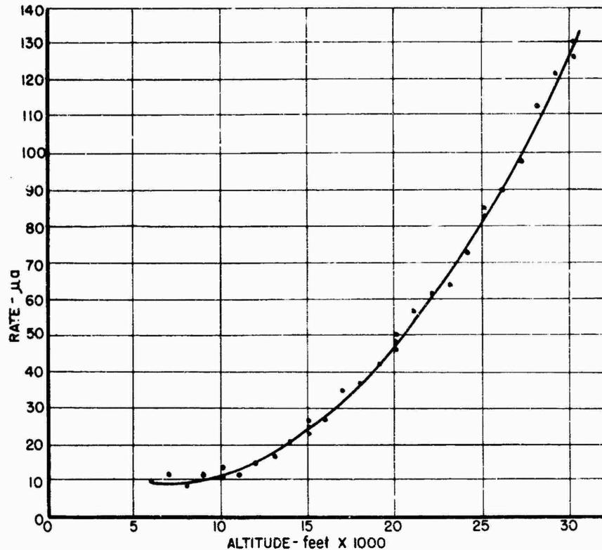
FIG. 56 Flight Calibration for Cosmic Ray Altimeter
