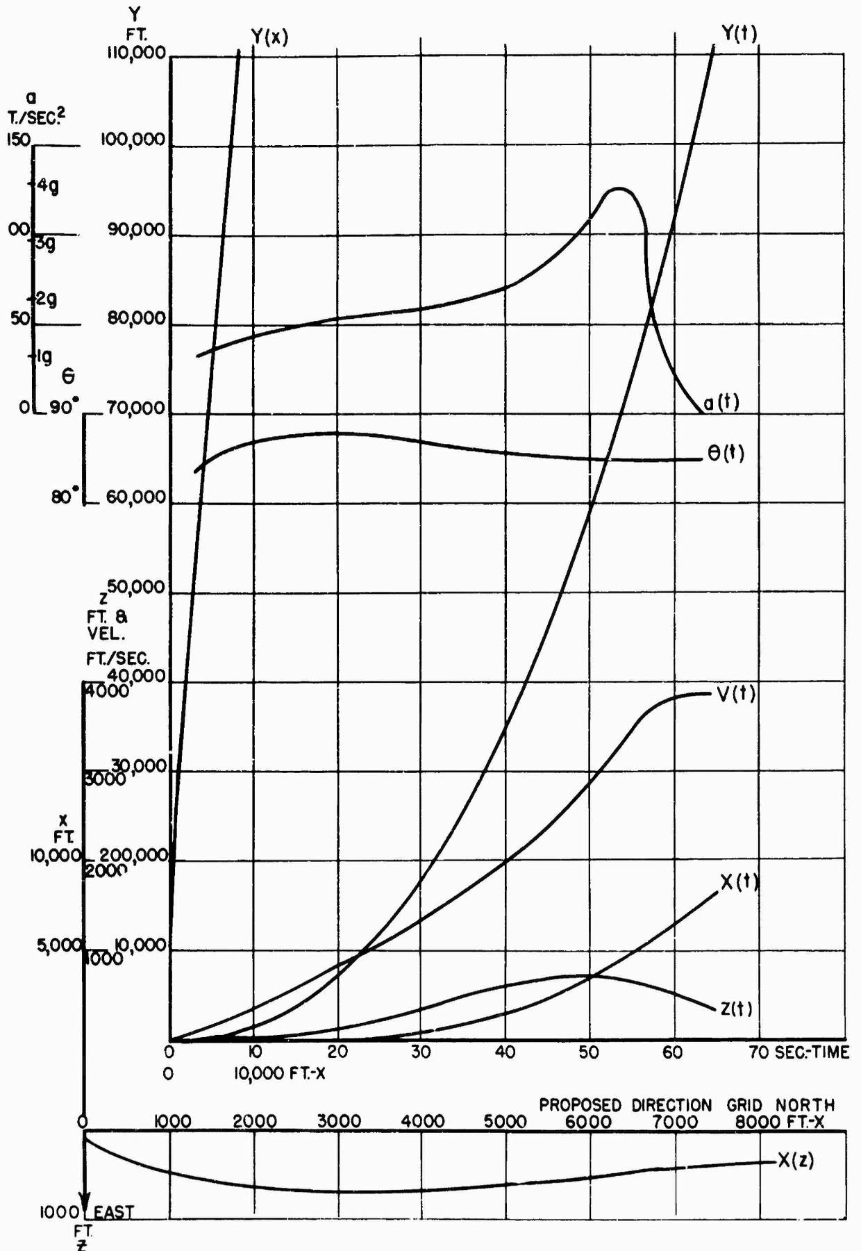
FIG. 13 Trajectory of A-4 (V-2) Rocket Launched 8 April 1947
