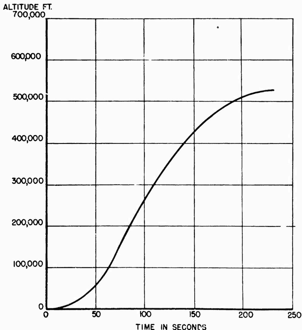
**FIG. 5** Trajectory of A-4 (V-2) Rocket Launched 30 July 1946
