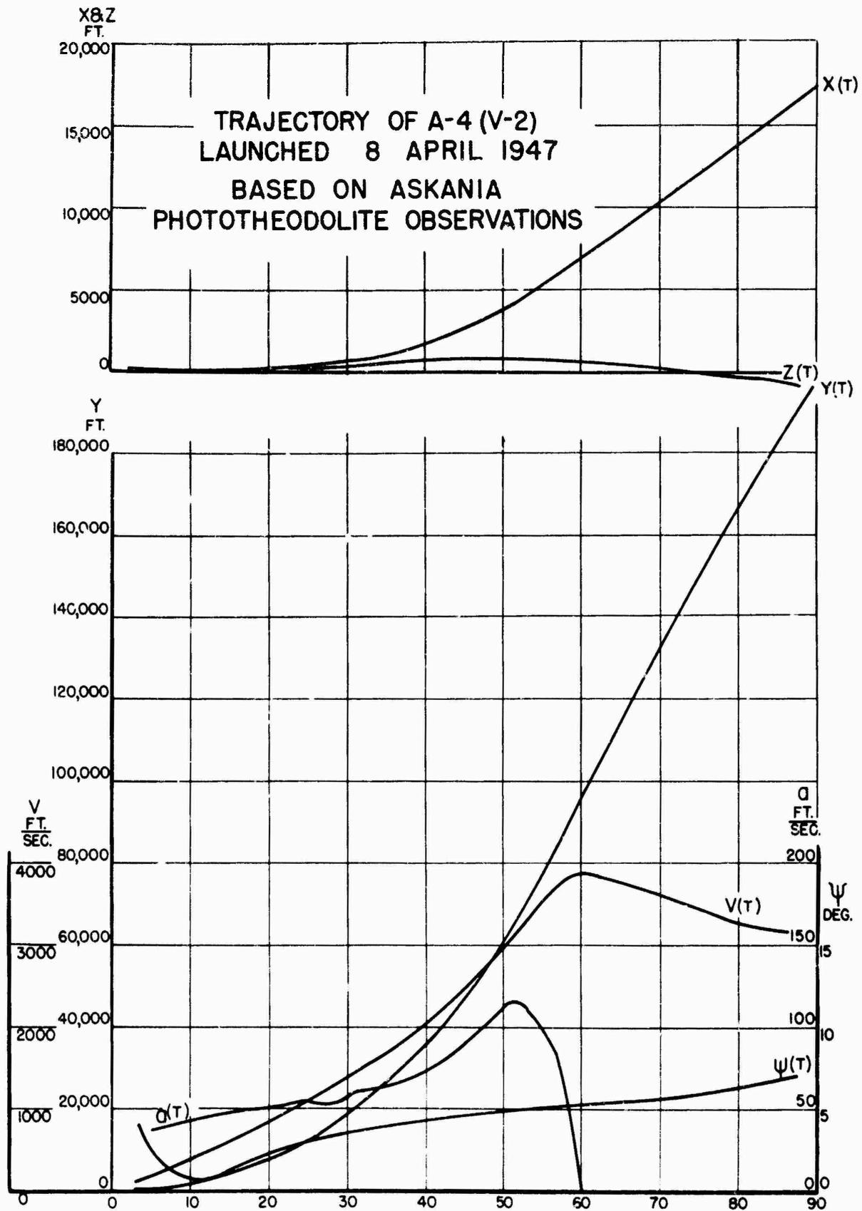
FIG. 15 Trajectory of A-4 (V-2) Rocket Launched 8 April 1947
