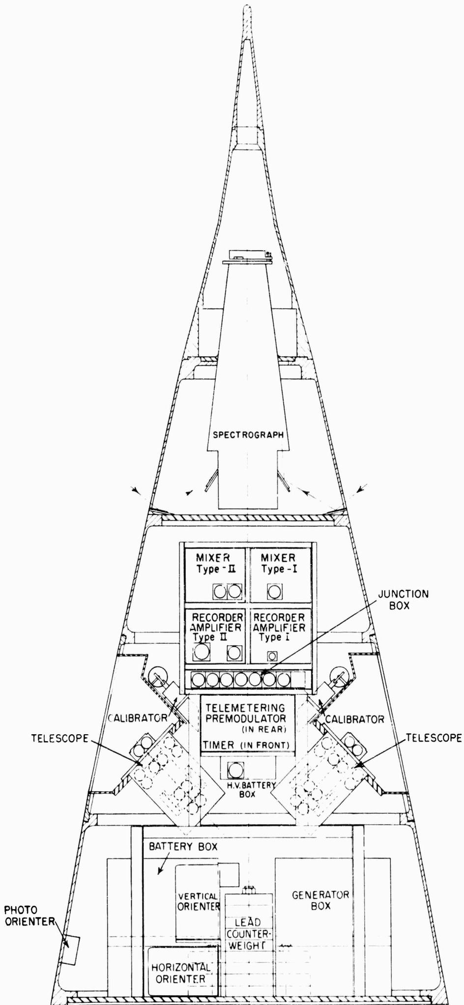
**FIG. 48    Warhead Instrumentation**
