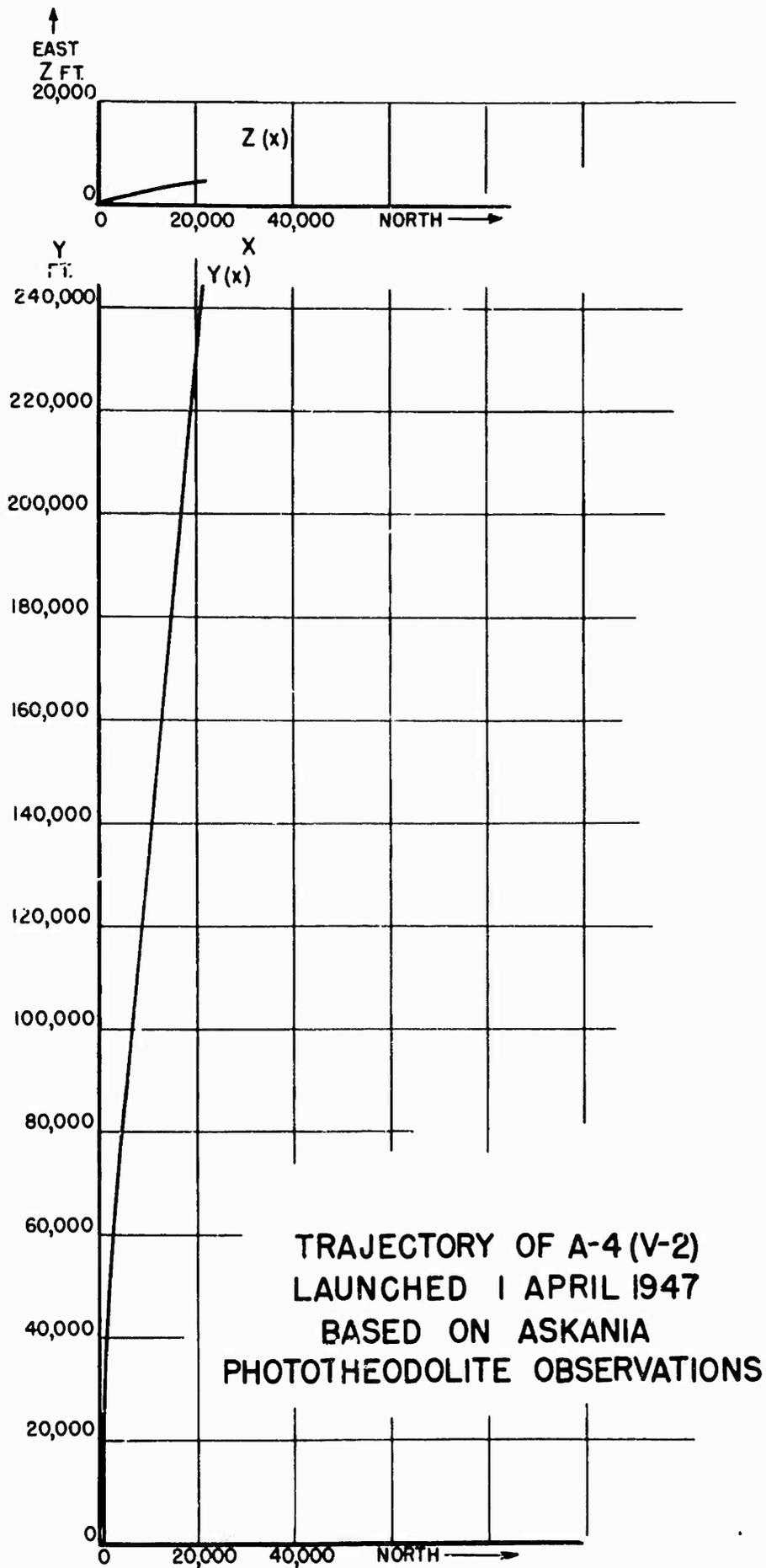
FIG. 10 Trajectory of A-4 (V-2) Rocket Launched 1 April 1947
