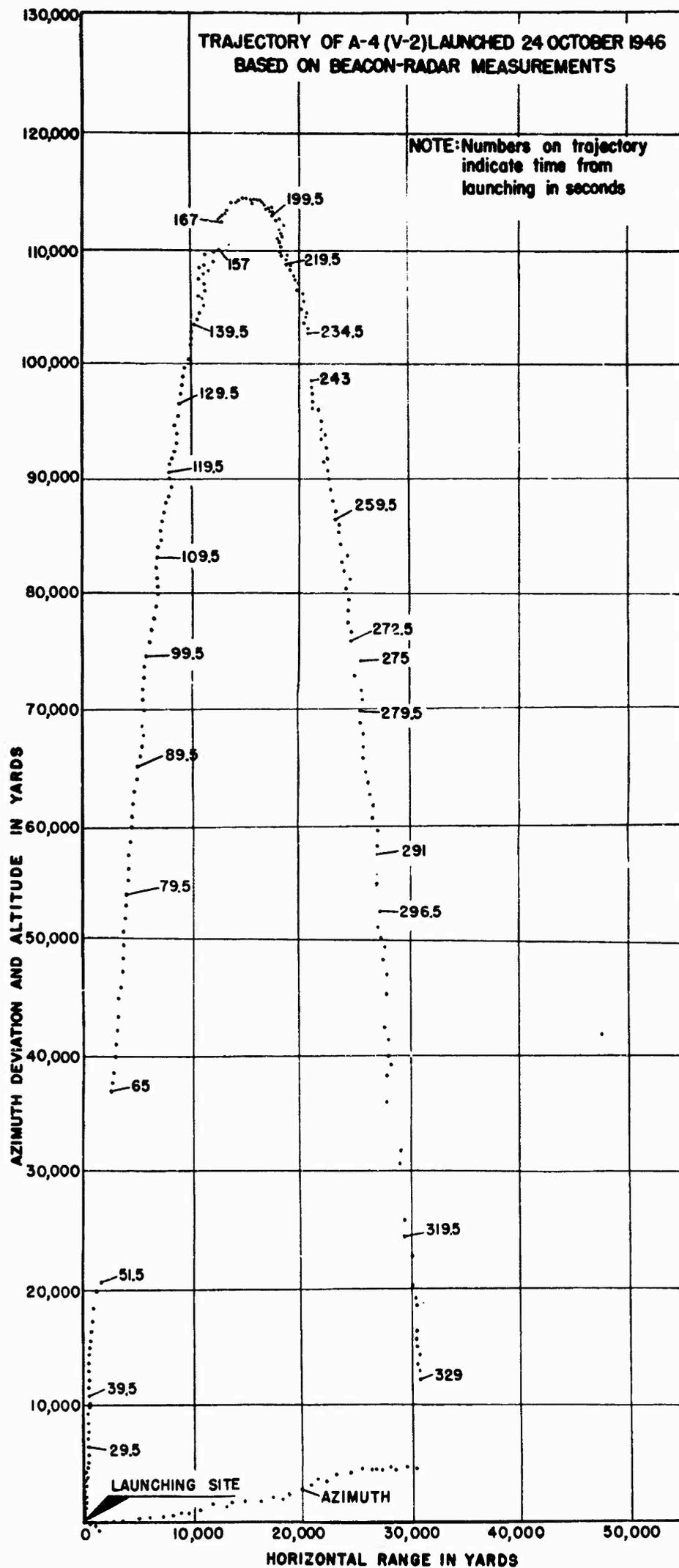
**FIG. 2** Trajectory of A-4 Launched 24 October 1946
