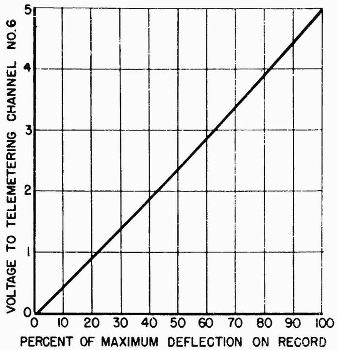
FIG. 20 Calibration Curve for Telemetering Channel No. 6
