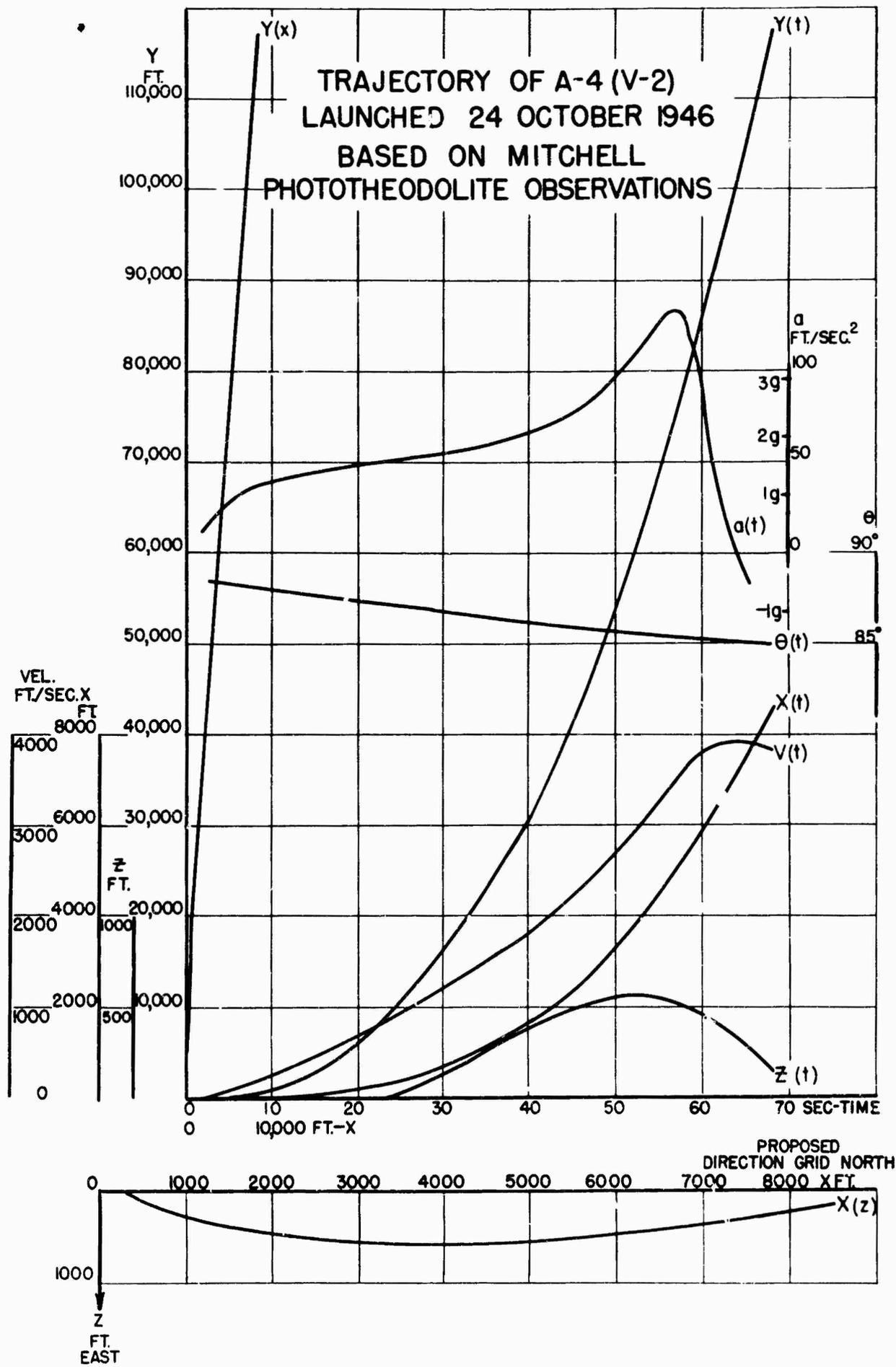
FIG. 6 Trajectory of A-4 (V-2) Rocket Launched 24 October 1946
