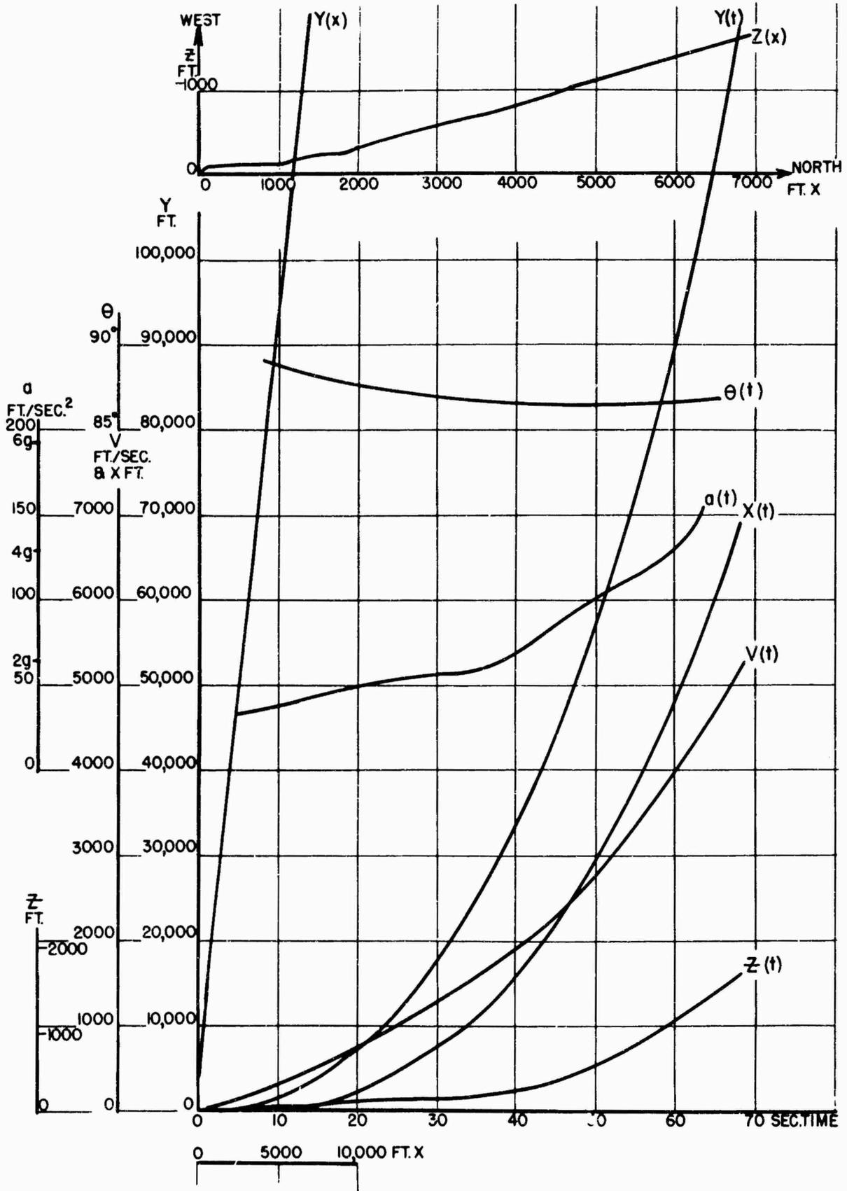
FIG. 7 Trajectory of A-4 (V-2) Rocket Launched 17 December 1946
