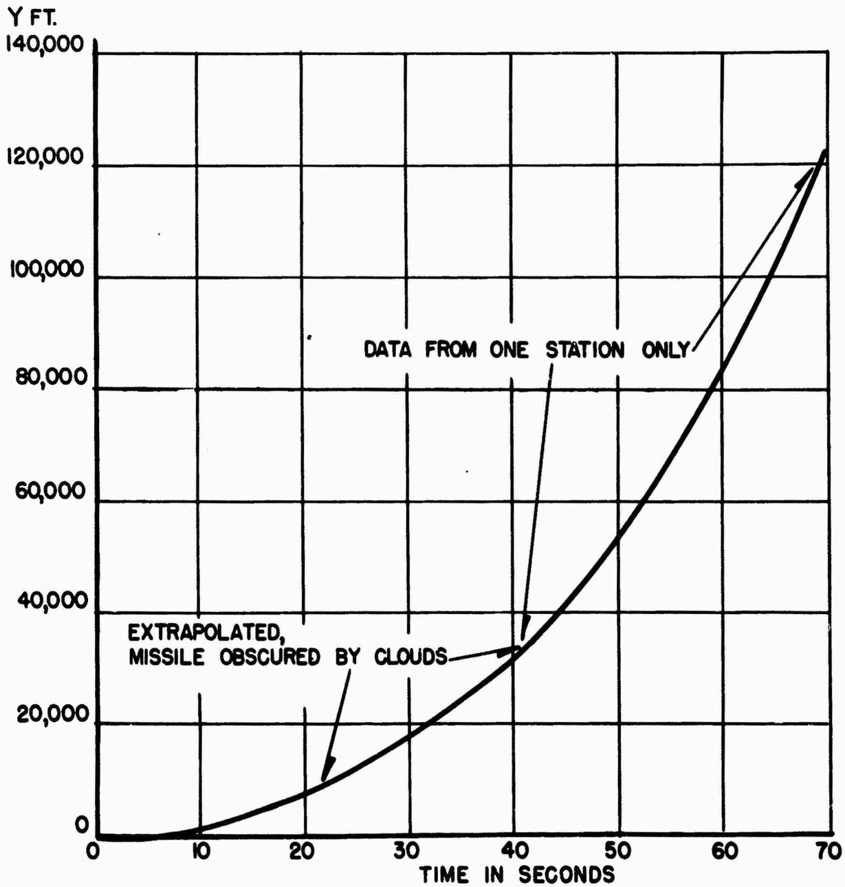
**FIG. 4 Trajectory of A-4 (V-2) Rocket Launched 30 July 1946**
