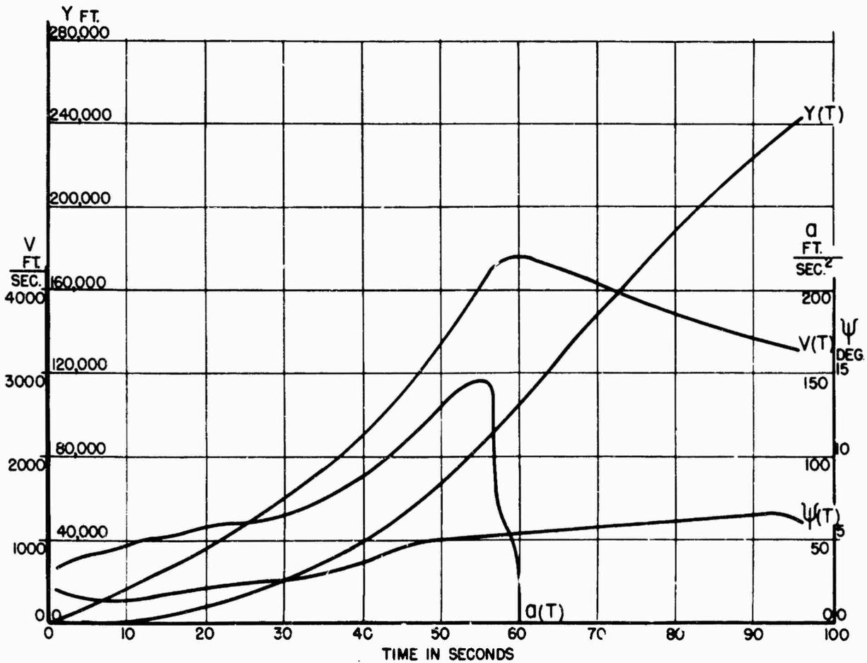
**FIG. 12** Trajectory of A-4 (V-2) Rocket Launched 1 April 1947
