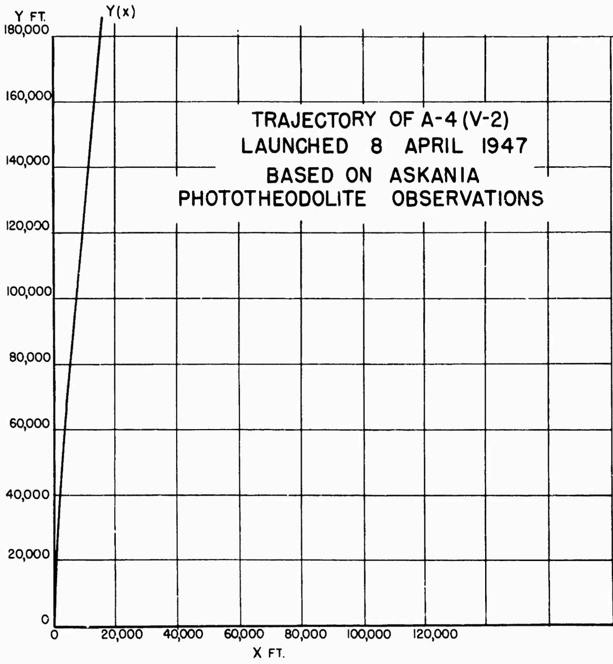
FIG. 14 Trajectory of A-4 (V-2) Rocket Launched 8 April 1947
