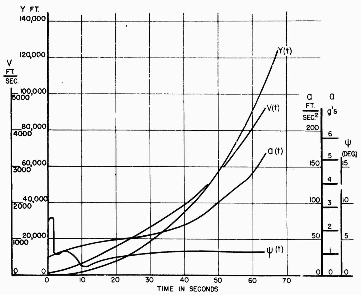
**FIG. 9 Trajectory of A-4 (V-2) Rocket Launched 17 December 1946**
