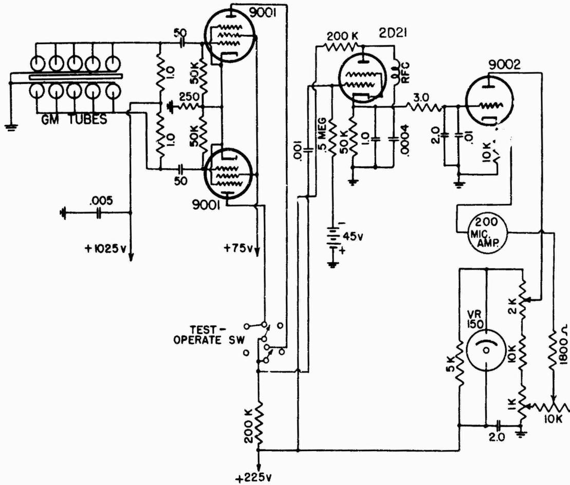
FIG. 54 Cosmic Ray Altimeter Circuit
