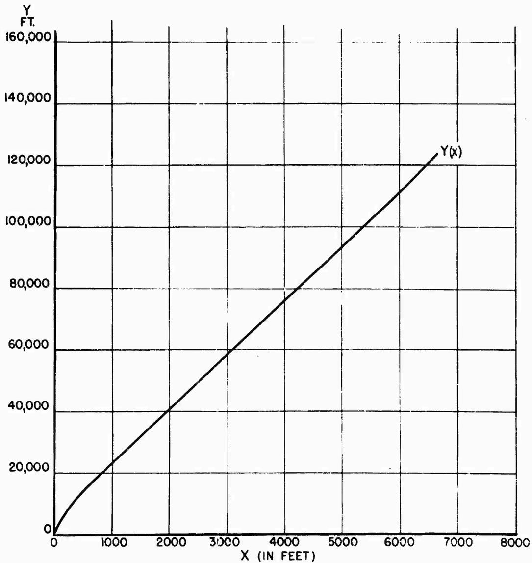
FIG. 8 Trajectory of A-4 (V-2) Rocket Launched 17 December 1946
