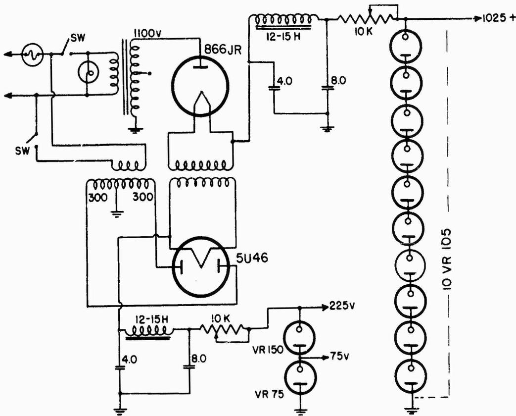
FIG. 55 Power Supply Circuit for Cosmic Ray Altimeter
