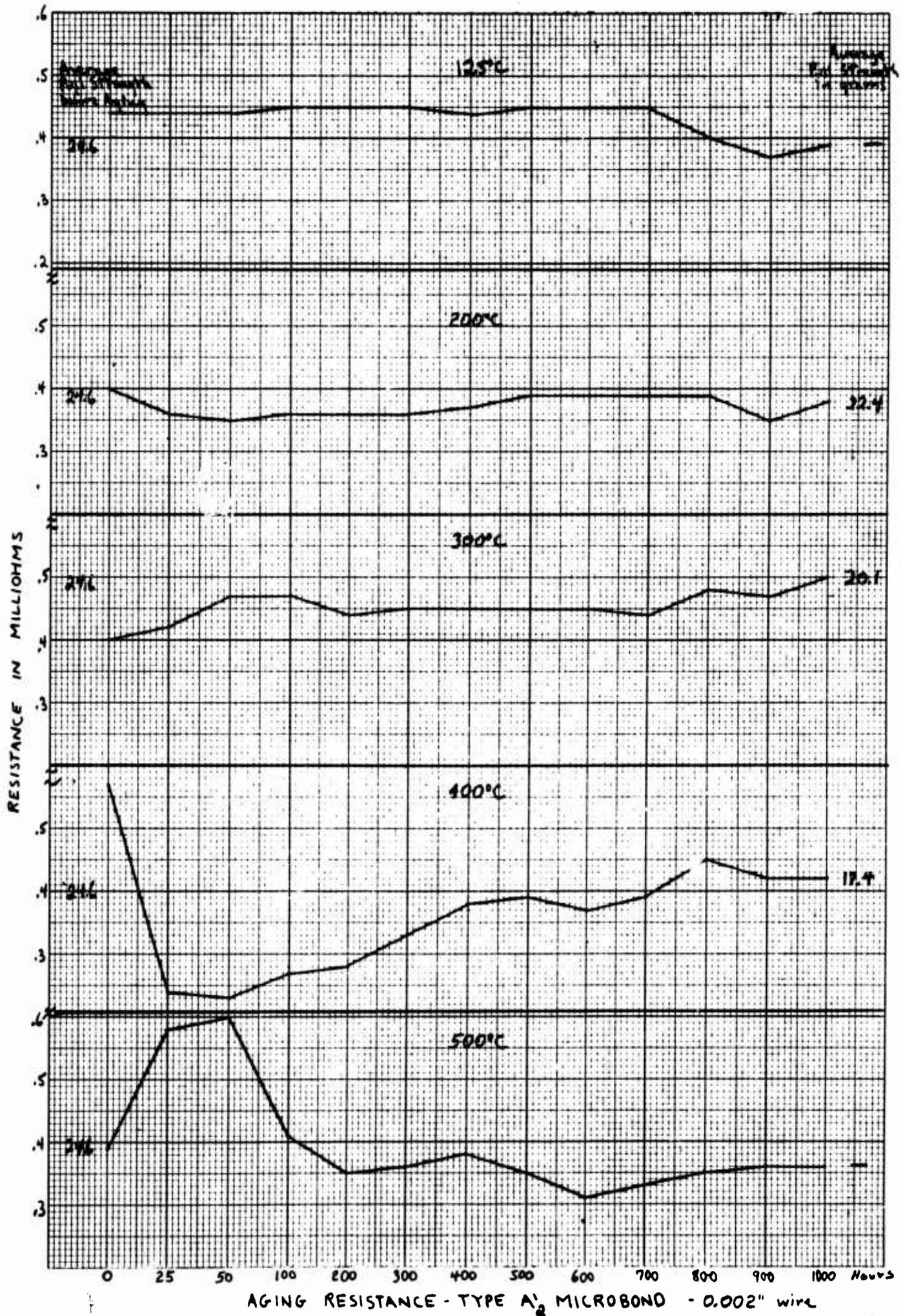
Figure 52 Resistance vs Thermal Aging Time - Type A<sub>2</sub> Microbonds
