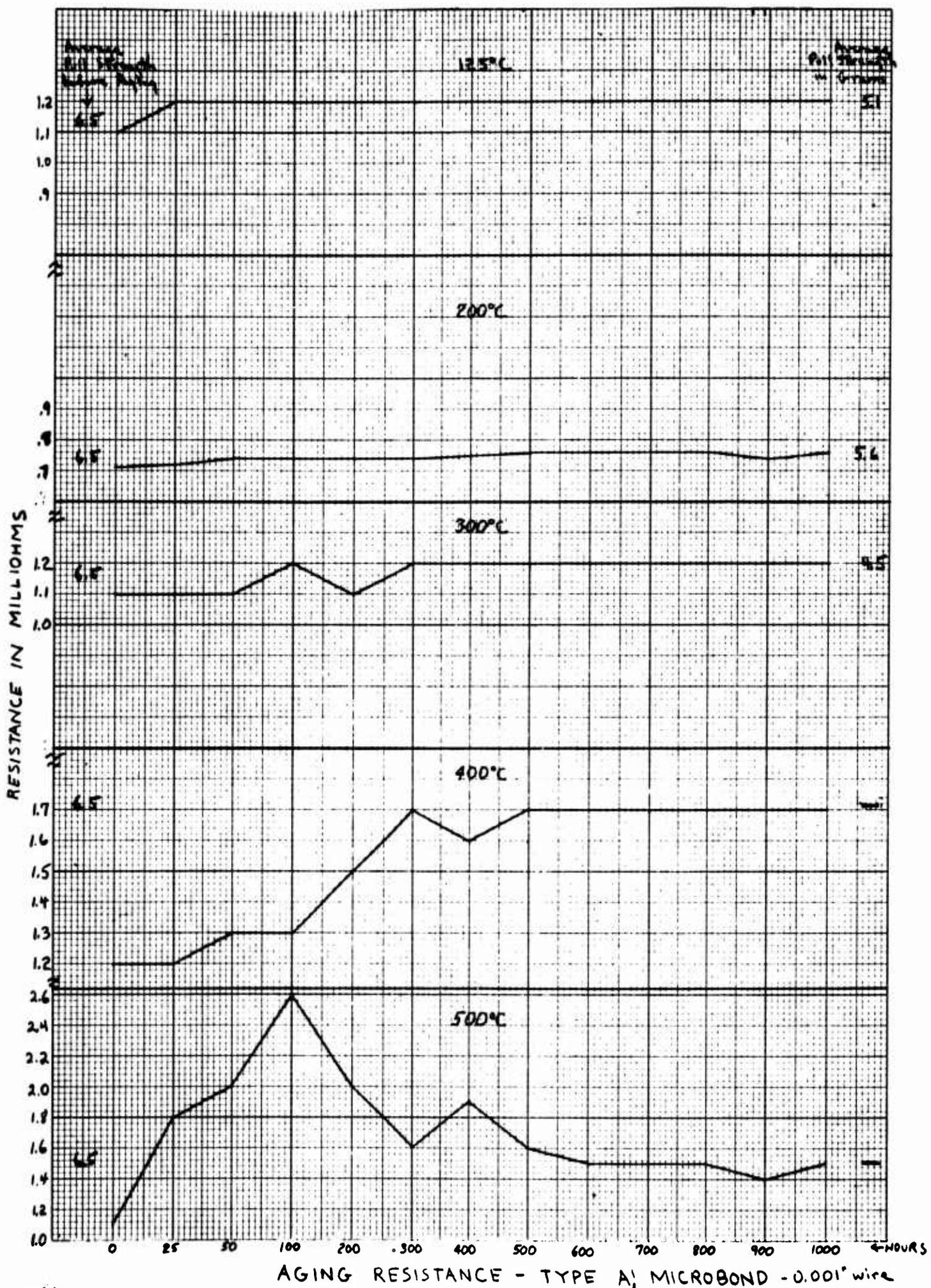
Figure 51 Resistance vs Thermal Aging Time Type A<sub>1</sub> Microbonds
