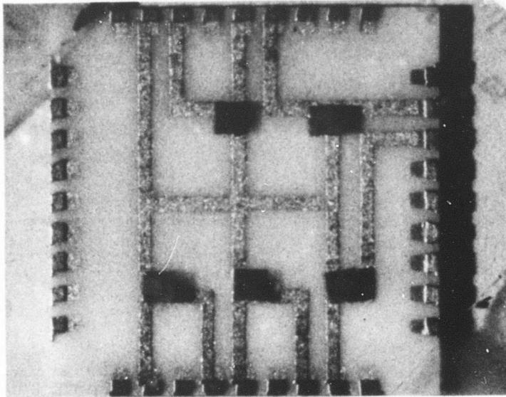
Figure 65 Ultrasonically Bonded Flip-Chip Transistors
