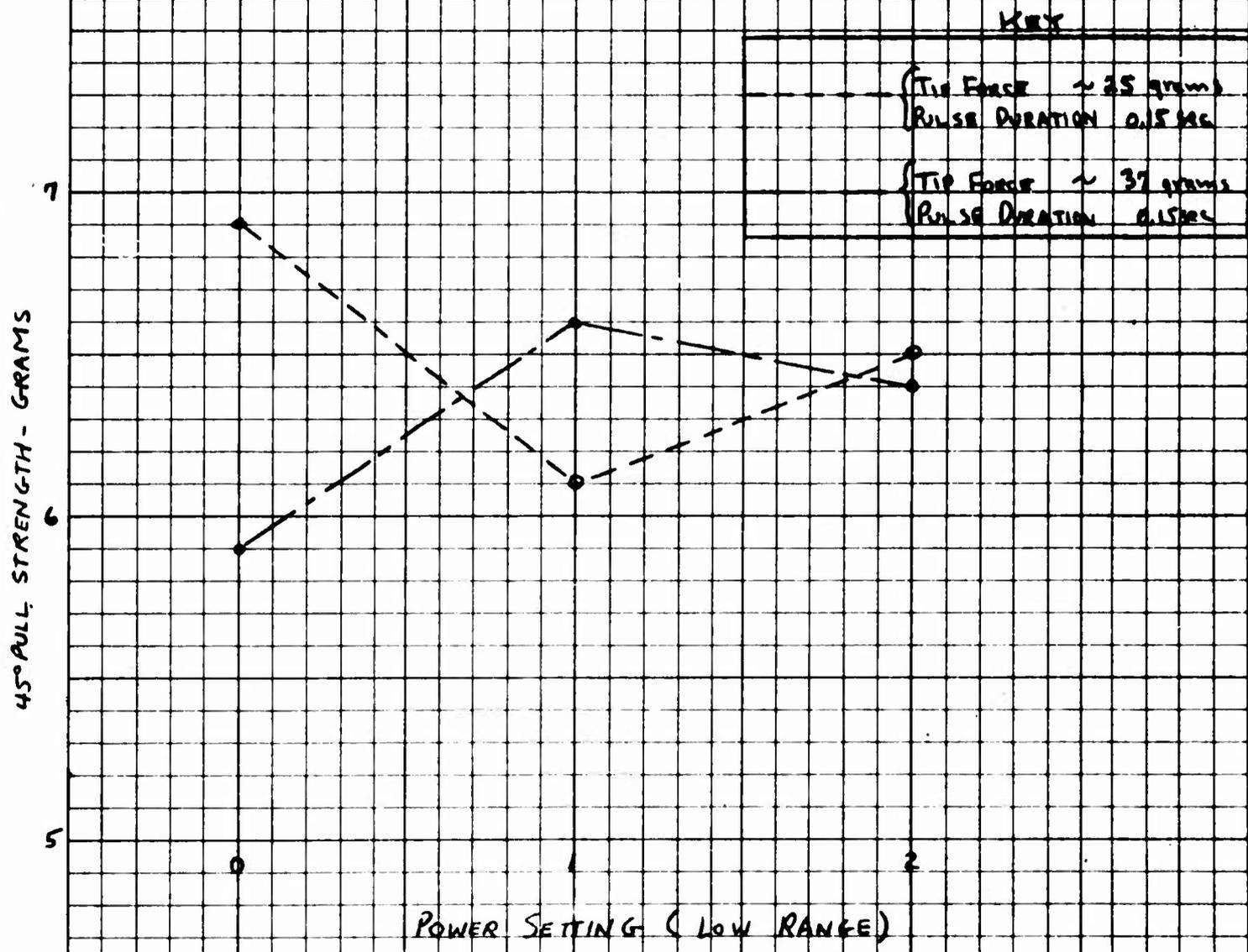
Figure 9 Weld Profile - Type K Microbonds
