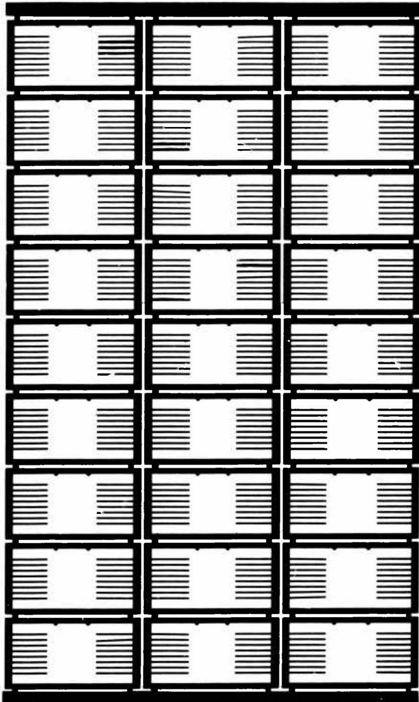
Figure 63 Nickel Lead Frames
