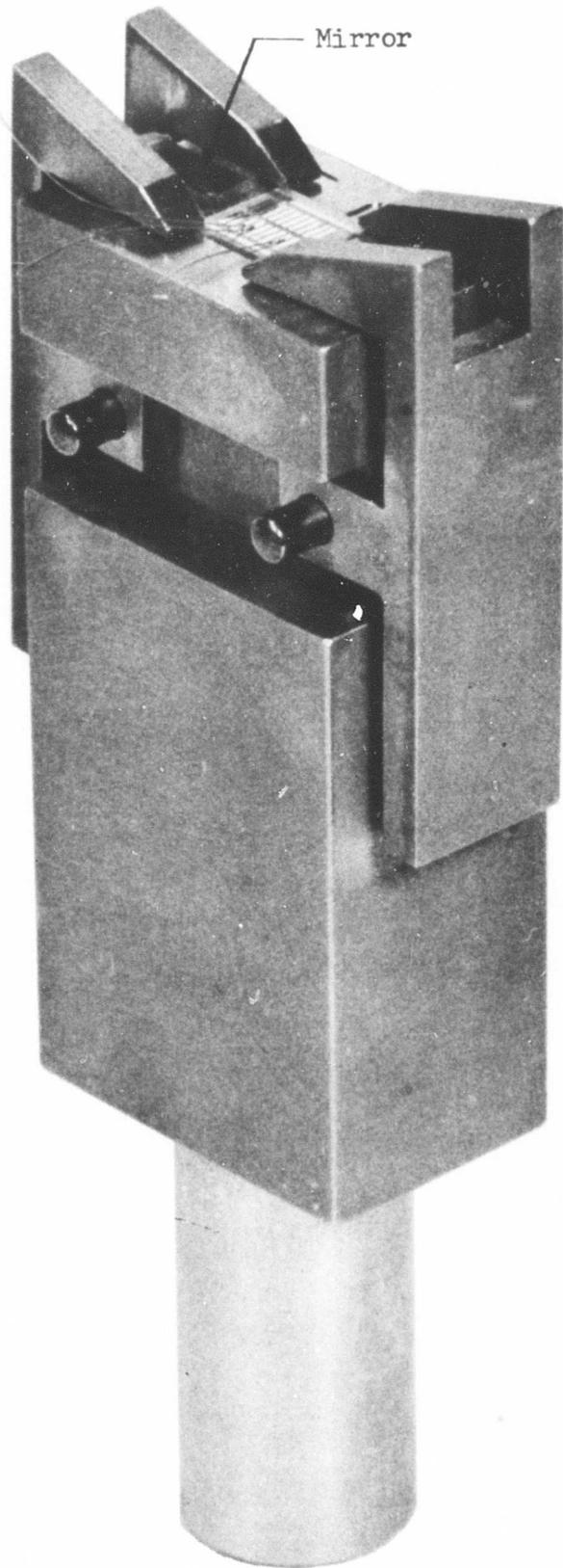
Figure 7 Modified Substrate Hold-down Fixture
