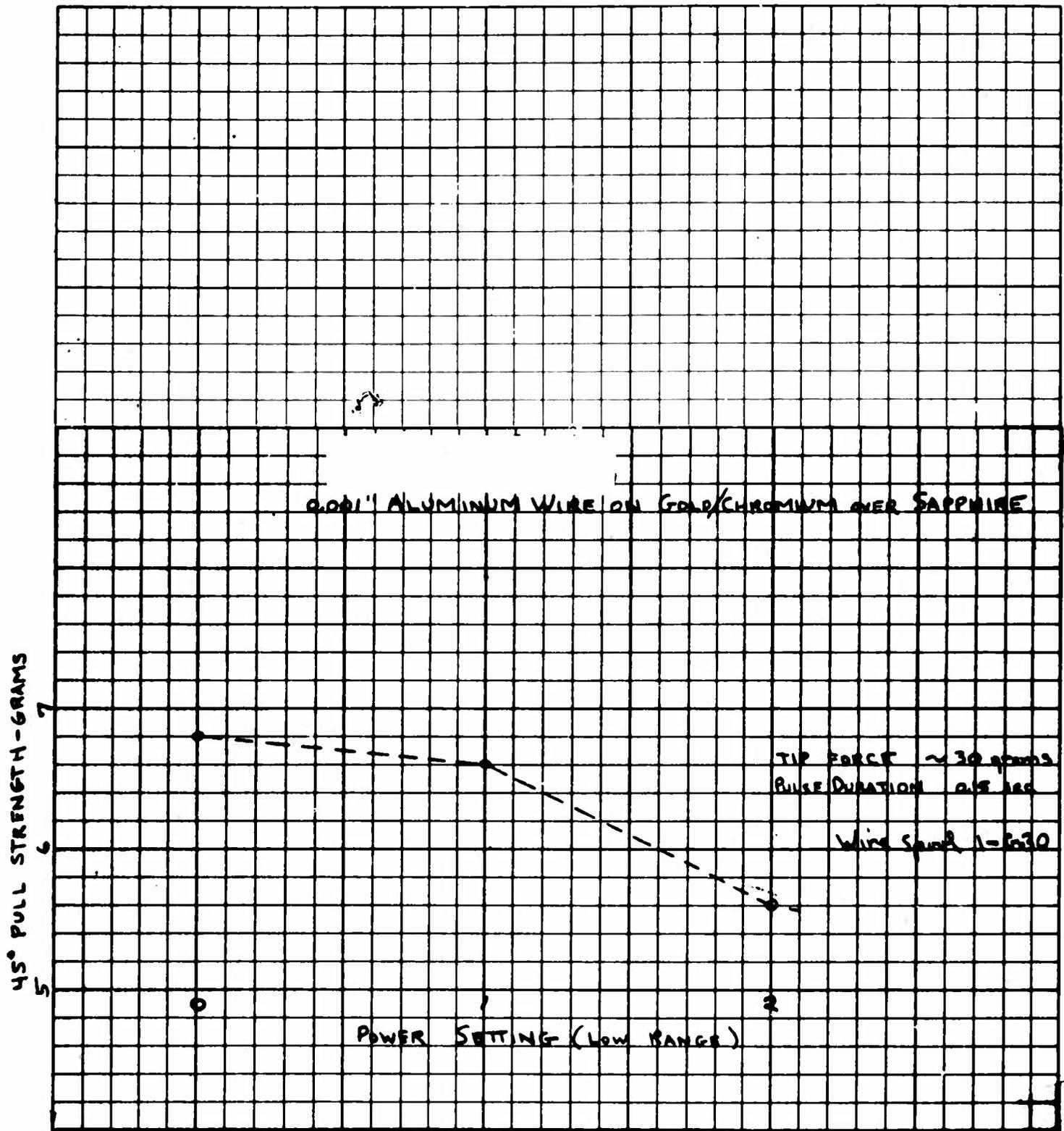
Figure 22 Weld Profile - Type B<sub>1</sub> Microbonds
