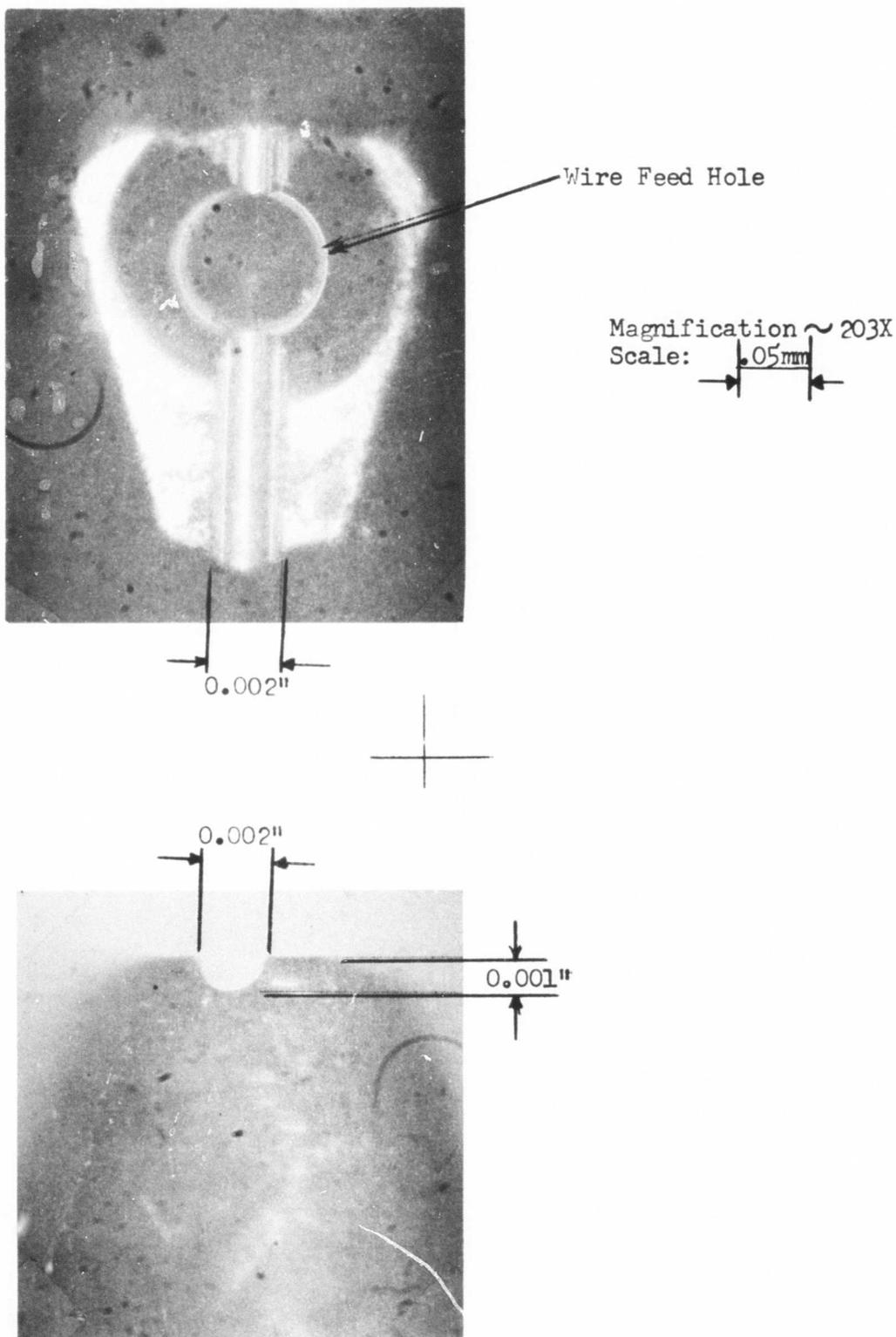
Figure 18 Photomicrograph of Bonding Tip for 0.002 inch Diameter Wire
