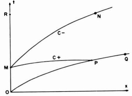
have a simple analytic solution, as long as the gas velocity remains below the local sound speed at the base of the barrel (segment OM in the diagram). At point M, the gas velocity equals the local sound speed; it is prescribed that thereafter they remain equal (but not constant) at the base of the barrel (segment MR). The initial analytic solution is regarded as holding throughout the region QOMN bounded by the projectile path and by the C<sup>-</sup>characteristic MN through M.
