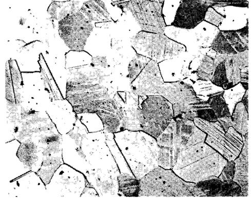
Figure 5. The as-cast structure of cerium metal.
