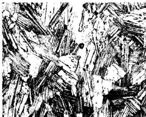
Figure 18. A 50 a/o Nd-50 a/o Gd alloy. Homogenized. Structure all samarium-type phase. 250X
