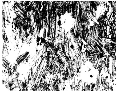
Figure 31. A 50 a/o Nd-50 a/o Gd alloy. Homogenized, cold worked, annealed at 800°C. 250X
