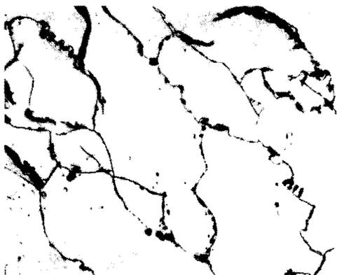
Figure 22. The homogenized structure of a 70 a/o Nd-30 a/o Gd alloy. Gadolinium solid solution present. 250X
