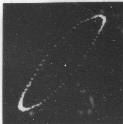
c.) INPUT VERSUS OUTPUT AT 50 CPS (SHOWING PHASE LAG).
