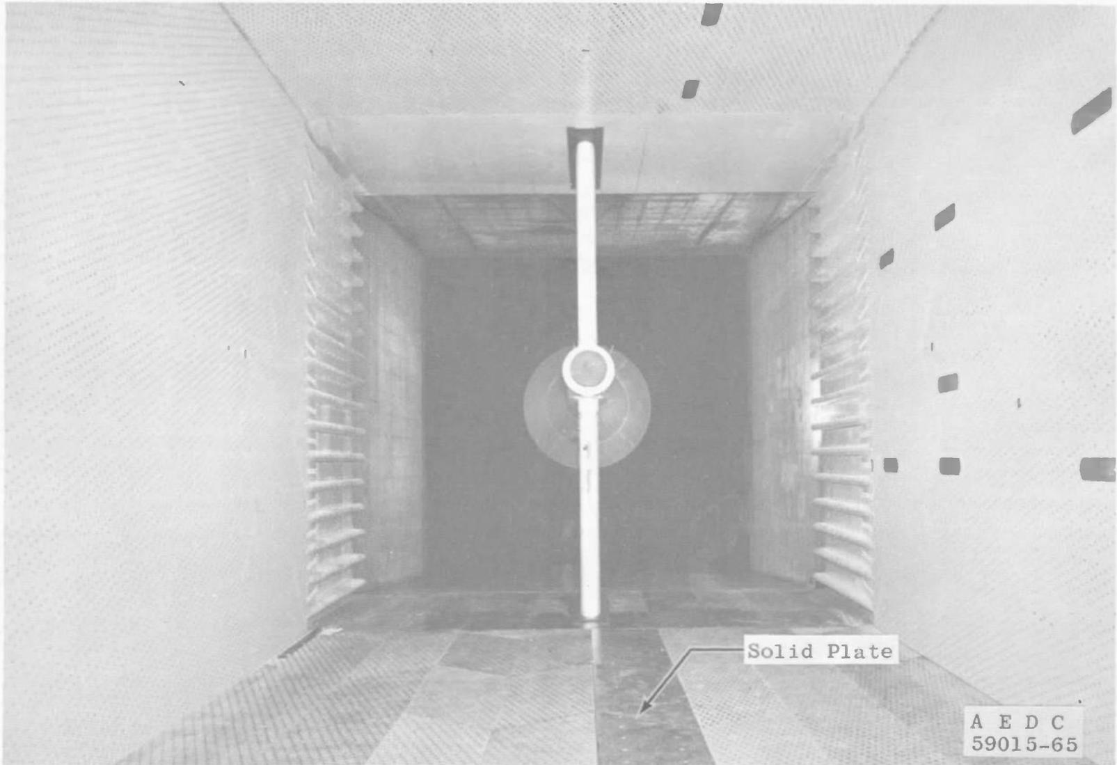
Fig. 4 Photograph of Empty Test Section Showing Solid Plates
