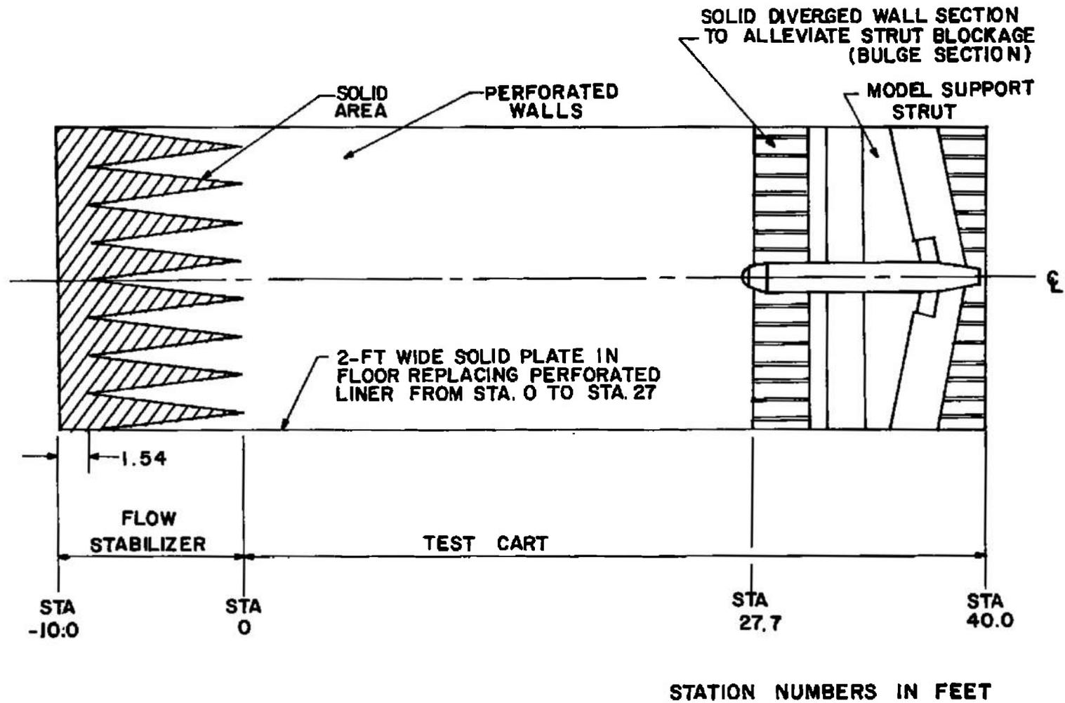
Fig. 2 16-ft Transonic Tunnel Test Section
