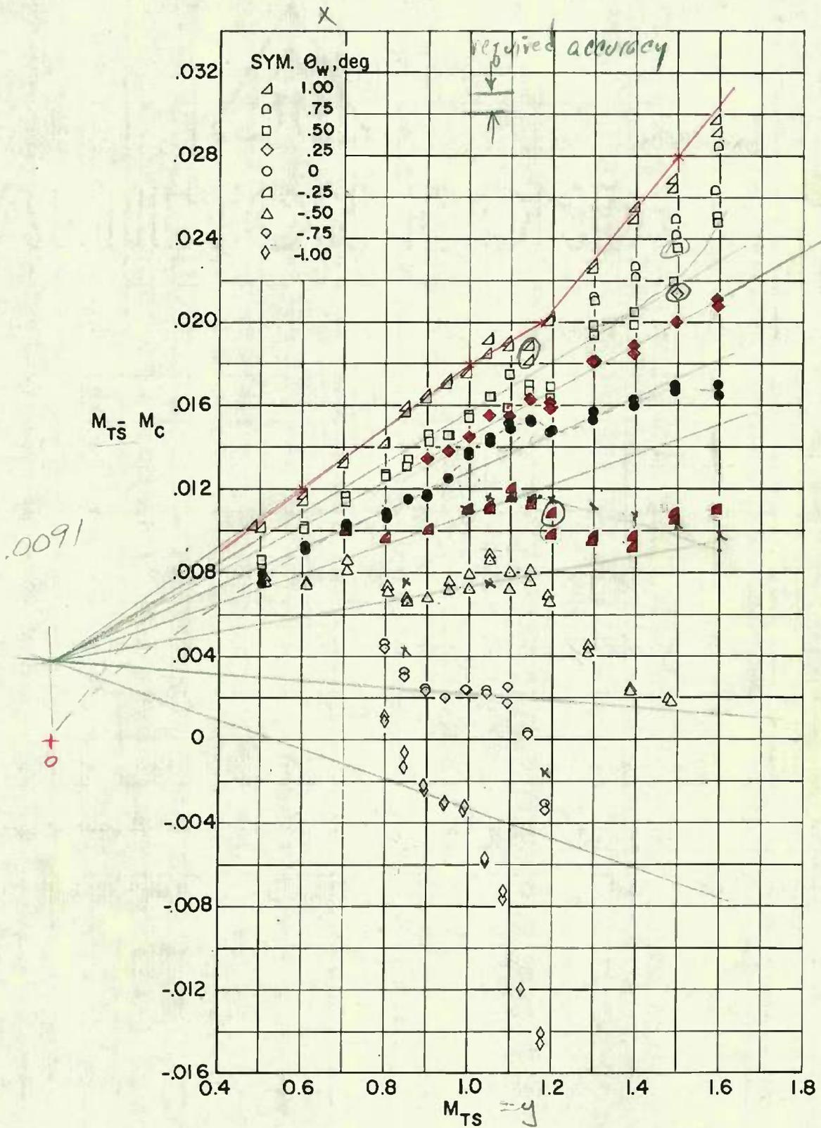
Fig. 7 Tunnel Calibration Based on Solid Plate Orifices
