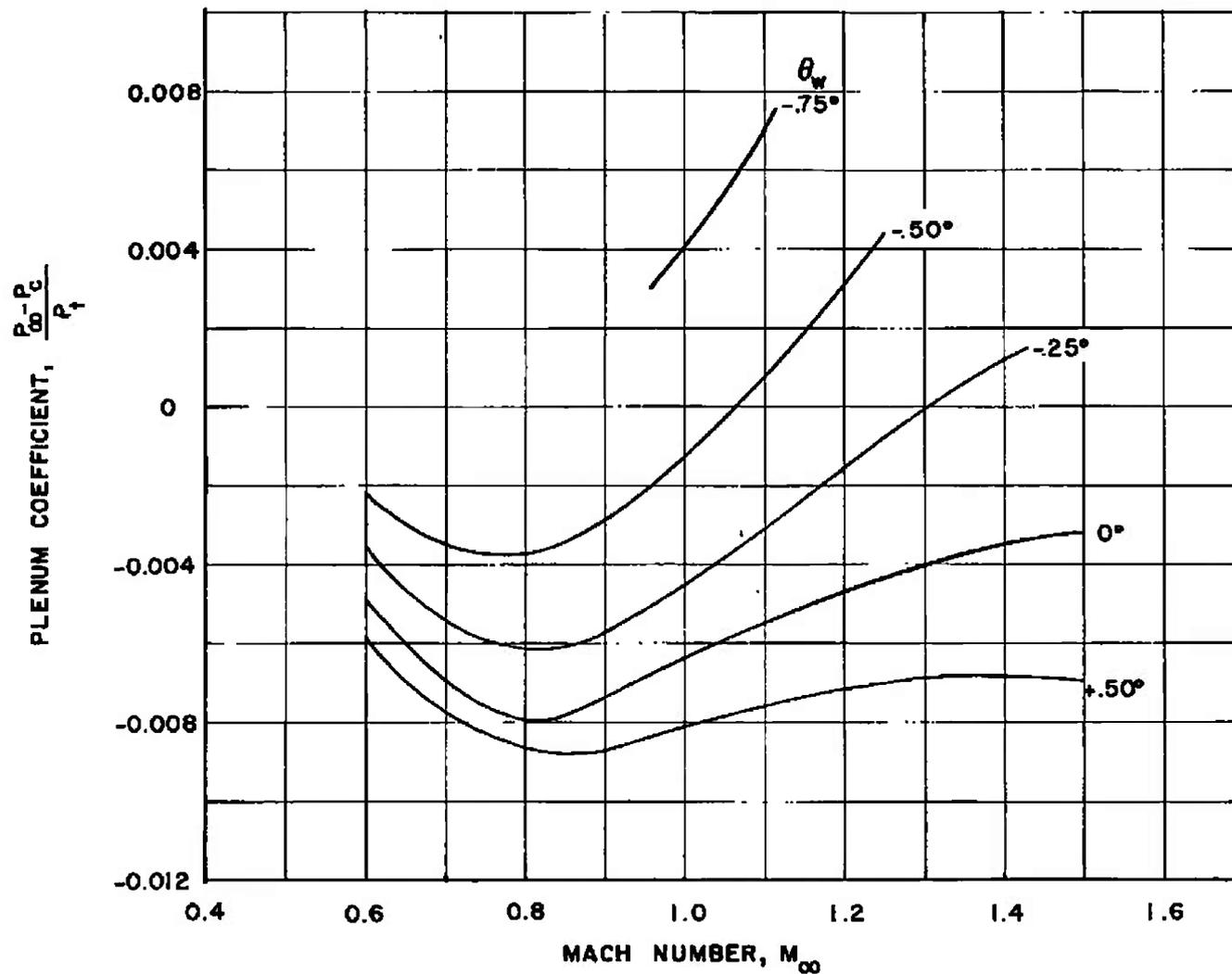
Fig. 9 Effect of Wall Angle on the Test Section Calibration - Data Obtained from Tunnel 1T Using Long Static Probe (From Ref. 4)
