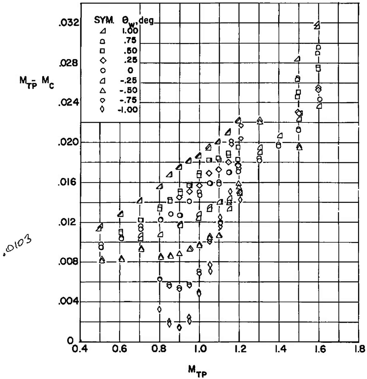
Fig. 8 Tunnel Calibration Based on Perforated Plate Orifices
