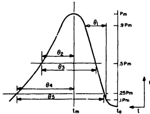
Fig. 11 - The form of an ideal oscillographic record, indicating the various time measurements
