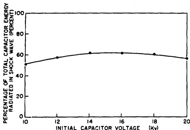
Fig. 10 — Ratio of shock-wave energy to initial capacitor energy versus initial capacitor voltage
