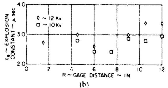
Fig. 12 - A plot of  $t_{max}$  versus gage distance (a) for 20, 18, 16, and 14 kv EWP explosions and (b) for 12 and 10 kv EWP explosions
