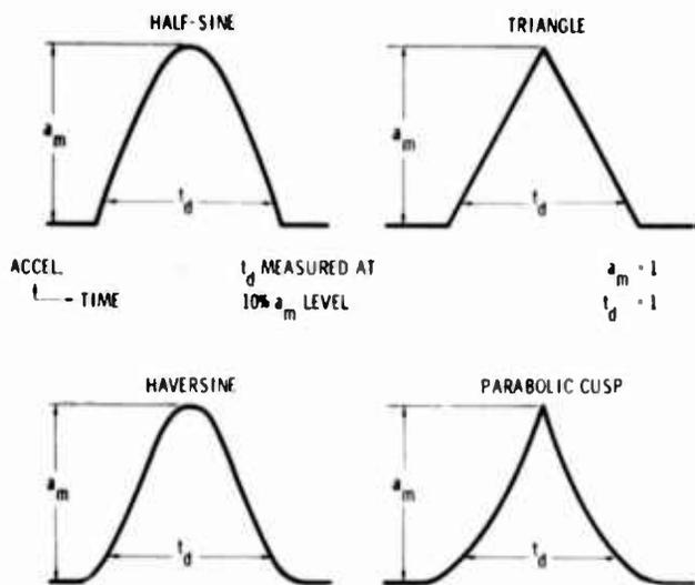
Fig. 1. Four normalized symmetrical pulse shapes
