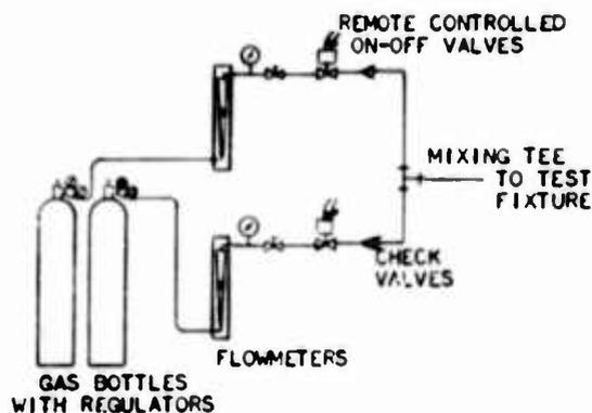
Fig. 5. Schematic diagram of gas metering equipment
