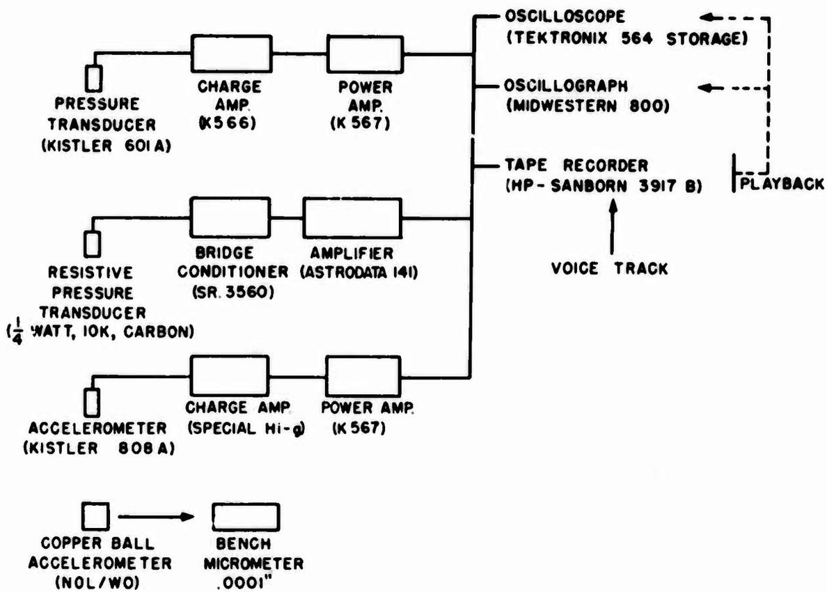
Fig. 16. Typical instrumentation block diagrams
