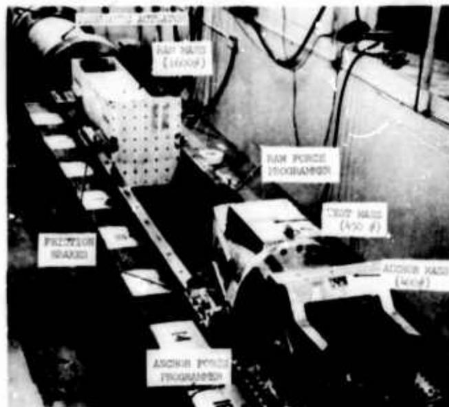
Fig. 3. Setup for shock test -- longitudinal axis
