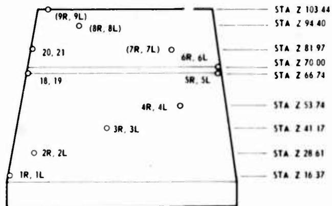
Fig. 5. Accelerometer locations on adapter skin -- test 2
