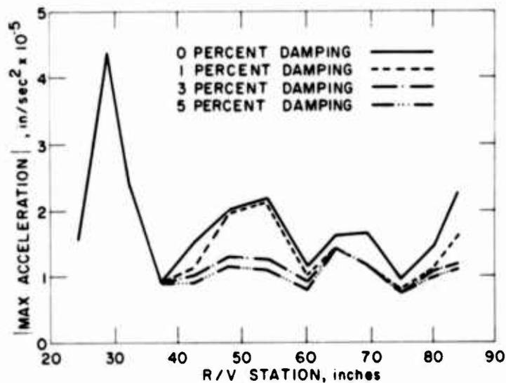
Fig. 28. Absolute max acceleration vs station lateral model
