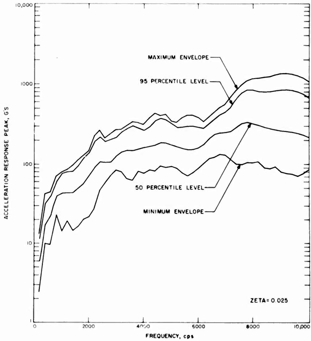
Fig. 12. Ranger Case IV response to mechanical separation
