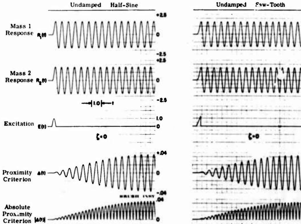
Fig. 2. Proximity criteria for half-sine and sawtooth pulses
