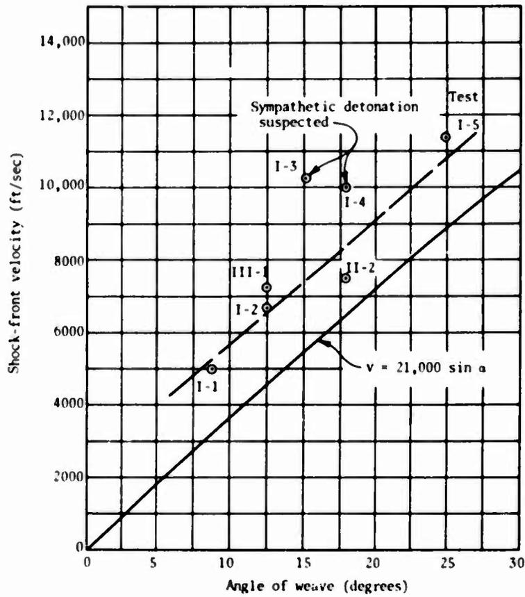
Fig. 14. Shock-front velocity vs angle of weave
