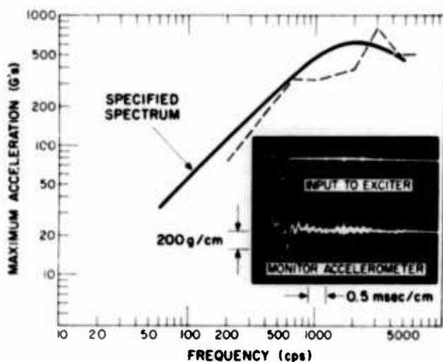
Fig. 3. Shock response spectrum for half-cycle sine input
