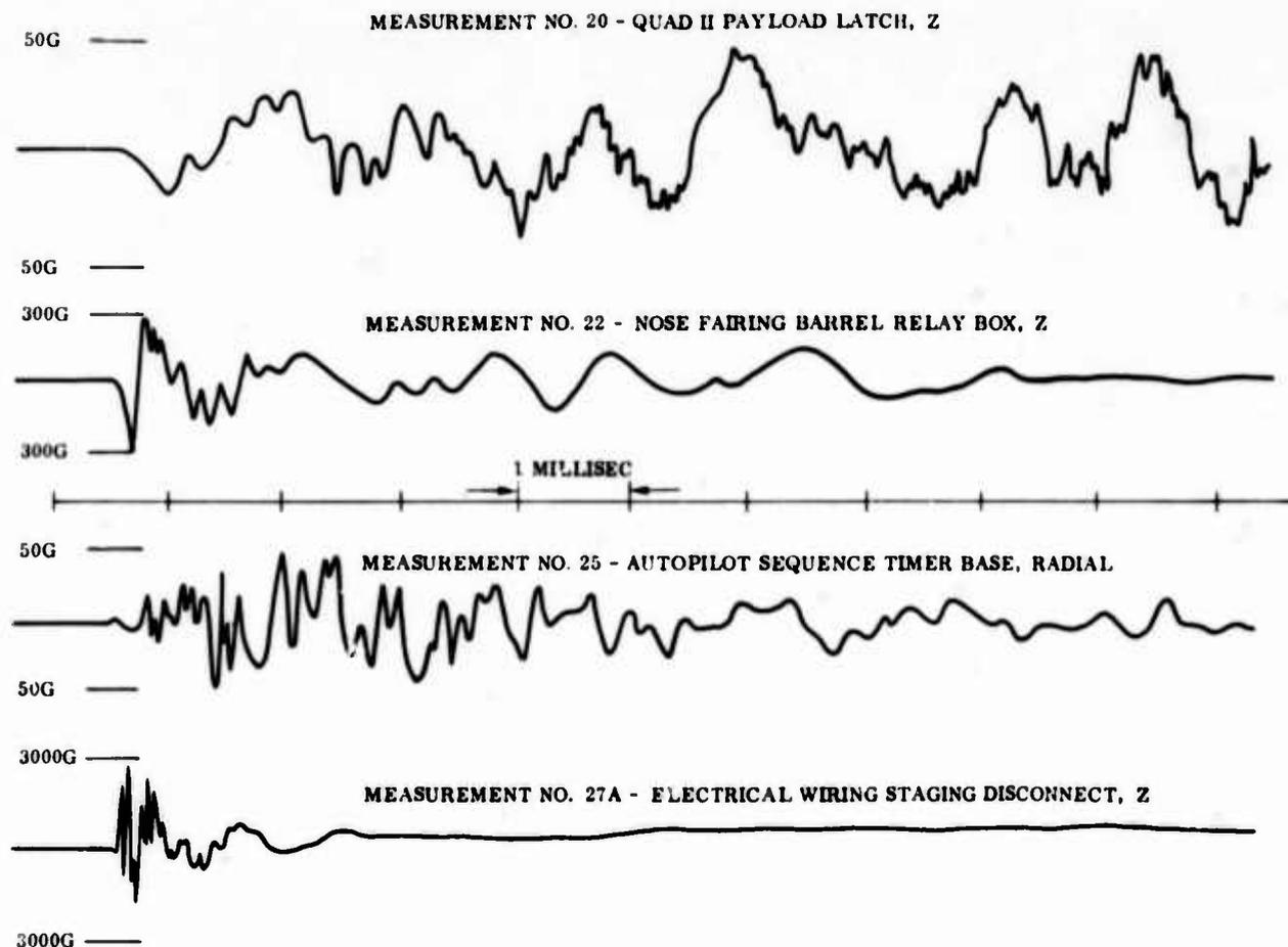
Fig. 10. Selected waveforms from insulation panel separation tests
