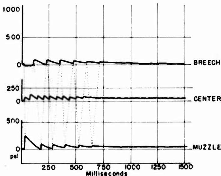
Fig. 24. Barrel air pressure vs time, without load
