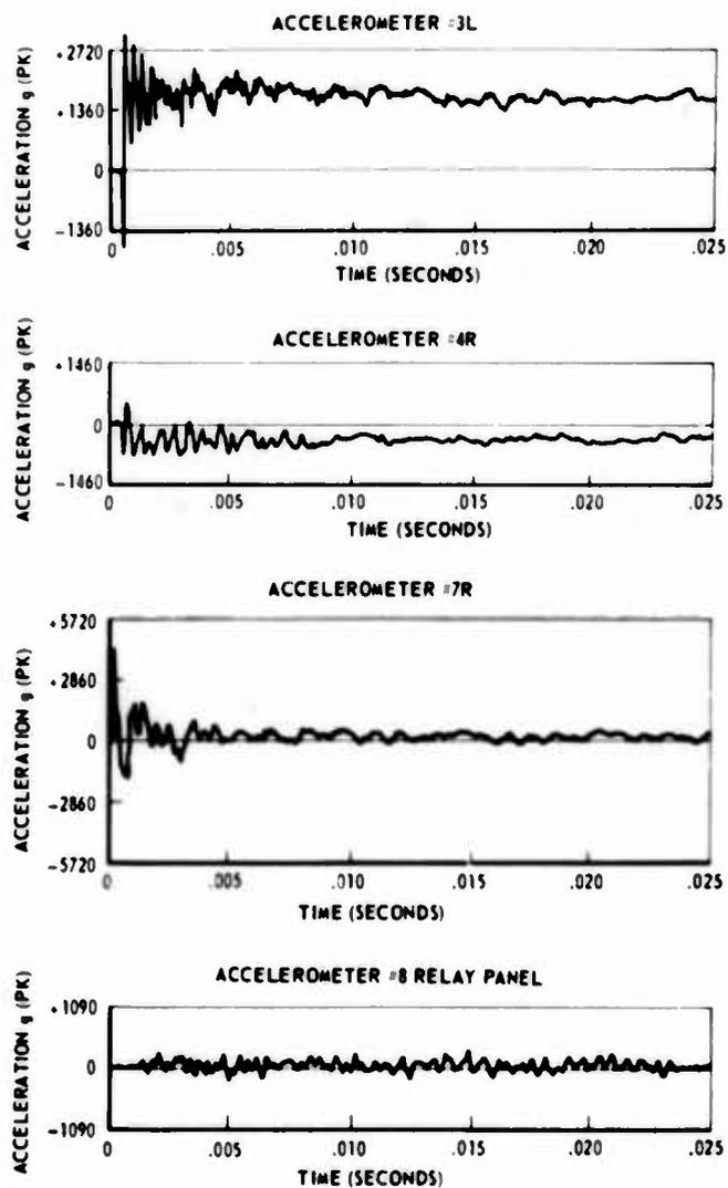
Fig. 6. Shaped charge firing at Z-13 -- test 1
