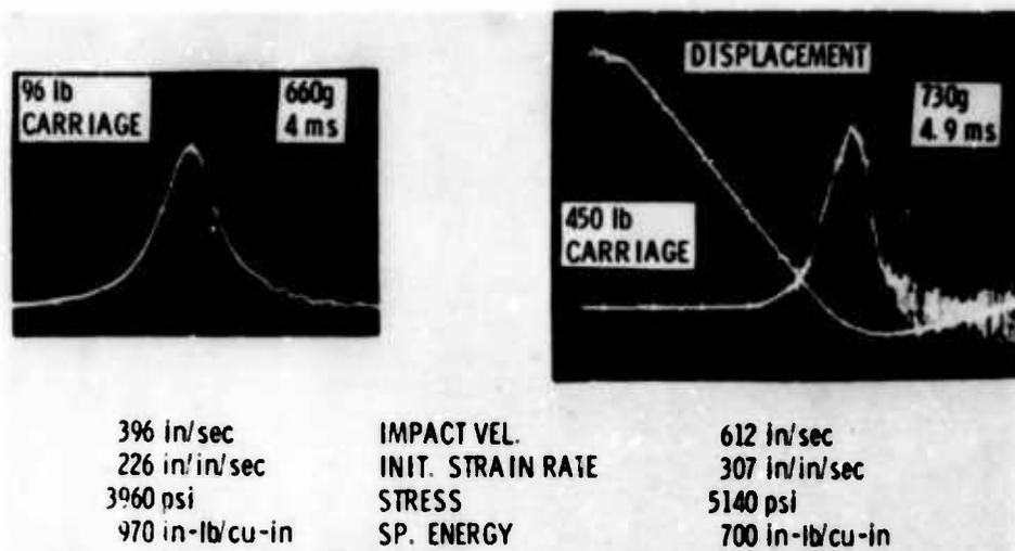
Fig. 4. Parabolic cusps from 30 Durometer A butyl rubber
