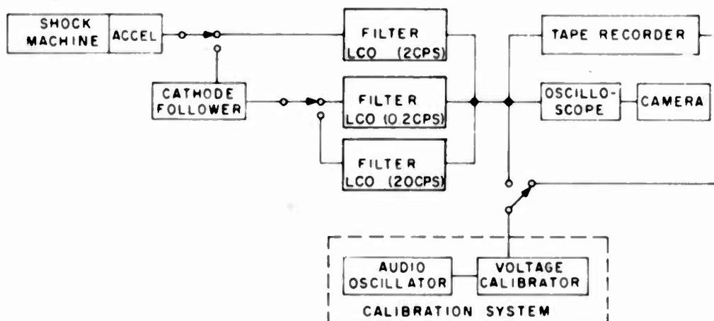
Fig. 1. Typical pulse recording system
