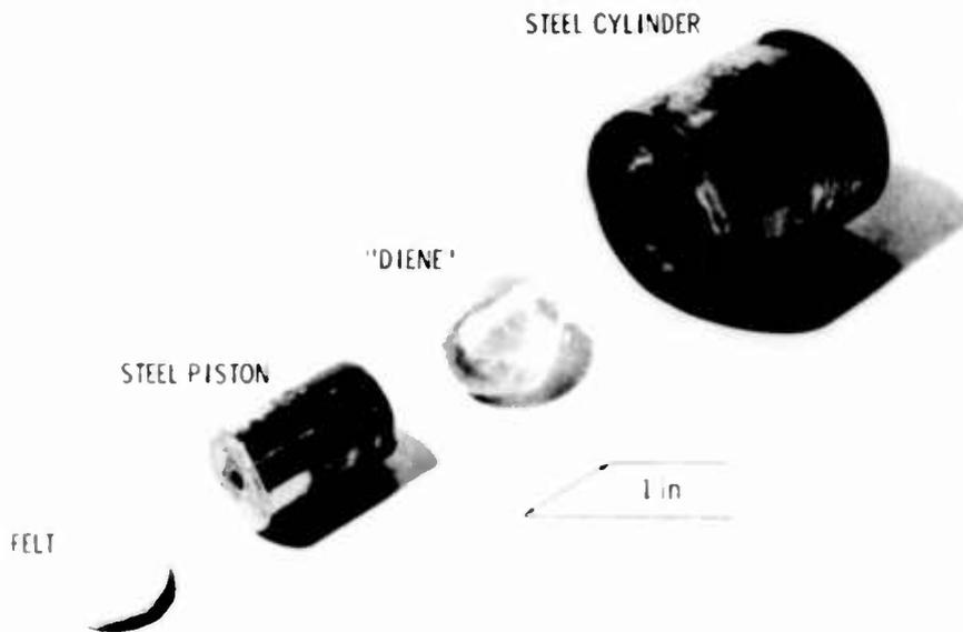
Fig. 19. Exploded view of contained Diene shock spring
