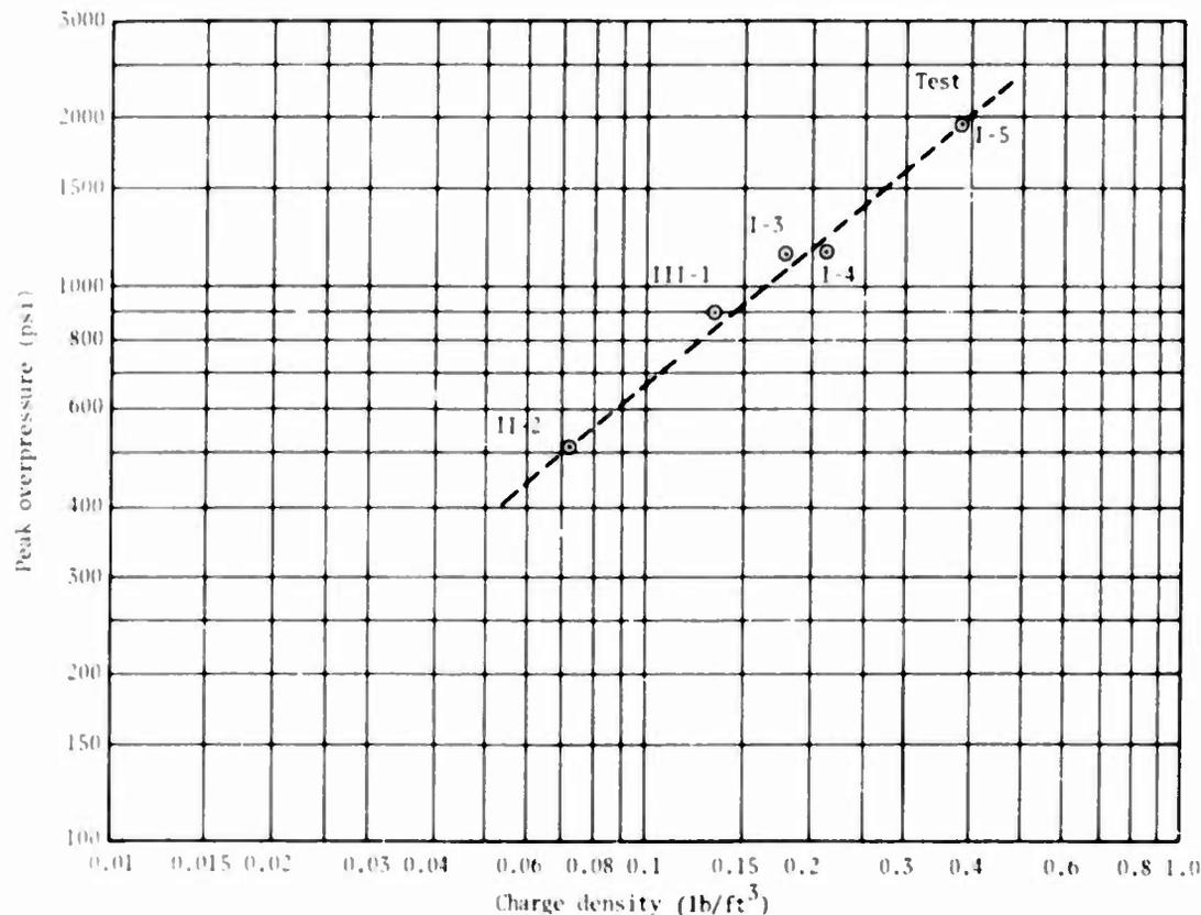
Fig. 12. Peak overpressure vs charge density
