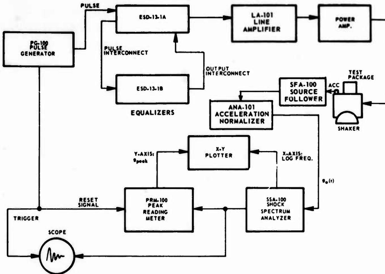
Fig. 1. Electrodynamic shaker shock synthesis and analysis system
