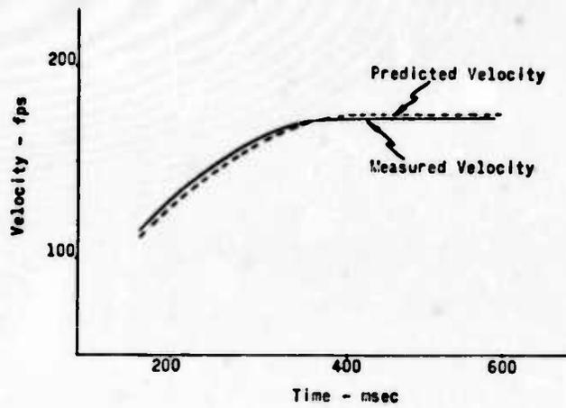
Fig. 6. Comparison of computed and measured carriage velocity
