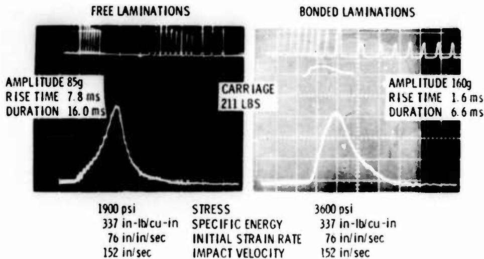
Fig. 6. Comparison of recorded pulses generated by free and bonded laminated rubber spring
