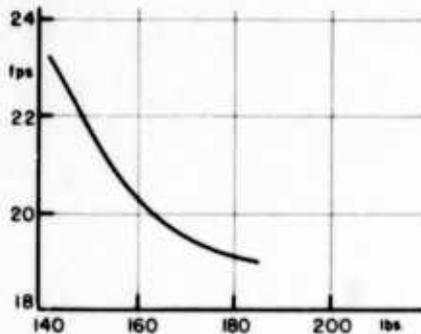
Fig. 27. Impact load velocity vs load weight, 0.25-in. platform spacing
