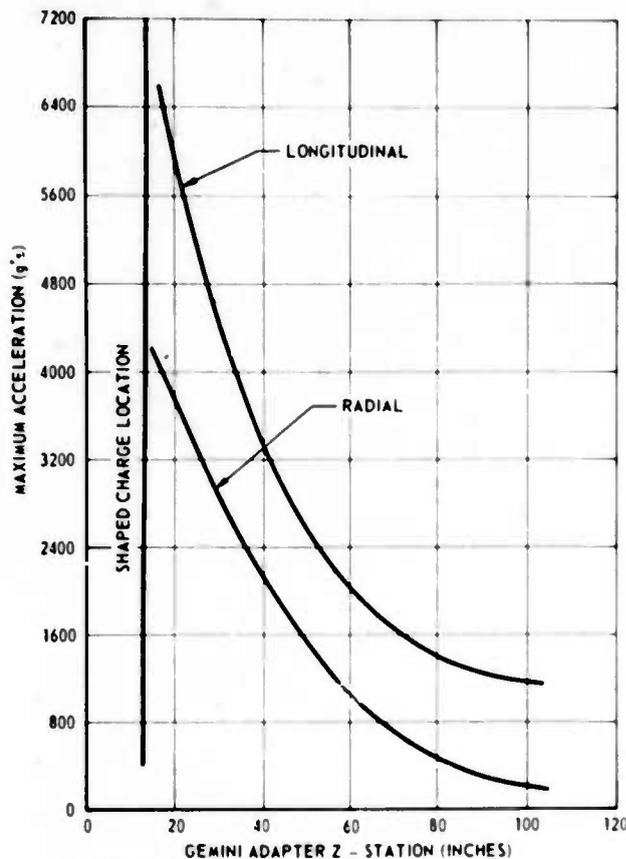
Fig. 12. Impulse attenuation -- Z-13 firing, 10 grains/ft
