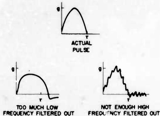
Fig. 1. Effect of filtering on shock pulses
