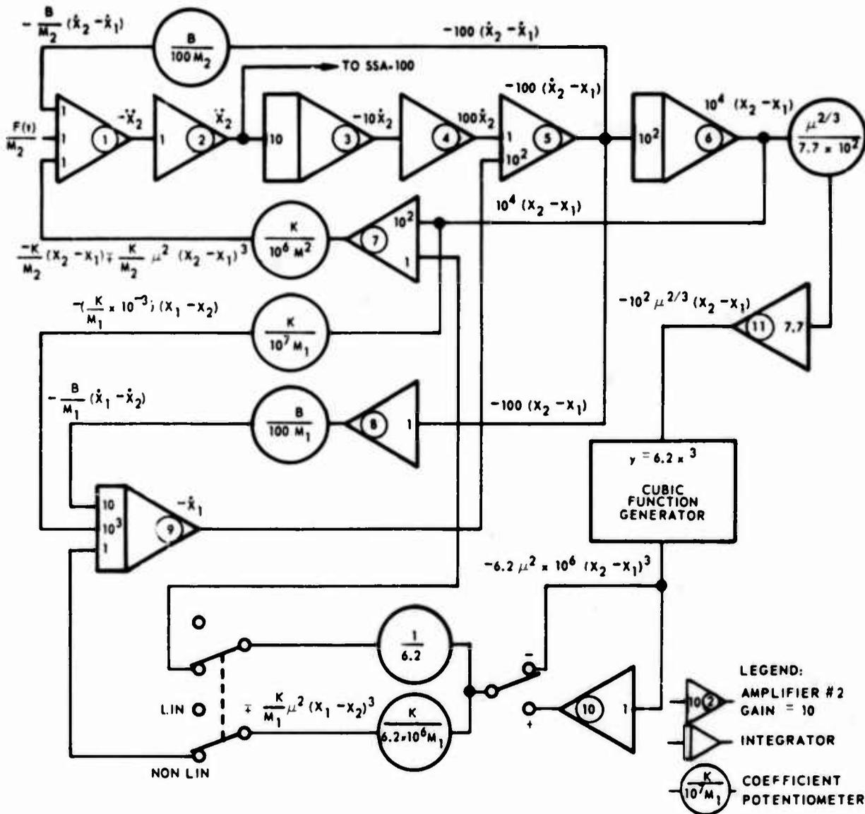
Fig. 4. Simulated load and armature dynamics
