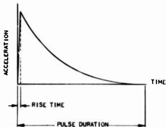
Fig. 1. Idealized blast wave rigid body acceleration-time history
