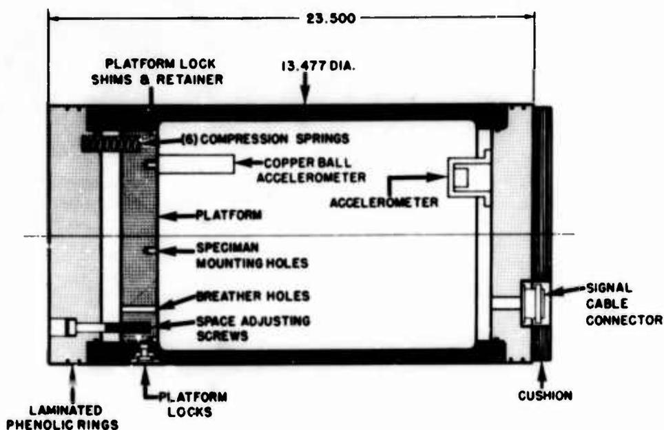
Fig. 21. Piston load (test item carriage) diagram
