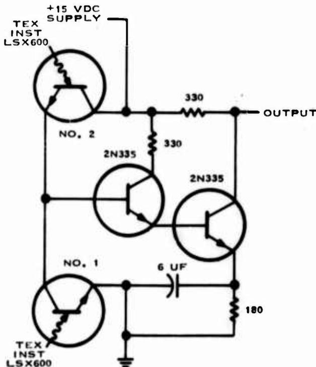
Fig. 6. Light sensor circuit, schematic diagram
