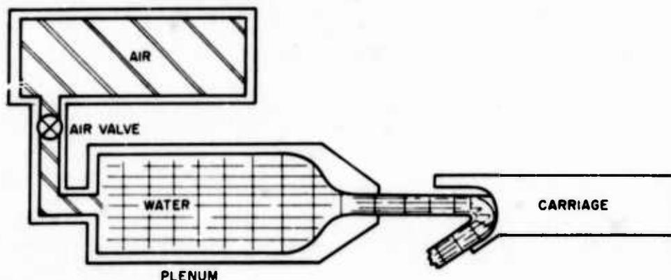
Fig. 1. Schematic of water jet catapult system
