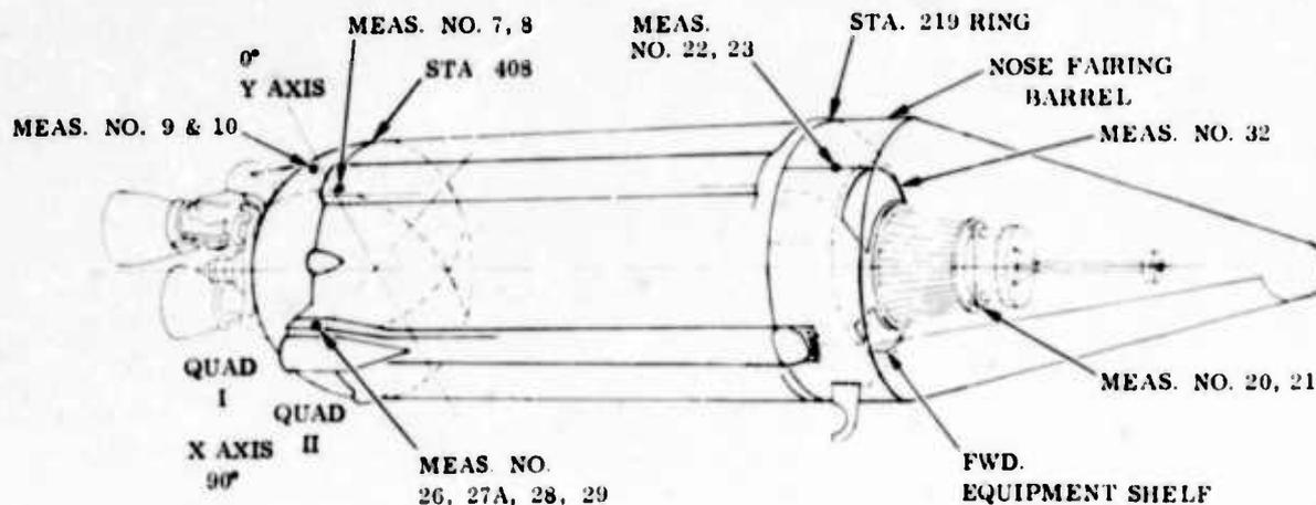
Fig. 4. Accelerometer locations for insulation panel jettison test
