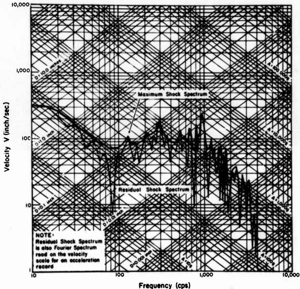
Fig. 9. Maximax and residual spectra for record 4
