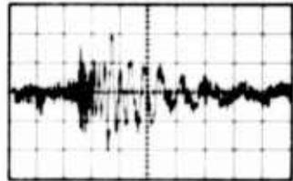
Fig. 11. Amplitude/time trace of shock, synthesized on electrodynamic shaker with and without 10 g rms random vibration
