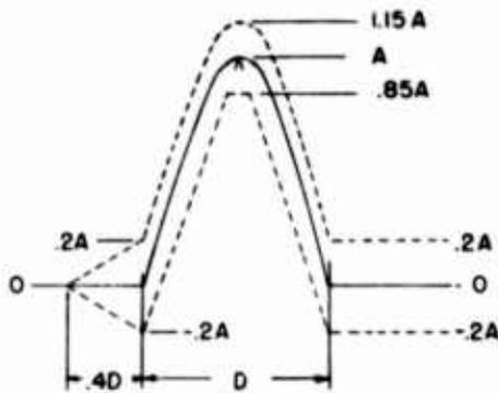
Fig. 3. Half-sine acceleration pulse with tolerance envelopes. Velocity change associated with pulse is  $\Delta V_i = 0.636DA$  ( $D$  expressed in seconds and  $A$  as acceleration).  $\Delta V_m$  (measured) must be equal to  $\Delta V_i \pm 10$  percent. Tolerances proposed by IEC/50A/WG1.
