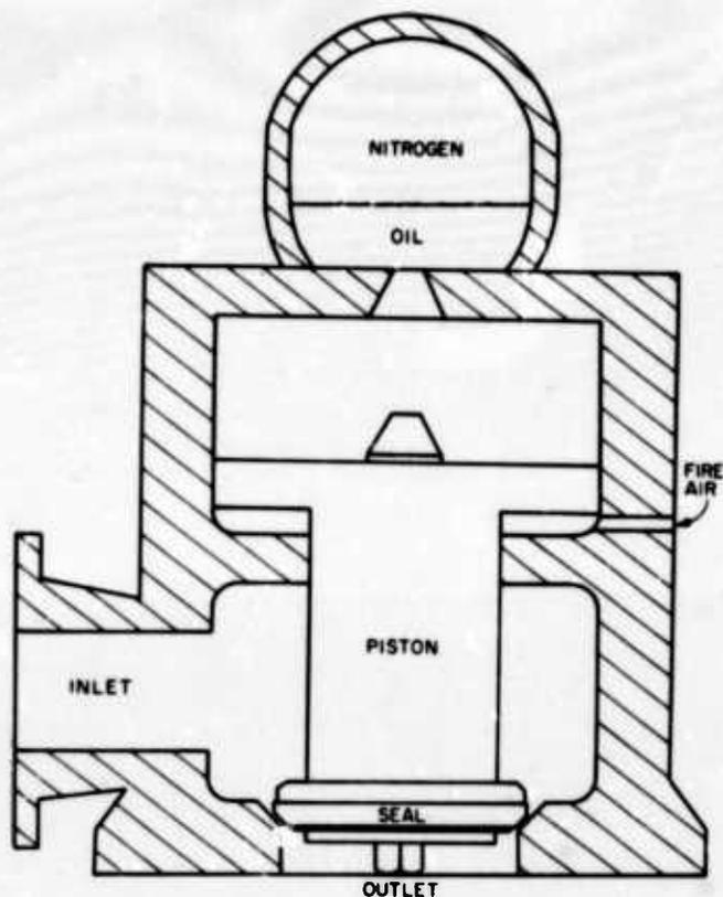
Fig. 2. Firing valve for water jet catapult
