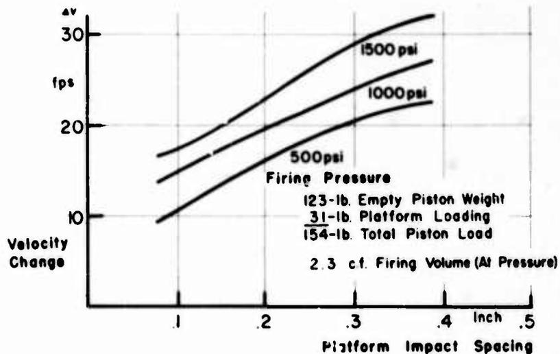
Fig. 26. Impact load velocity vs impact spacing
