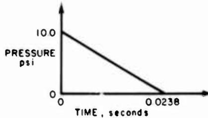
Fig. 15. Cylindrical shell and loading function
