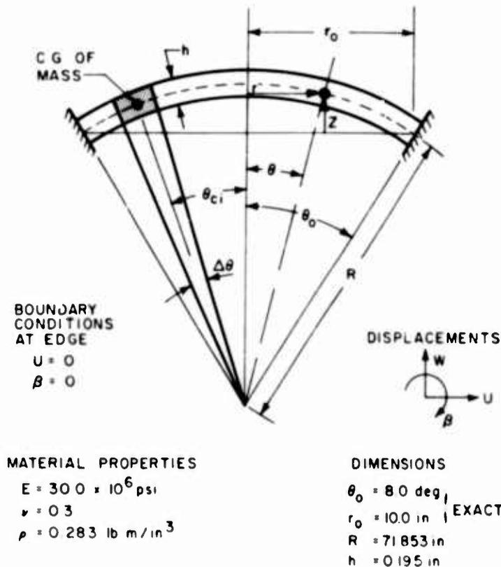
Fig. 9. Spherical cap model used for analytical study
