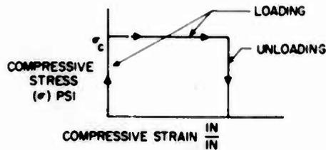
Fig. 8. Ideal plastic behavior of honeycomb as assumed during analysis
