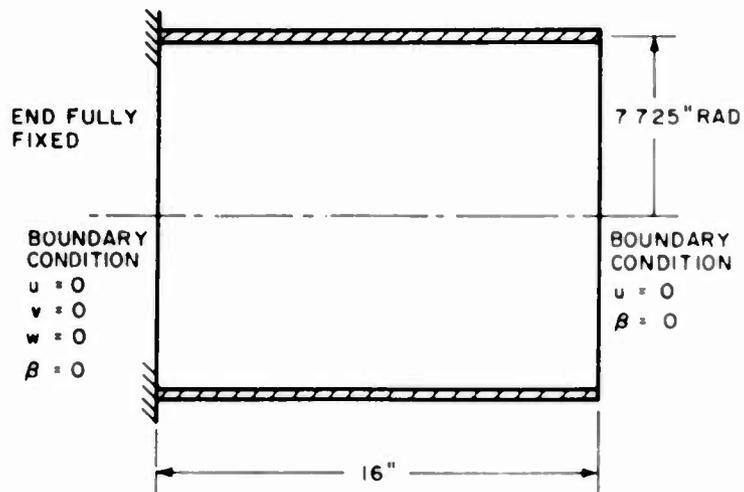
READING FROM THE FULLY FIXED END THE MODEL WAS COMPOSED OF THE FOLLOWING ELEMENTS
