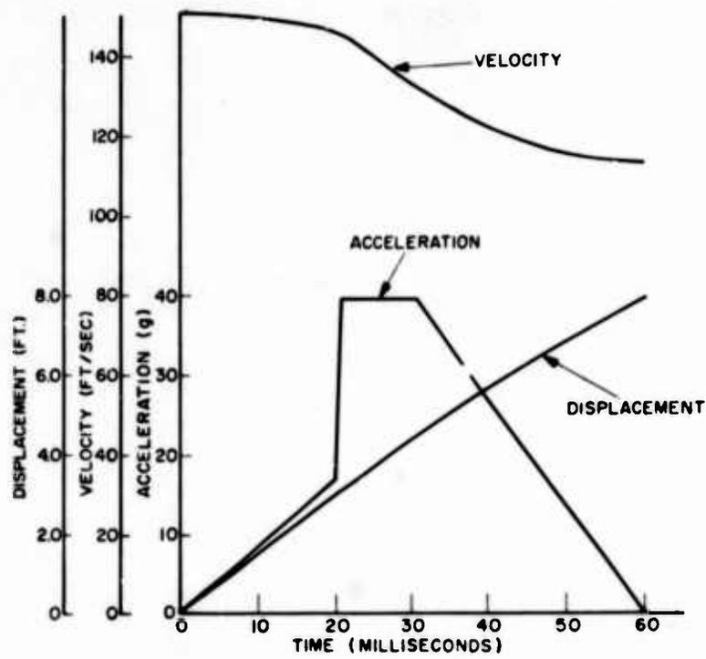
Fig. 8. Moving sled acceleration, velocity, and displacement curves
