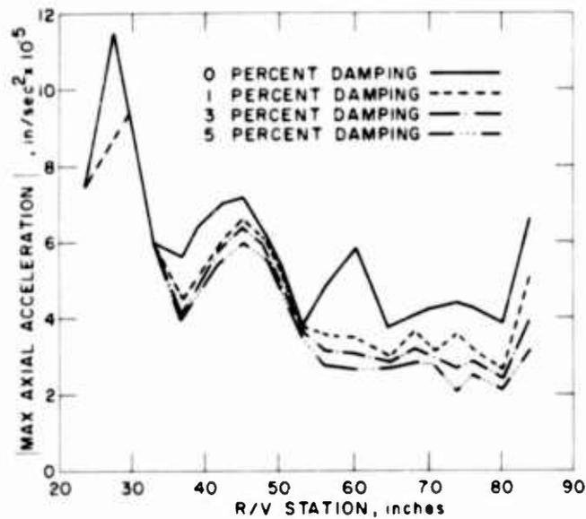
Fig. 27. Absolute max acceleration vs station axial model
