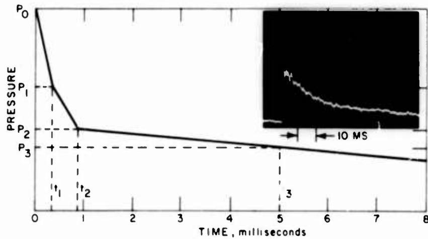
Fig. 13. Idealized pressure pulse applied to cylinder end
