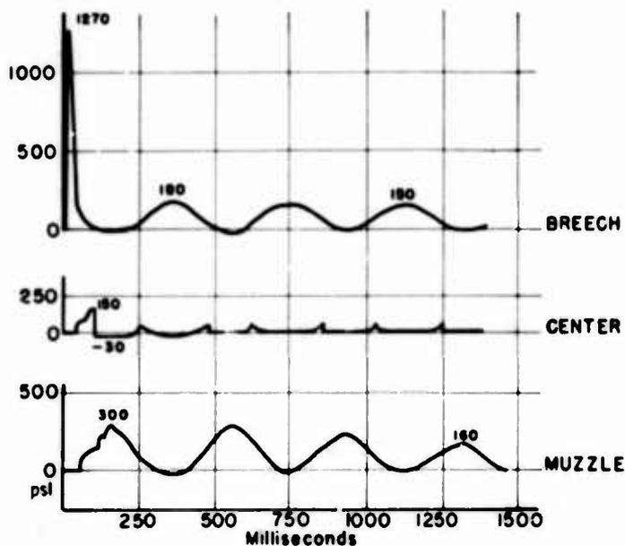
Fig. 28. Barrel air pressure vs time, 154-lb load
