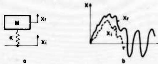
Fig. 2. Response of single degree of freedom system
