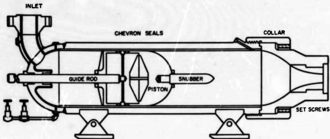
Fig. 4. Plenum assembly for water jet catapult
