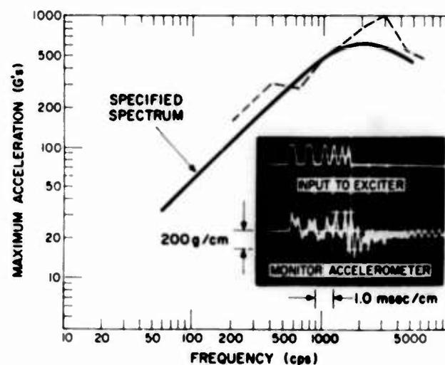
Fig. 4. Shock response spectrum for compound pulse input
