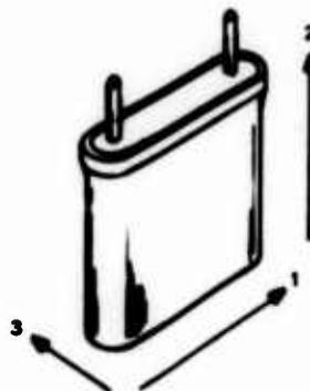
Fig. 13. CR-23/U crystal, axes of applied shock
