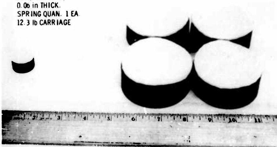
Fig. 13. Two laminated phenolic spring setups
