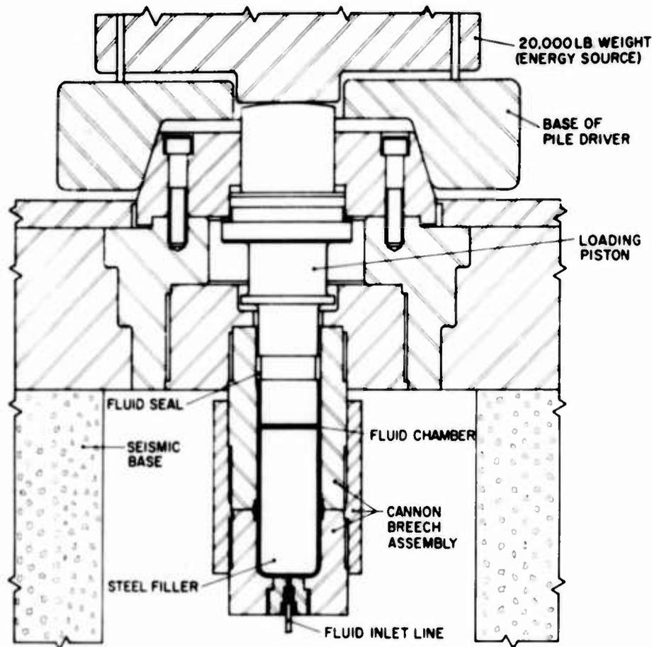
Fig. 1. Sectional view of impact test facility
