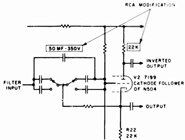
Fig. 5. Schematic diagram of modification to N504 amplifier
