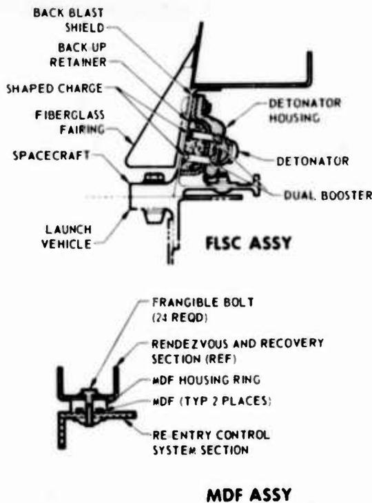
Fig. 3. Pyrotechnic assemblies
