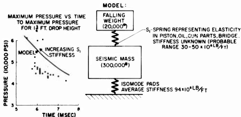
Fig. 13. Comparison of experiment with simplified analytical model
