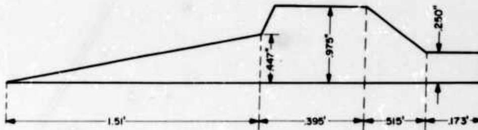
Fig. 16. Cross section of shear metal configuration
