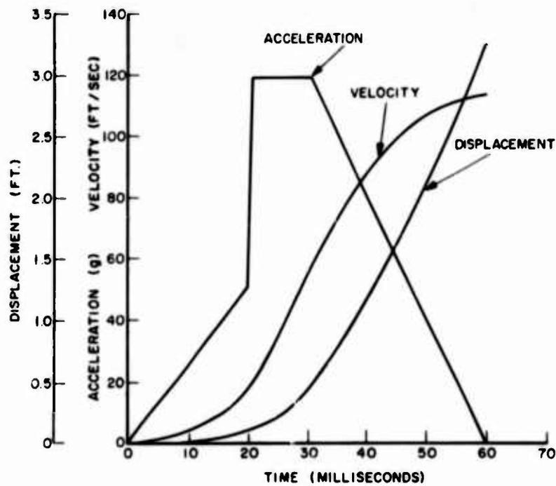
Fig. 9. Stationary sled acceleration, velocity, and displacement curves
