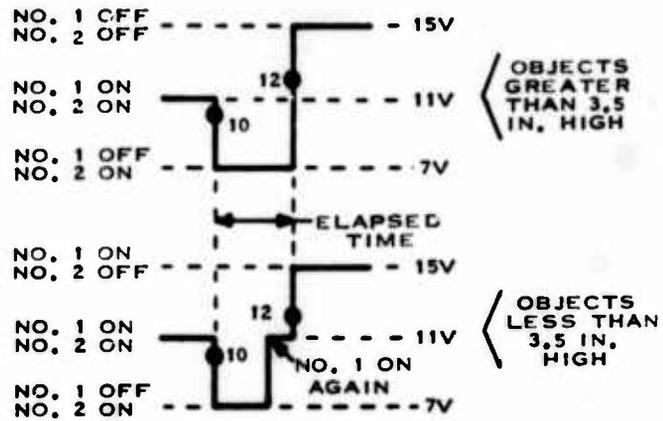
Fig. 7. Theoretical light sensor circuit output pulse
