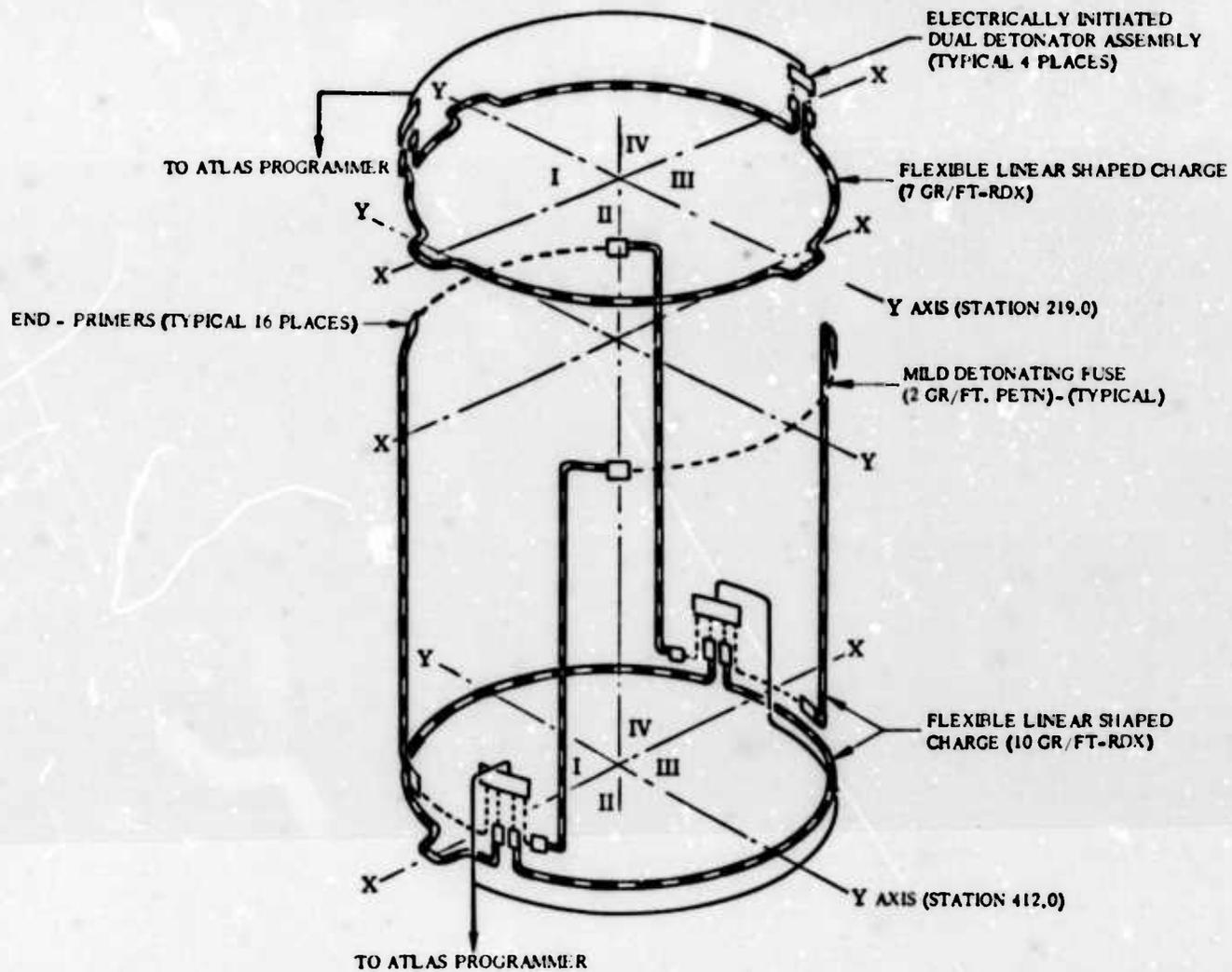
Fig. 2. Insulation panel shaped charge separation system
