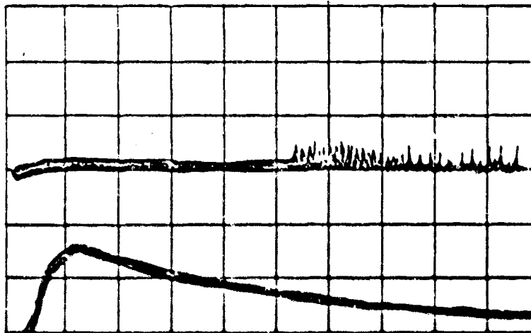
Figure 4 Intensity of radiation from ruby versus time. Light emitted from ruby: upper trace. Light emitted from flashlamp: lower trace. Horizontal scale = 1 cm = 0.1 milliseconds
